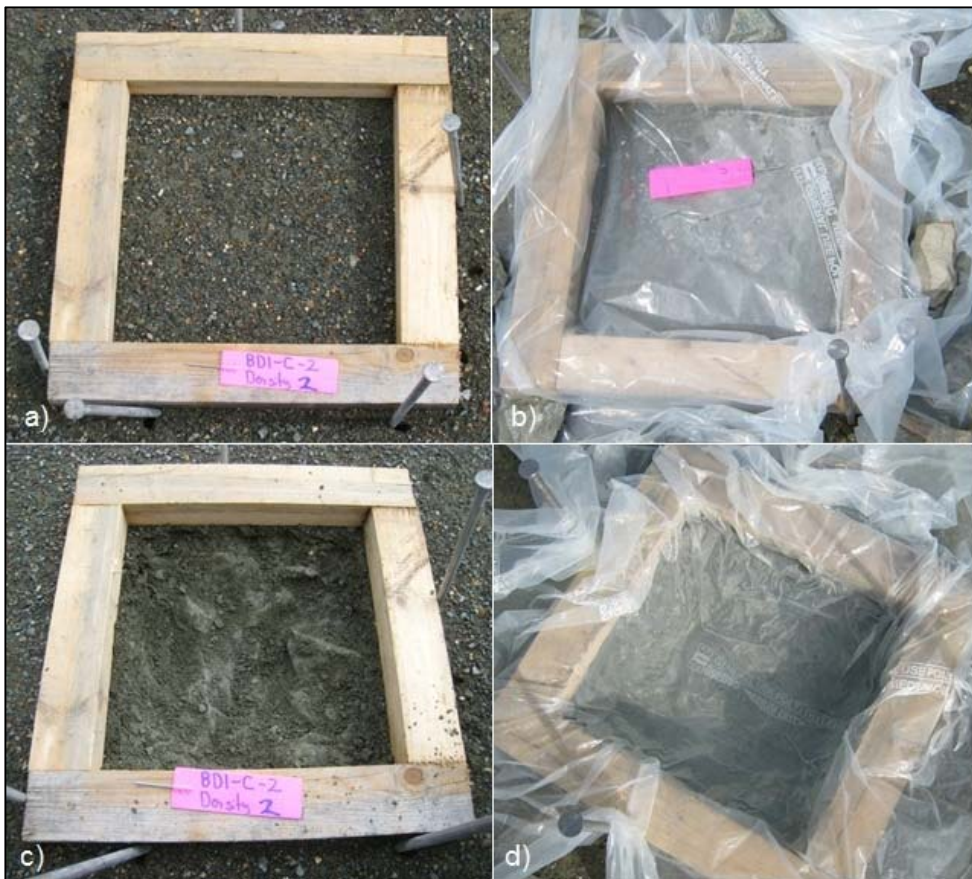
Figure 3-9: Water replacement density test - a) secured frame, b) initial surface volume, c) excavation, d) test pit volume
