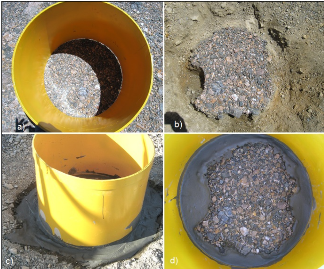
Figure 3-8: Single-ring infiltration test in coarse waste rock - a) intended test surface, b) final test surface excavation, c) grouted in place, d) inner grout seal
