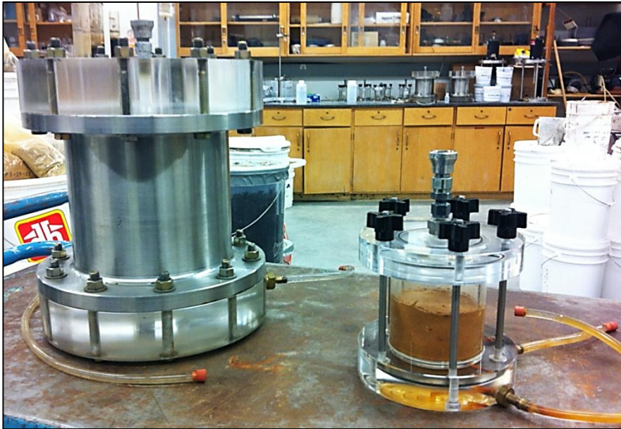
Figure 3-19: Large (left) and small (right) Tempe cells used for soil-water characteristic curve testing
