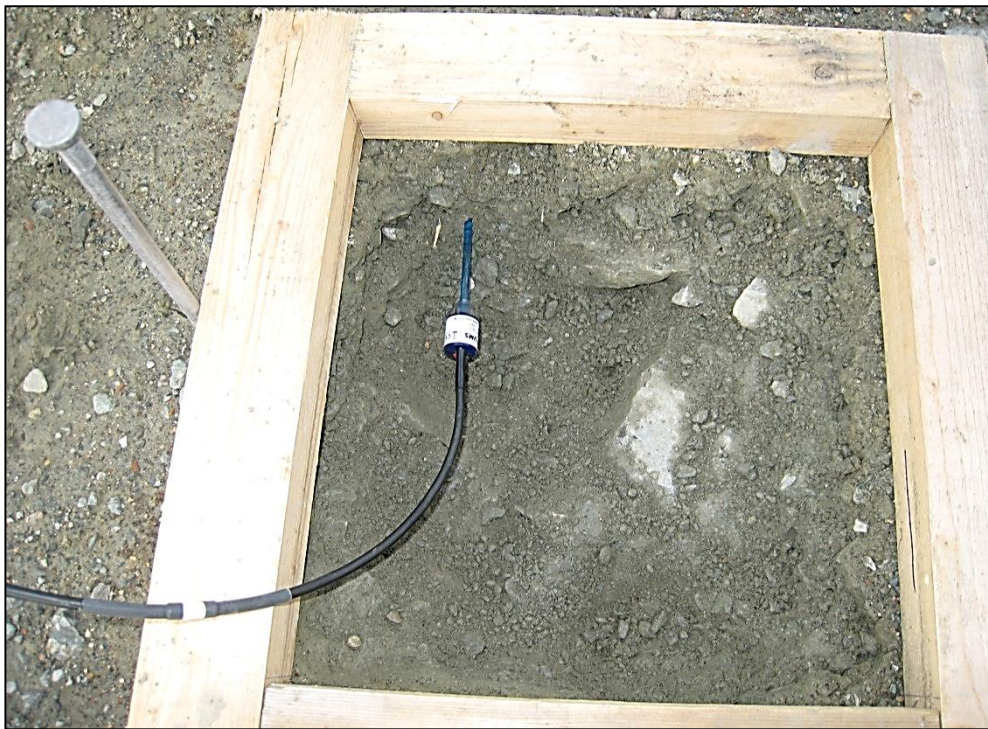
Figure 3-10: Soil suction measurement using pressure transducer tensiometer
