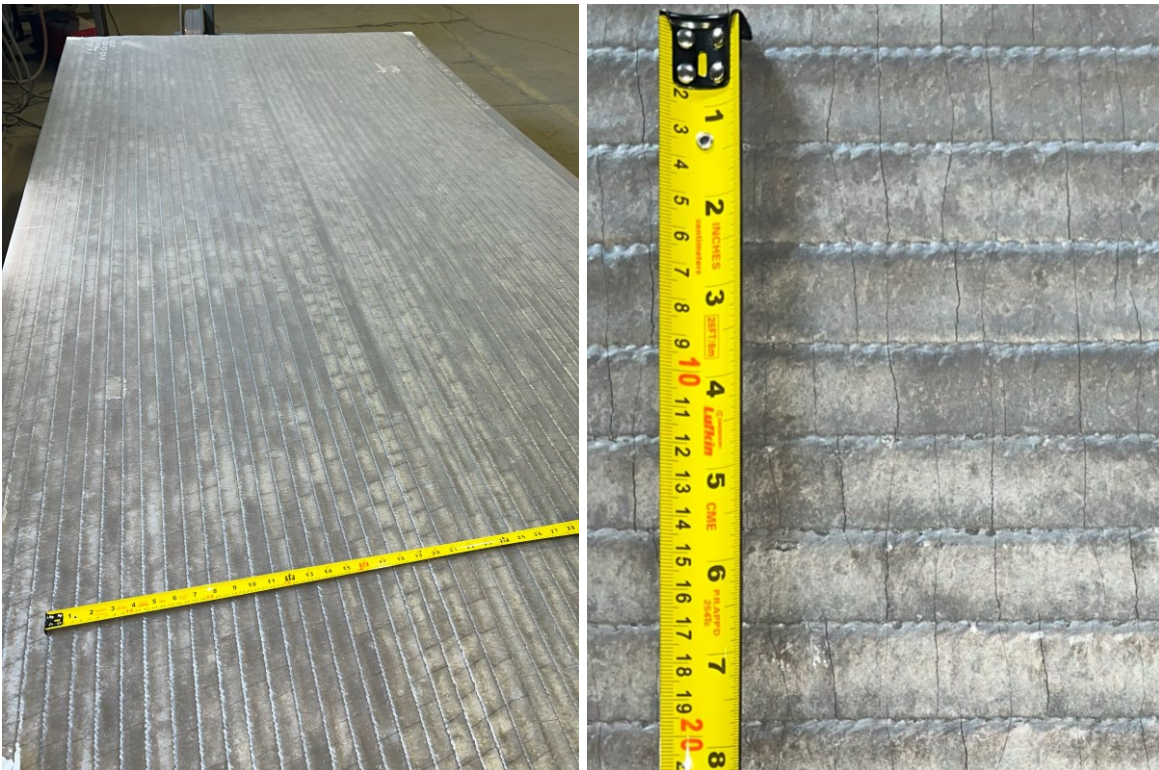
Figure 2.3: (a) chromium carbide overlay on a 5' × 10' mild steel plate produced by submerged arc welding and (b) details of the relief cracks on the same plate.
