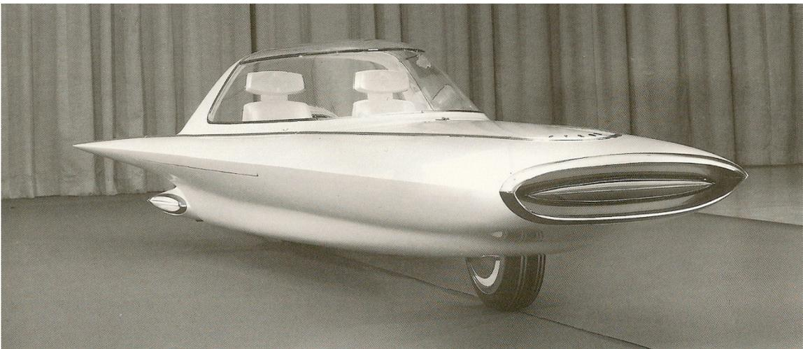
In 1967, a California-based company Gyro Transport Systems built another gyro-stabilized prototype car known as the Gyro-X.<sup>62</sup> The vehicle was invented by Thomas O.
