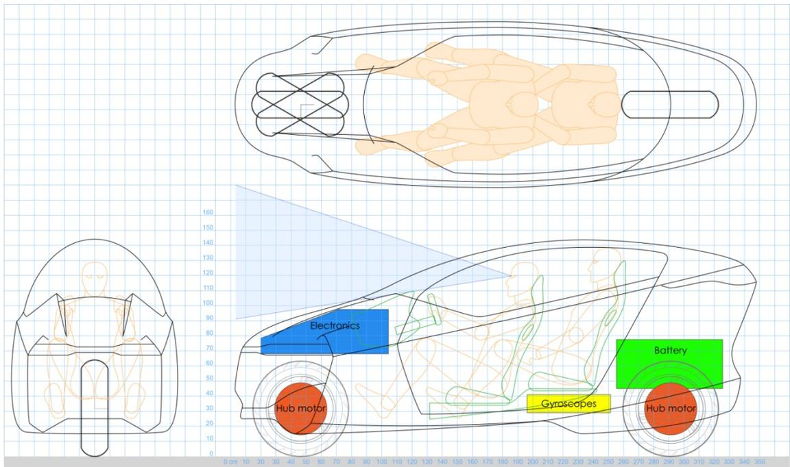
As can be seen in Figure 5.9, the design can carry two 95<sup>th</sup> percentile males and minus the space for main components, there is still plenty of space for equipment storage for each different emergency service. For the fire rescue version which is a single-seater, the rear seat will be replaced with a light weight aerial ladder.
