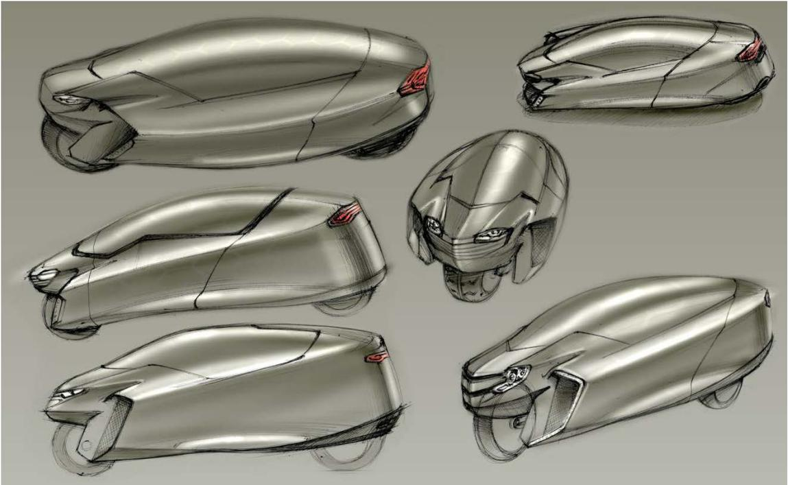
Figure 5.5. Adjusted side air-intakes of RapiDES.
