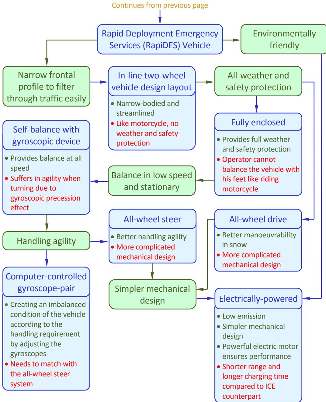
The mapping exercise continues in Figure 3.6 which shows the logical thought process of formulating the basic requirements and key features of the design of RapiDES. The most important requirement of RapiDES is to have a narrow frontal profile, which is having a narrow body width, in order to be streamlined enough to filter through traffic effortlessly, even in a gridlock situation. Figure 3.7 shows that a narrow-bodied RapiDES will filter through (lane splitting) traffic with ease.
