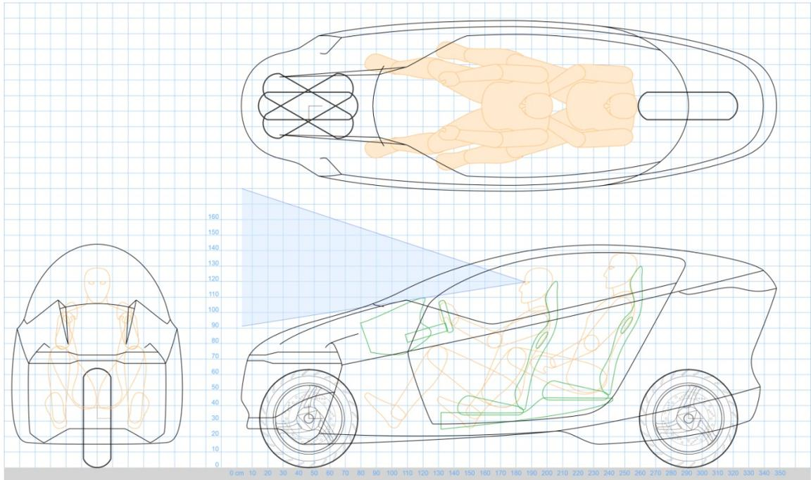
Figure 5.9. Main component layout of RapiDES.
