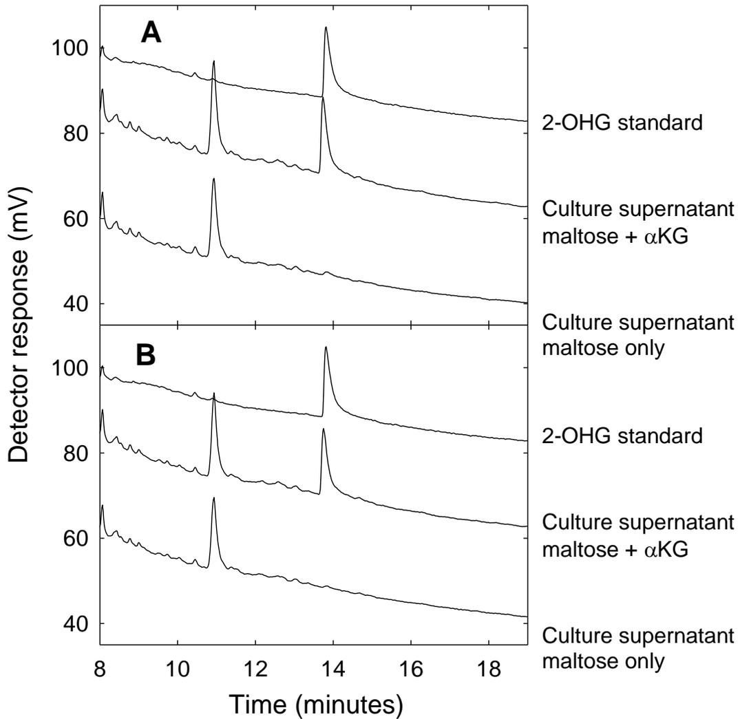
**Figure 3.1.** Gas chromatographic quantification of 2-OHG produced by *L. sanfranciscensis* (Panel A) and by *L. reuteri* (Panel B) in mMRS media containing maltose and  $\alpha$ -KG as substrates. Upper traces, injection of  $4 \text{ mM L}^{-1}$  2-OHG standard; middle traces, culture supernatant of mMRS containing 23 mM maltose as carbon source and 10 mM  $\alpha$ -KG as electron- or amino group acceptor; lower traces, culture supernatant of mMRS containing 23 mM maltose.
