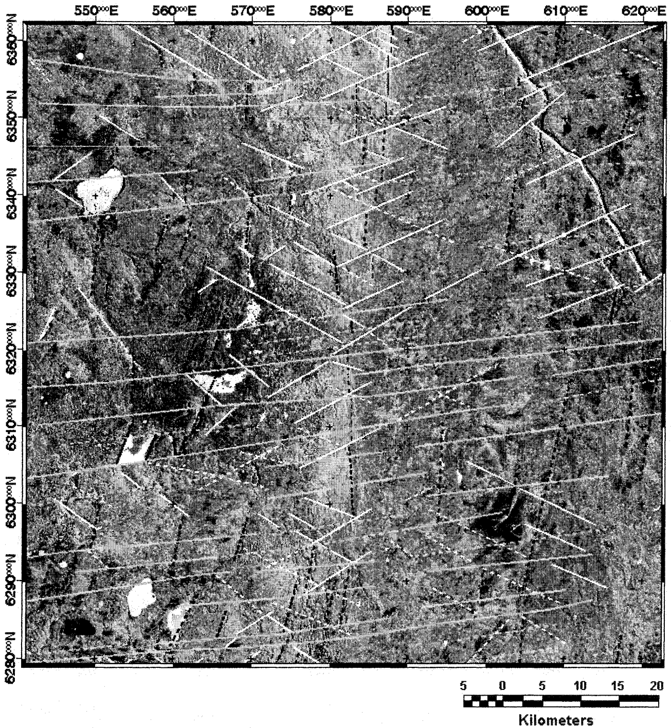
Figure 3.18B. RADARSAT-1-PC2 subset structural interpretation map.
