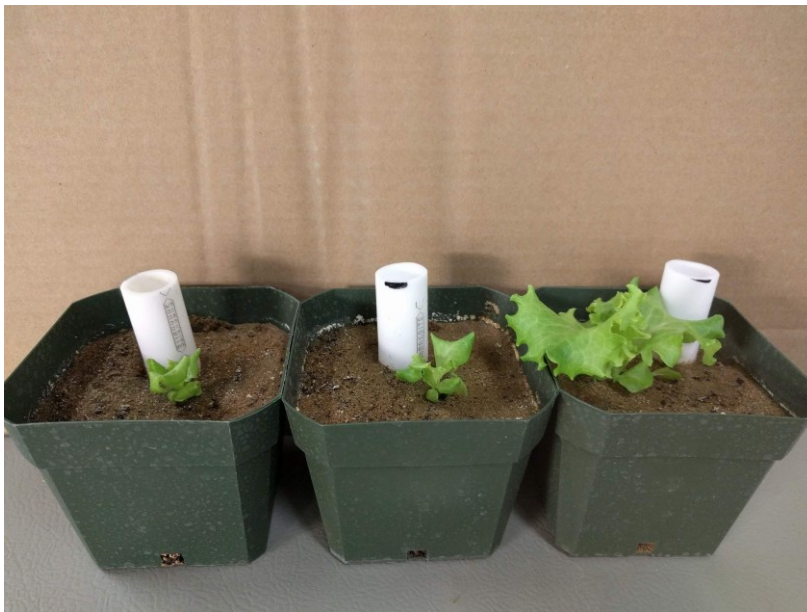
Figure S2.2 Lettuce ( Lactuca sativa ) grown in greenhouse pots (Growers Solution, Cookville, Tennessee, USA) filled with lean oil sand (LOS) and capped with field soil. Top image shows a water tile allowing the water to drain below the soil cap. Bottom image shows greenhouse pots with water tiles filled with High LOS, Low LOS, or field soil (left to right).
