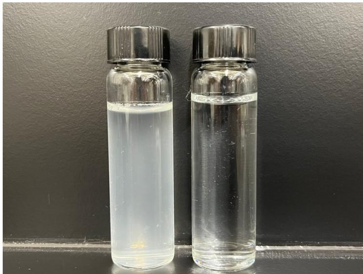
Figure 4.3. Photographs of Snomax suspensions (0.01 wt% stock solution (left) and 0.0005 wt% suspension (right)).
