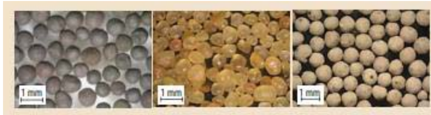
Fig. 1.10: Several proppant types. (a) High-strength bauxite (b) Resin-coated silica (c) Lightweight ceramic. 18
