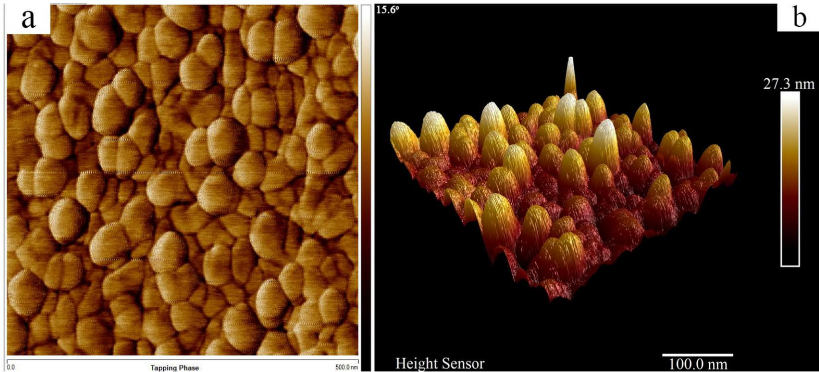
Figure 4.10: a) Phase image atomic force micrograph of the surface of the GaN films b) a three-dimensional reconstruction of the surface contour, extracted from the AFM height sensor data.
