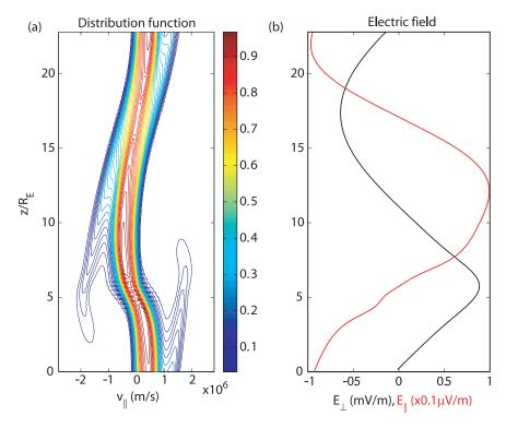
**Figure 3.** The left panel shows the electron distribution function as a function of  $\nu_{\parallel}$  and the spatial coordinate along the field line. The right panel shows the corresponding wave electric field components perpendicular and parallel to the geomagnetic field. The electron temperature corresponds to  $T_e = 0.5 \text{ eV}$ , with  $\nu_A = 1.42 \times 10^6 \text{ ms}^{-1}$  and  $\nu_{th} = 4.19 \times 10^5 \text{ ms}^{-1}$ .
