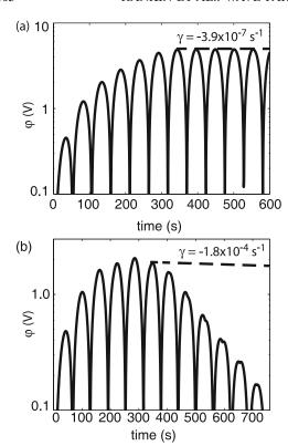
**Figure 1.** Growth of perpendicular electric field as a function of time in cold plasma with  $T_e = 0.5$  eV. The wave frequency is approximately 10 mHz. The perpendicular wavenumber corresponds to  $k_{\perp} = 2 \times 10^{-5}$  m<sup>-1</sup> in (a) and  $k_{\perp} = 1.5 \times 10^{-4}$  m<sup>-1</sup> in (b). In both (a) and (b),  $\nu_A = 1.42 \times 10^6$  ms<sup>-1</sup>, and  $\nu_{th} = 4.19 \times 10^5$  ms<sup>-1</sup>.
