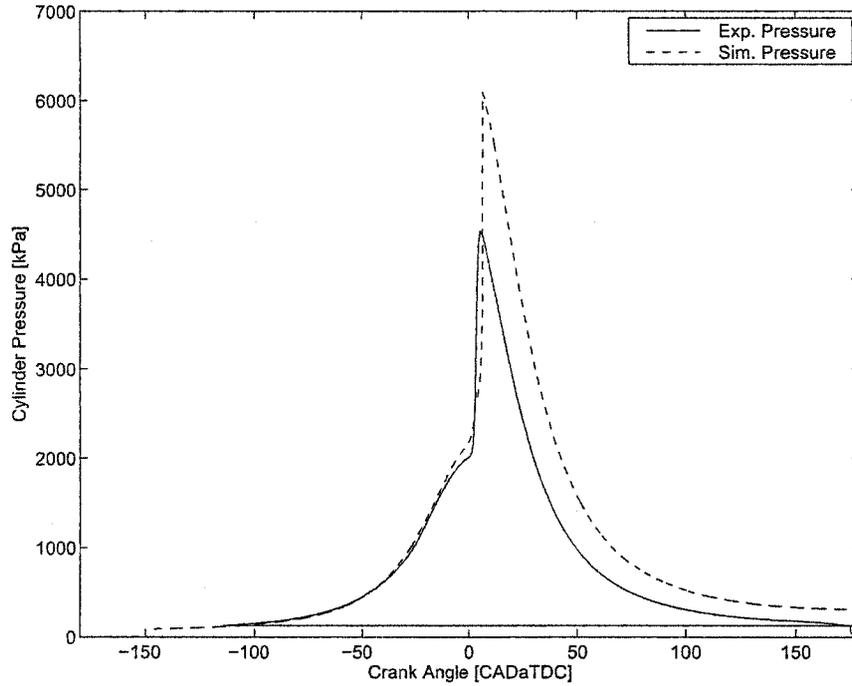
Figure 4.10: Comparison of calculated and experimental pressure histories using 60PRF fuel. Experimental pressure history from Atkins (2004).  $T_{o,sim} = 360\text{K}$ ,  $\phi_{ign,exp} = 1.8 \pm 1.9\text{CAD}$ ,  $\phi_{ign,sim} = 1.3\text{CAD}$ ,  $T_{wall} = 390\text{K}$
