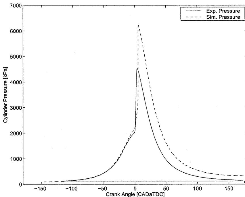
Figure 4.9: Comparison of calculated and experimental pressure histories using 40PRF fuel. Experimental pressure history from Atkins (2004).  $T_{o,sim} = 360\text{K}$ ,  $\theta_{ign,exp} = 0.4 \pm 1.4\text{CAD}$ ,  $\theta_{ign,sim} = 0.5\text{CAD}$ ,  $T_{wall} = 390\text{K}$
