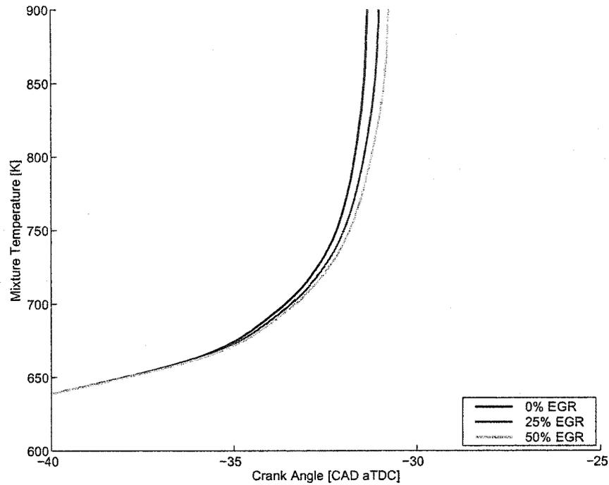
Figure 5.2: The effect of EGR addition on the ignition timing for fired HCCI operation, for mixtures with a constant specific heat capacity.  $ON=0$ ,  $N = 1000\text{rpm}$ ,  $T_o = 400\text{K}$ ,  $\Phi = 0.7$ ,  $P_o = 100\text{kPa}$ .
