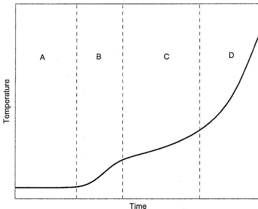
Figure 3.2: A characteristic temperature history of the two-stage autoignition of a hydrocarbon. Region A: Induction period, Region B: Cool flame, Region C:  $\dot{R}OOH$  and  $R'CHO$  formation, Region D: Hot ignition.
