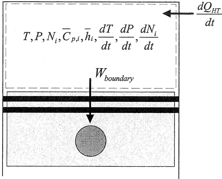
Figure 3.1: Control mass used in the one zone model. The thermodynamic state is assumed to be constant throughout the entire volume.
