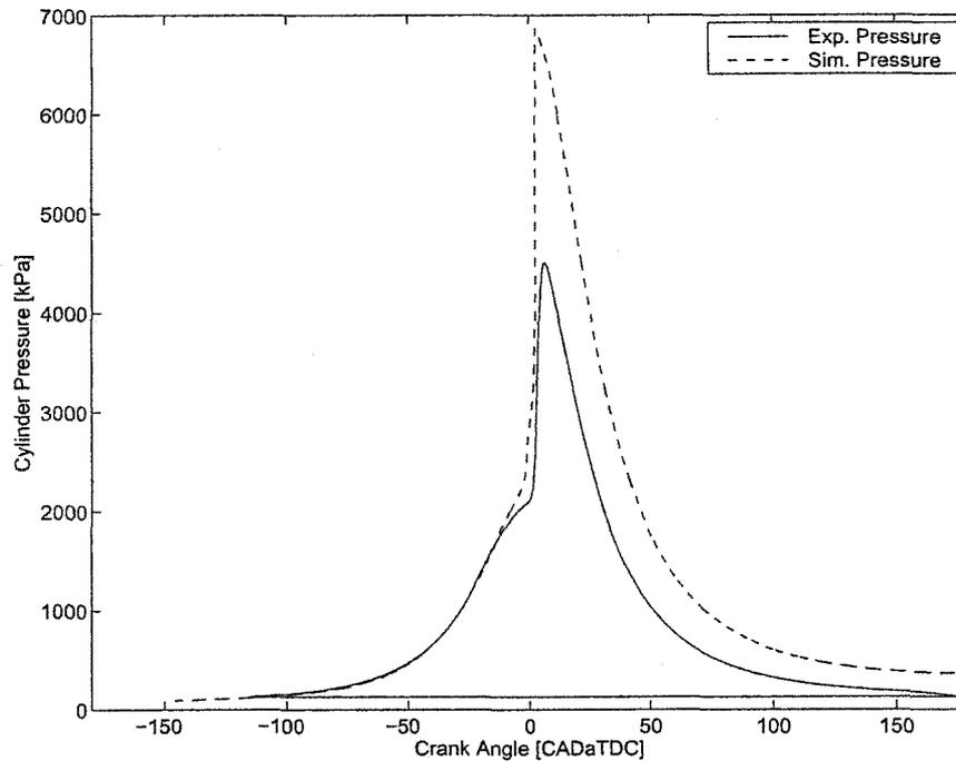
Figure 4.8: Comparison of calculated and experimental pressure histories using 20PRF fuel. Experimental pressure history from Atkins (2004).  $T_{o,sim} = 360\text{K}$ ,  $\theta_{ign,exp} = 1.1 \pm 1.7 \text{ CAD}$ ,  $\theta_{ign,sim} = -2.3\text{CAD}$ ,  $T_{wall} = 390\text{K}$
