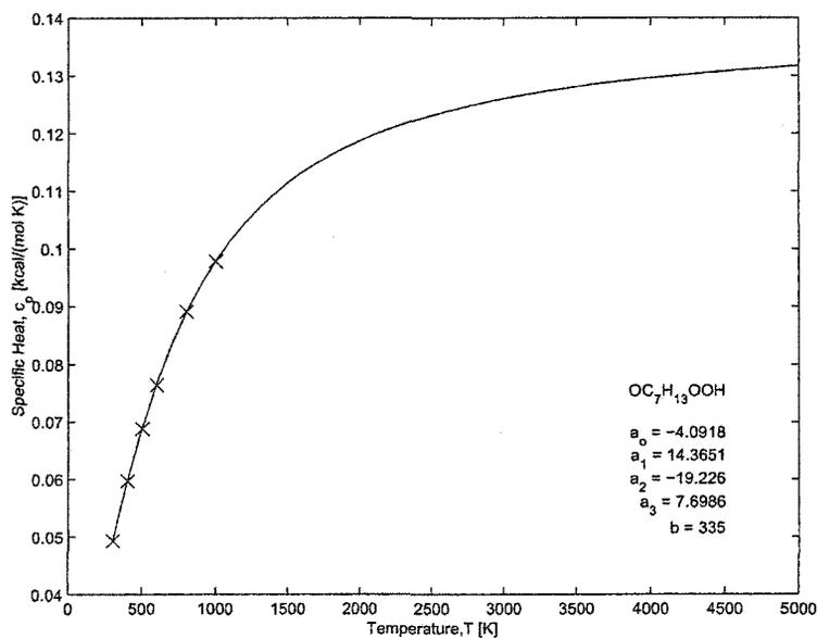
Figure B.14: Estimation of the specific heat of OC<sub>7</sub>H<sub>13</sub>OOH.
