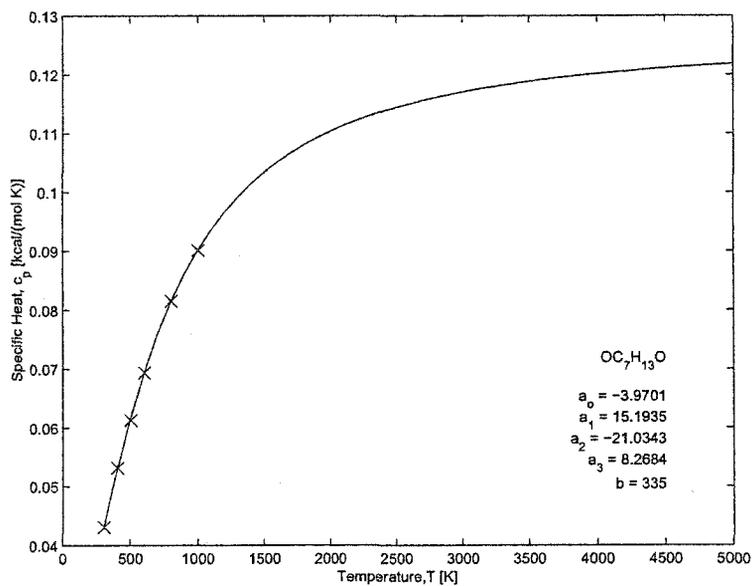
Figure B.13: Estimation of the specific heat of OC<sub>7</sub>H<sub>13</sub>O.
