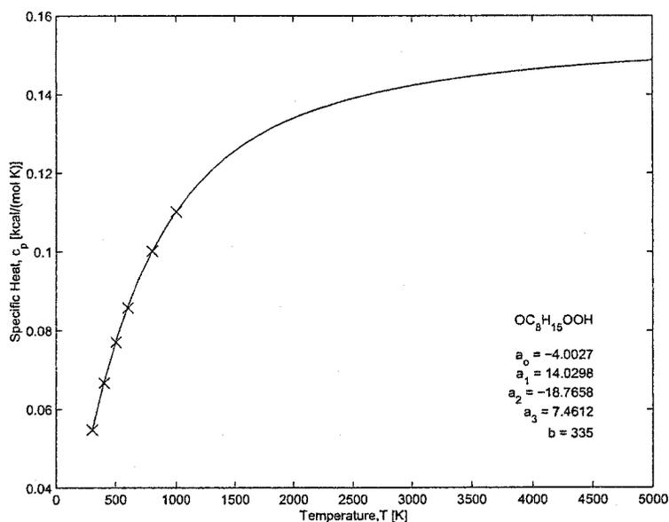
Figure B.16: Estimation of the specific heat of OC<sub>8</sub>H<sub>15</sub>OOH.
