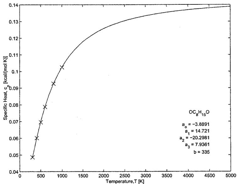
Figure B.15: Estimation of the specific heat of OC<sub>8</sub>H<sub>15</sub>O.
