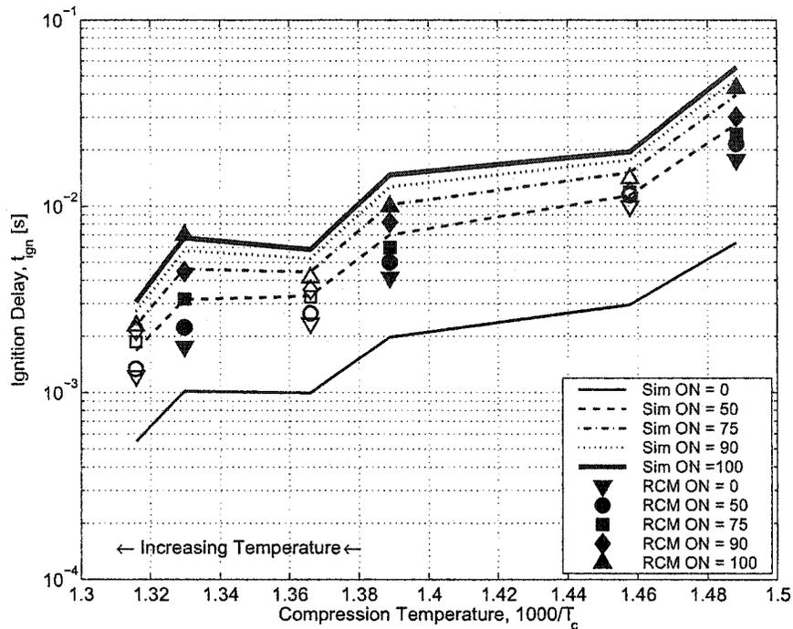
Figure 4.3: Comparison of measured (Park & Keck 1990) and calculated RCM ignition delays for various stoichiometric PRF blends. Hollow markers indicate initial pressure of  $\sim 5$ MPa and solid markers indicate initial pressures of  $\sim 2$ MPa.
