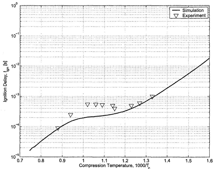
Figure 4.5: Comparison of calculated and experimental shock tube ignition delays taken from Fieweger et al. (1997).  $P = 40\text{bar}$ , stoichiometric n-heptane/air mixture. Simulations were carried out from 600K to 1200K in 20K increments.
