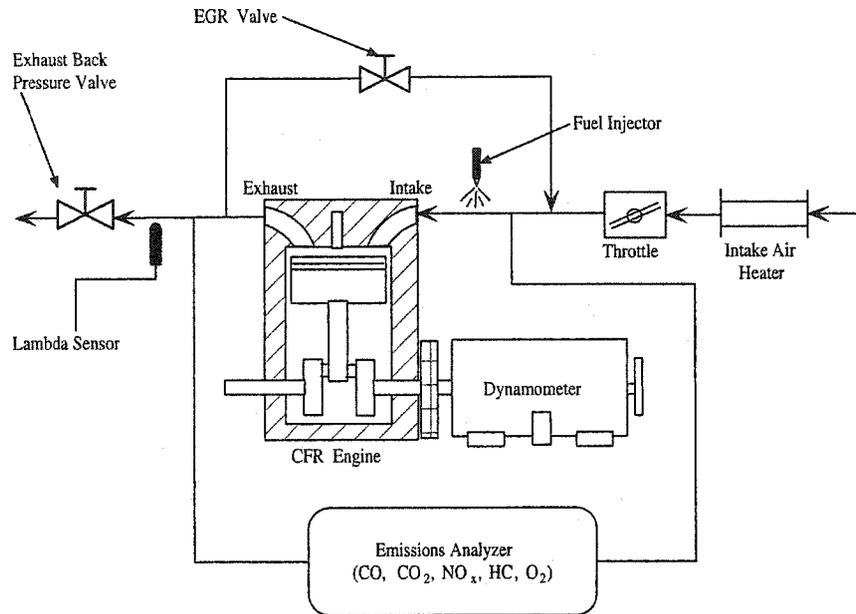
Figure 4.6: Schematic of the single cylinder CFR engine test bench (Atkins 2004)
