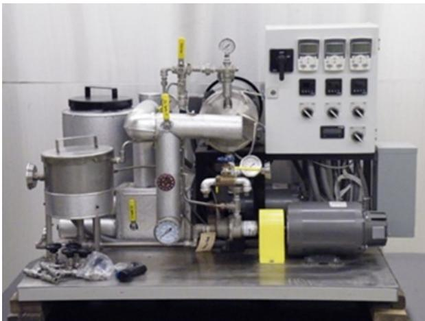
**Figure 3.1** Colloidal mill at Gecan (in Acheson, Alberta), where experiments were conducted.
