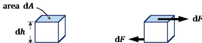
**Figure 2.1** An elemental volume of material under pure shear. The differential forces, both of equal magnitude  $dF$ , act tangent to the surfaces.
