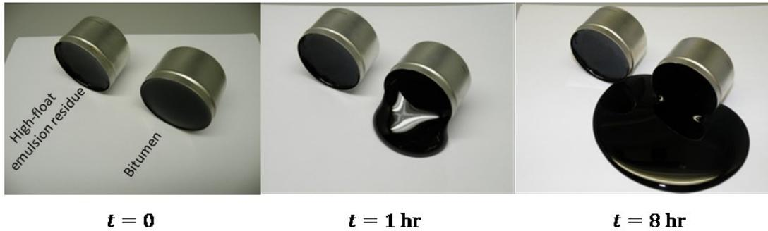
**Figure 1.6** Flow behaviours of bitumen (right) and a high-float emulsion residue (left) formed from the same bitumen. The ambient temperature was 23°C.
