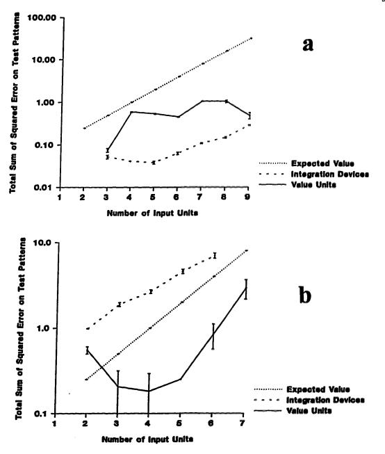
Figure 10: (a) Median total sum of squared error for networks on the 25% of the patterns not presented during training on the majority problem using a logarithmic scale (b) Median total sum of squared error for networks on the 25% of the patterns not presented during training on the parity problem using a logarithmic scale.
