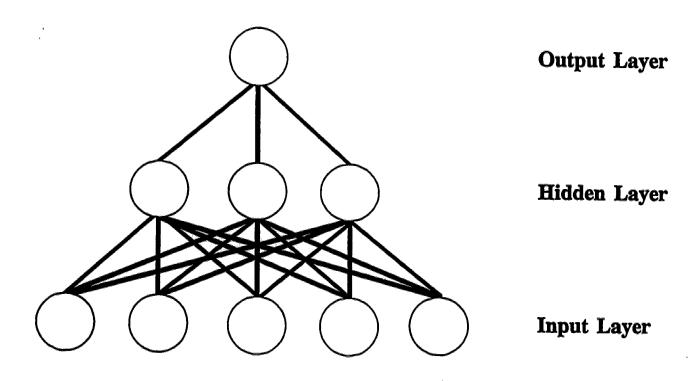
Figure 1 : A multilayer PDP network constructed from massively parallel connections between three layers of processing units.
