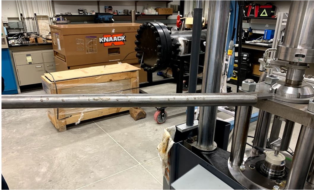
Figure B The picture of snipe bar/extension arm to turn thrust nut spanner wrench when applied axial force to the sample.
