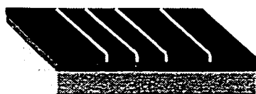
3. Developing the photoresist
