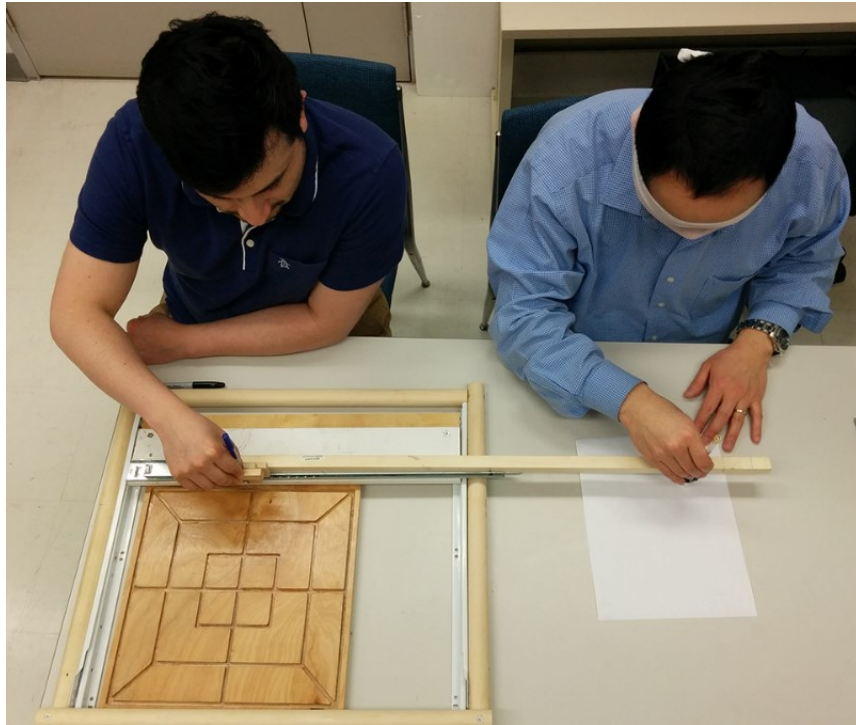
Figure 4-2. Experimental setup: The kinesthetic guidance device shares the kinesthetic information between the master and the trainee.
