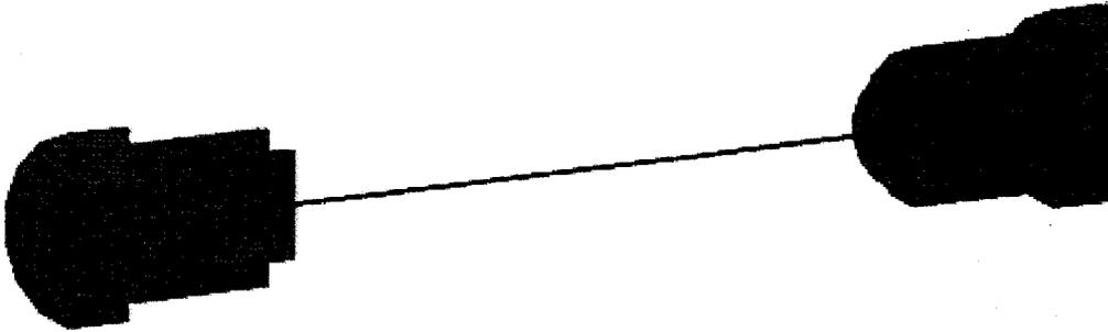
Figure 4.14: The beam pipe I model as beryllium. The forward shielding is solid iron and I build it as a cylinder of staggered outer radius. It has an inner radius of 3.7 cm, lying jut outside of the beam pipe.
