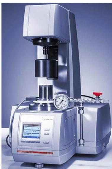
Figure 7.2 Anton Paar Rheometer MCR 302 for measuring dynamic viscosity and shear stress at different shear rate, and viscoelastic components  $G'$  (storage modulus) and  $G''$  (loss modulus) at different angular frequency.
