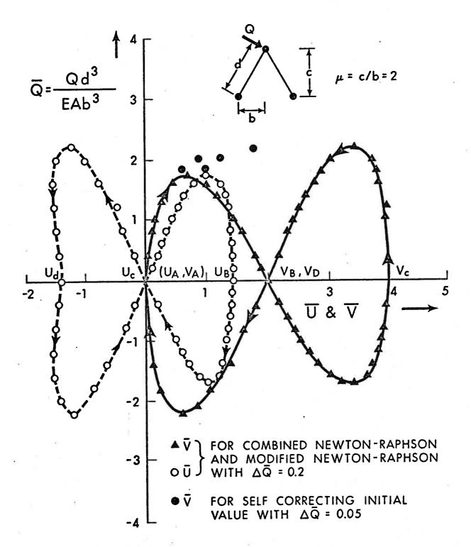
FIG. 15 - SOLUTIONS FOR TWO BAR TRUSS ( $\mu$ =2.0) WITH NON-CONSERVATIVE LOADING
