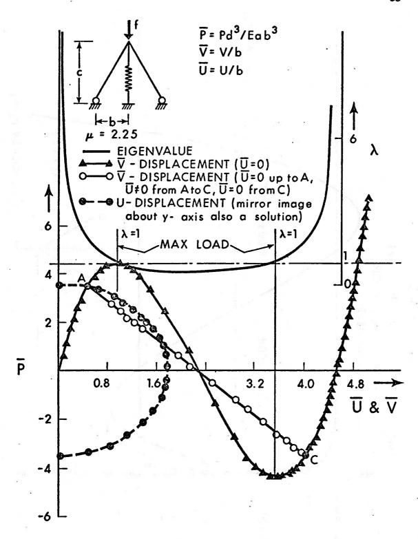
FIG. 11 - SOLUTIONS FOR TWO BAR TRUSS ( $\mu$  = 2.25)
