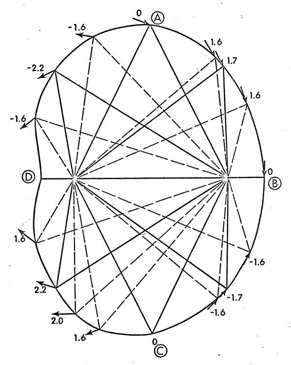
FIG. 16 - DISPLACED CONFIGURATIONS OF TWO BAR TRUSS (  $\mu$  = 2.0) WITH NONCONSERVATIVE LOADING
