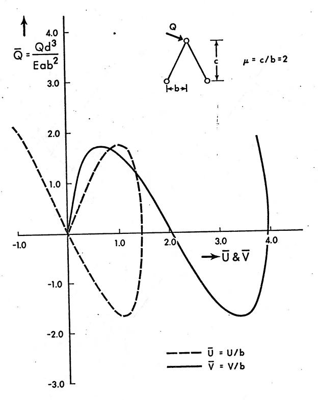
FIG. 17 - AUGMENTED STIFFNESS SOLUTION FOR TWO BAR TRUSS ( $\mu$  = 2.0) WITH NONCONSERVATIVE LOADING
