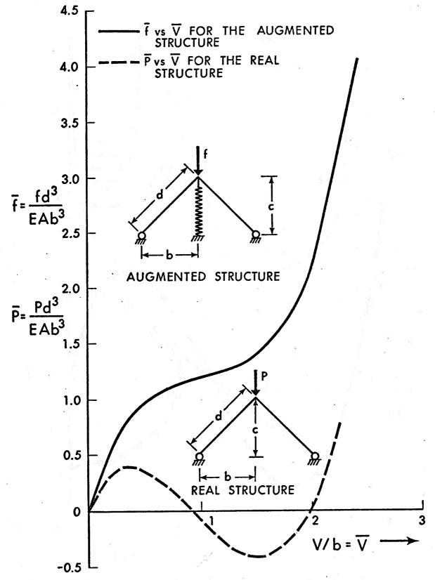
FIG. 10b - LOAD - DEFLECTION CURVES FOR AUGMENTED AND REAL STRUCTURES
