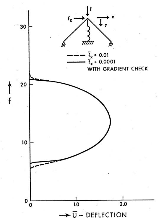
FIG. 13b - AUGMENTED STIFFNESS DISPLACEMENT WITH DISTURBING FORCES ( $\mu$  = 2.25)
