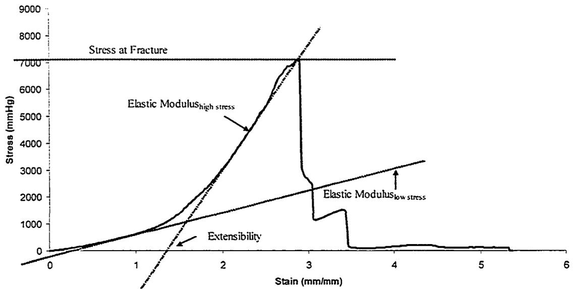
**Figure VI-1. Study methods: analysis of stress-strain curves.** Stress-strain curves were analyzed to determine stress at fracture, low stress (alignment) and high stress (stiffness) elastic modulus, and extensibility. (Adapted from Barber et al. *J Thorac Cardiovasc Surg* 2001;122:955-62).
