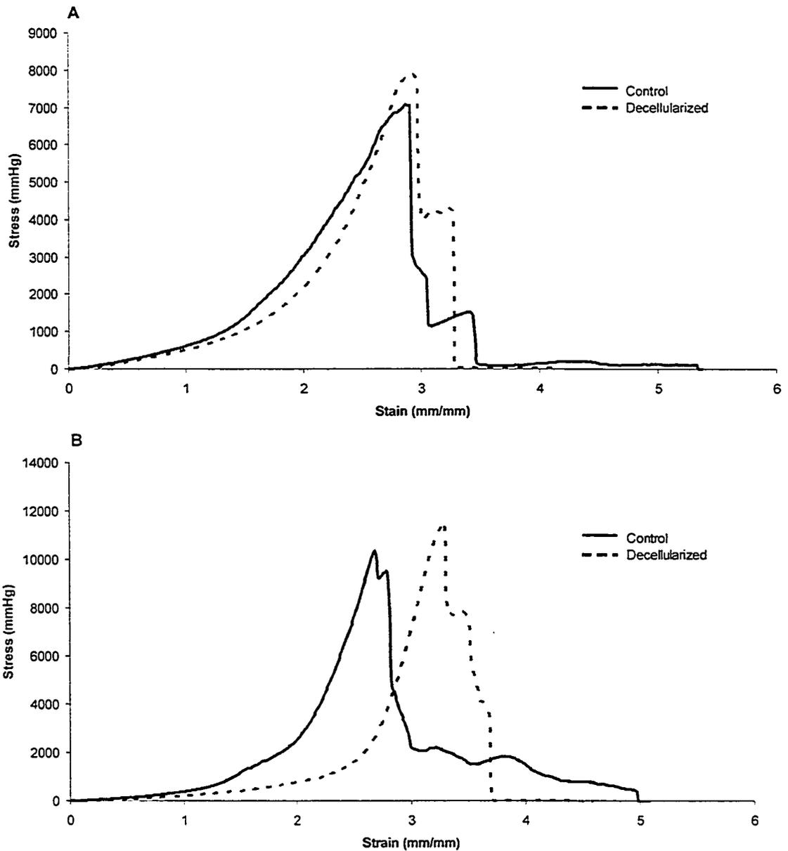
**Figure VI-3. Representative stress strain curves for control (nondecellularized) and decellularized porcine aortic wall and pulmonary trunk. Decellularization was associated with minimal changes in the biomechanical properties of (A) aortic wall and modest changes to (B) pulmonary trunk in these sample stress strain curves.**
