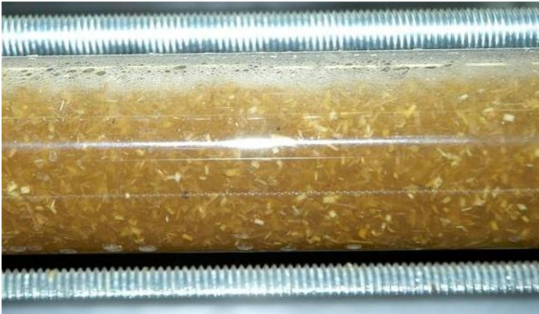
Figure 17: Air bubbles seen in viewing section
