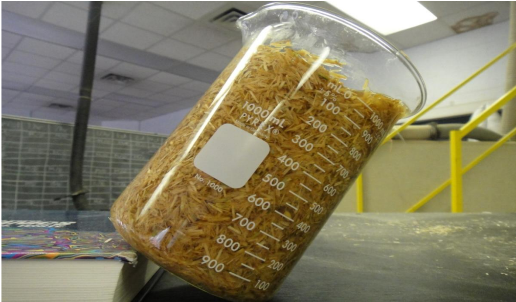
Figure 37: 40% concentration slurries are not flowable
