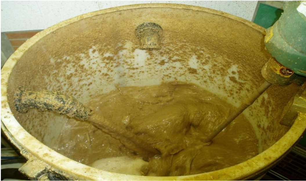
Figure 18: Slurry splashing caused by mixer and mixing tank inlet
