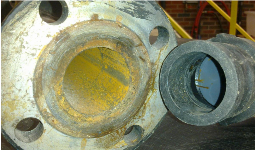
Figure 35: Inner diameter of cam lock fittings are 1/4" less than steel pipe
