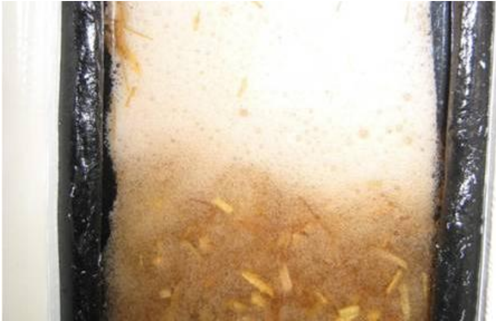
Figure 26: Air dissipating from slurry accumulates as bubbles on surface
