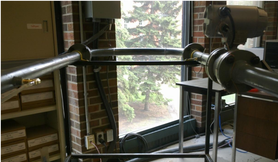
Figure 22: Pressure taps and flow meter are placed away from bends
