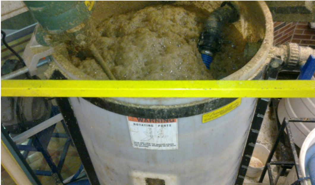
Figure 25: Mixing tank inlet submerged to allow air bubbles to dissipate
