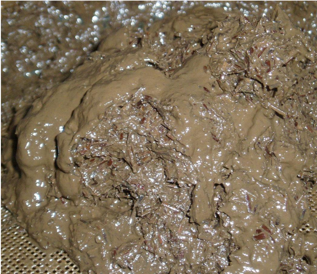
Figure 7: Carrier fluid impurities concentrated on the surface of wet straw
