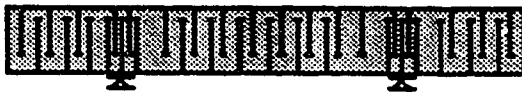
Members with continuous overlapping shear connectors which provide compatibility between the concrete core and the steel plates
