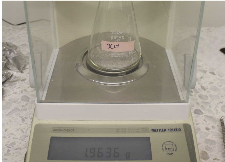
Figure 5.9. Weighing for initial weights of powdered samples and crucibles
