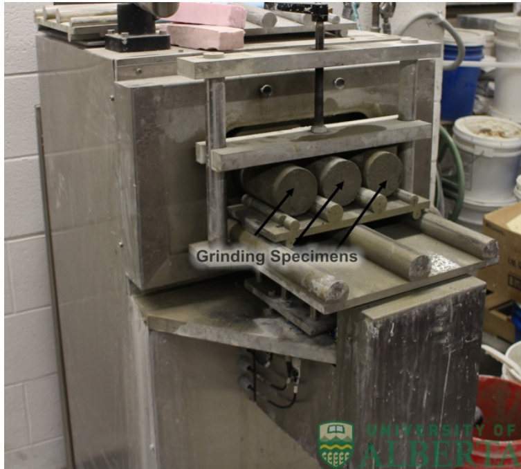
Figure 3.6. Grinding machine with three cylindrical samples
