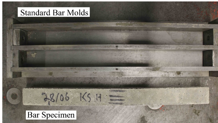
Figure 3.3. Bar molds used and length change bar specimen after de-molding
