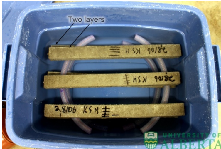
Figure 3.1. 11L container storing six length change bar specimens
