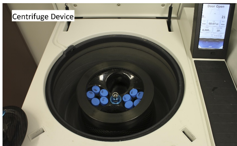
Figure 5.13. Symmetric centrifuge setup (8,000 xg at 20 centigrade)
