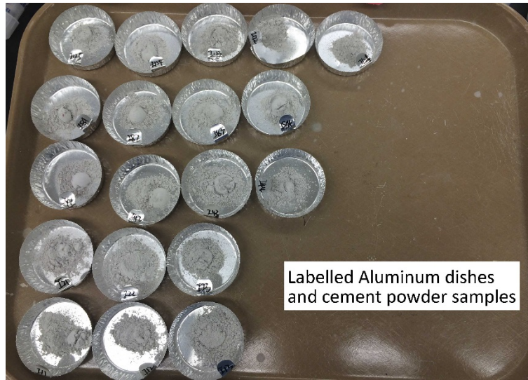
Figure 5.7. Labelled powdered samples after oven-drying
