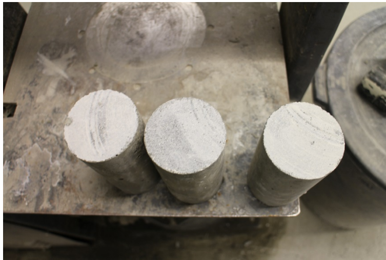
Figure 3.7. Grinded surface of cylindrical sample prior to test
