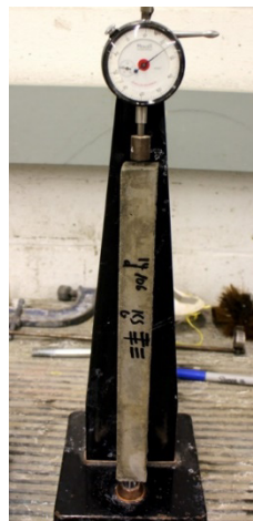
Figure 3.4. Length comparator employed for length change measurement
