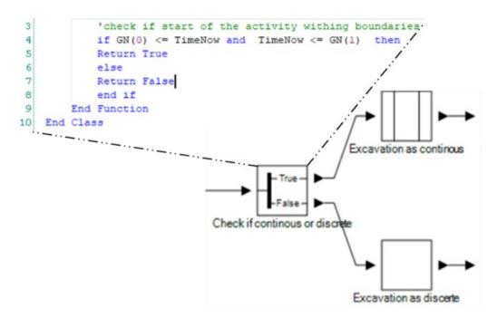
Figure 6.9. Modelling of weather-sensitive activity.
