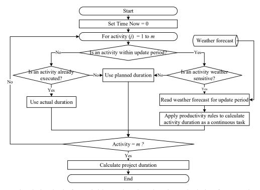
Figure 6.5. Simulation logic for activities and project duration calculation for an update period.
