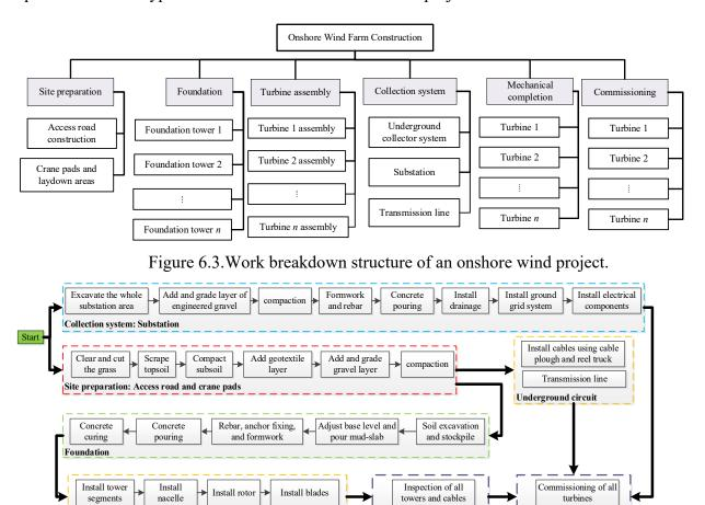
Figure 6.4. Detailed activities and sequence of work for an onshore wind project.
