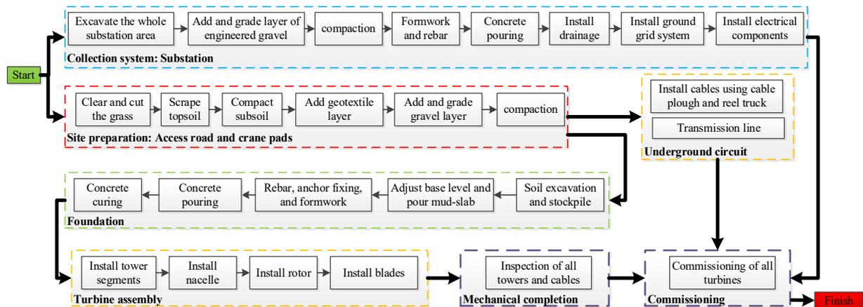
Figure 6.4. Detailed activities and sequence of work for an onshore wind project.
