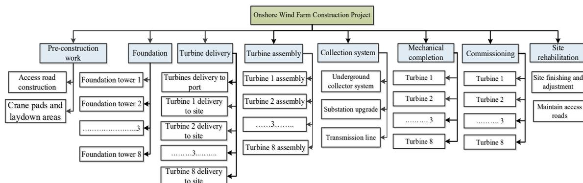
Figure 5.4. Work breakdown structure of case study.
