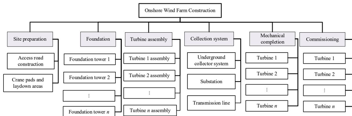
Figure 6.3. Work breakdown structure of an onshore wind project.
