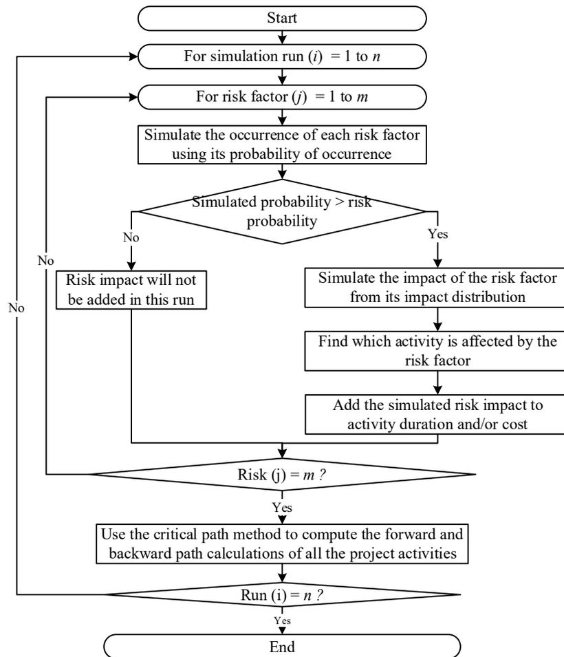
Figure 5.2. Simulation logic of MCS-CPM method.
