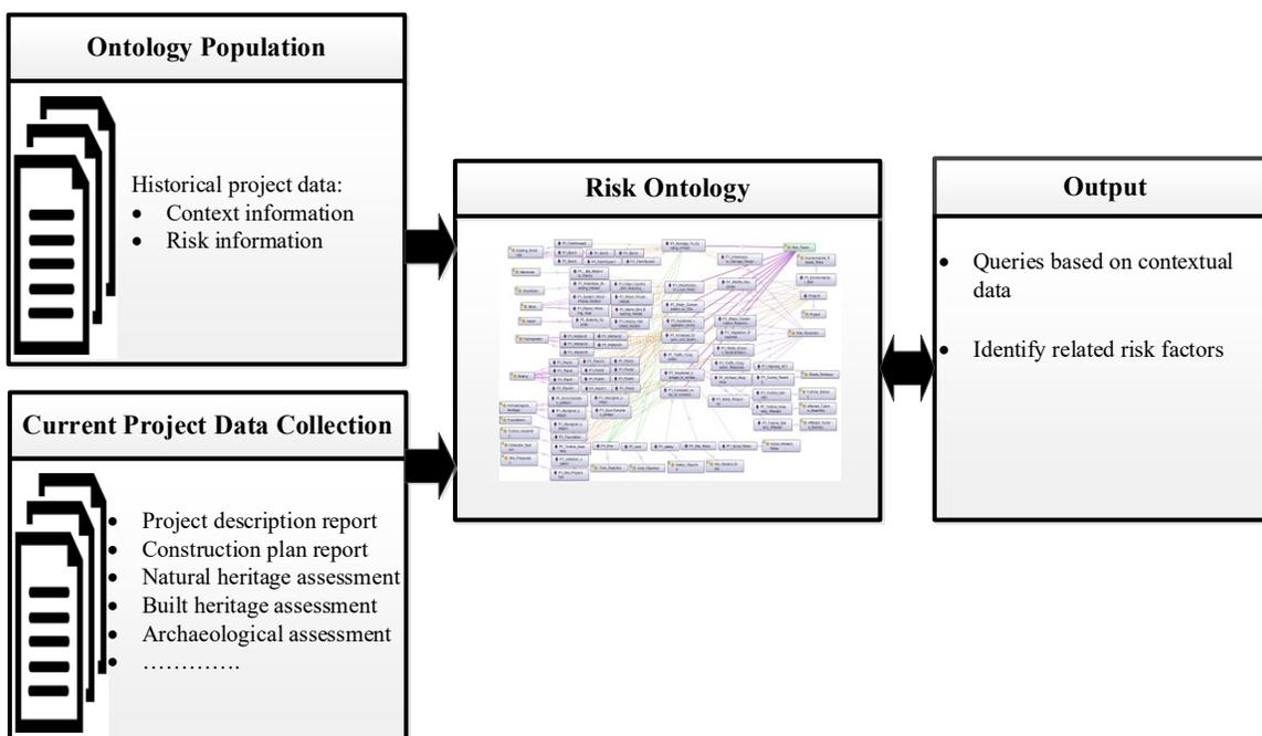
Figure 3.1. Proposed ontology-based framework for risk identification.
