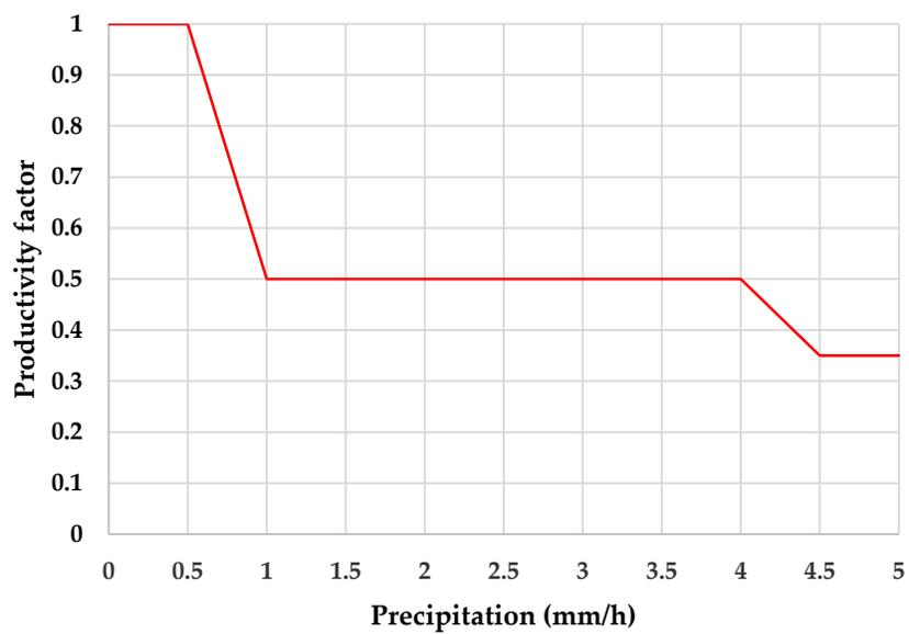
Figure 6.7. Effect of precipitation on construction productivity based on results from (Larsson and Rudberg 2019).
