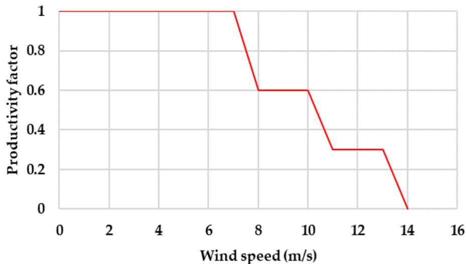
Figure 6.8. Effect of wind speed on construction productivity of crane based on results from (Guo et al. 2017b).
