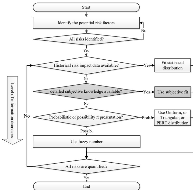
Figure 4.1. Levels of data available and accompanying methods used for input modelling.
