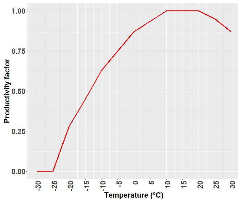
Figure 6.6. Effect of temperature on construction productivity based on results from (Moselhi and Khan 2010).
