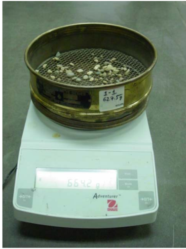
Figure 3-11. Left: a snapped image of weighing dry sands remaining in a sieve; Right: the image of sieve stack in a shaker machine
