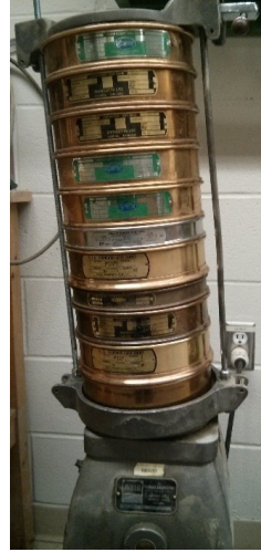
Figure 3-11. Left: a snapped image of weighing dry sands remaining in a sieve; Right: the image of sieve stack in a shaker machine
