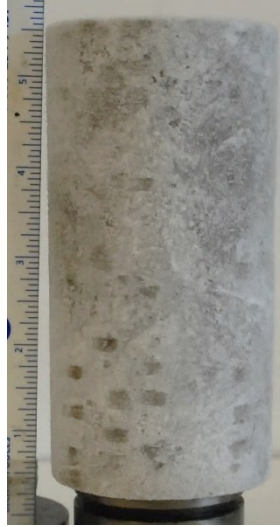
Figure 3-26. Sands core specimen used in one test prior to conducting the triaxial compression test
