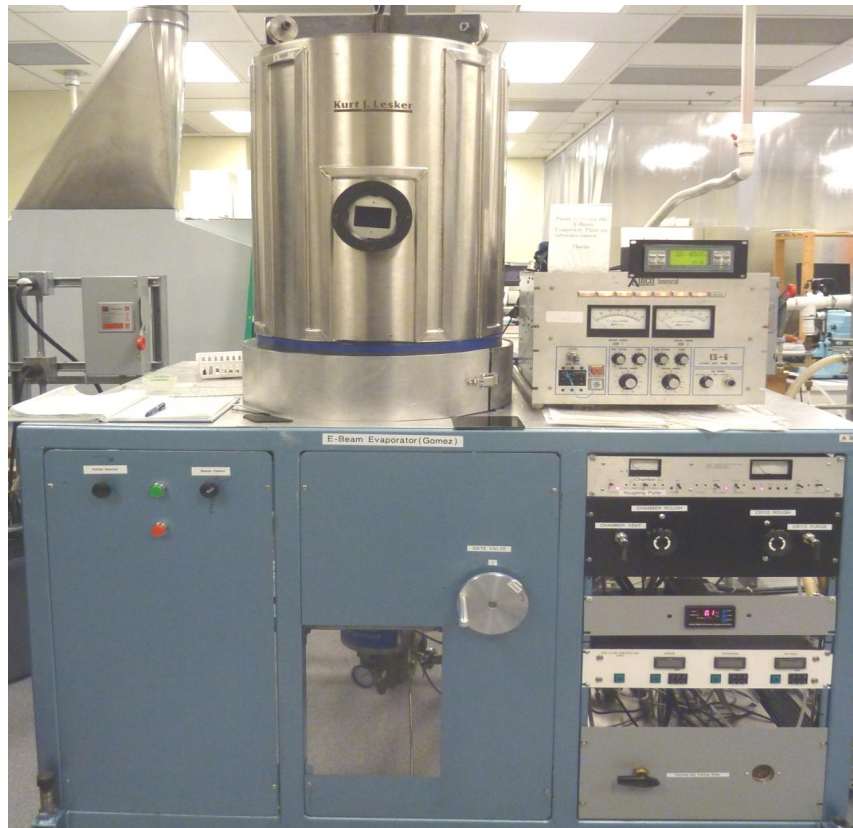
Figure 4-1 Electron beam deposition system used in the project
