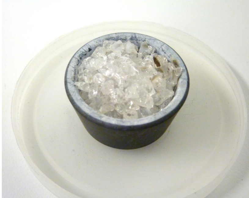
Figure 4-2 Used alumina source grains in coated graphite crucible
