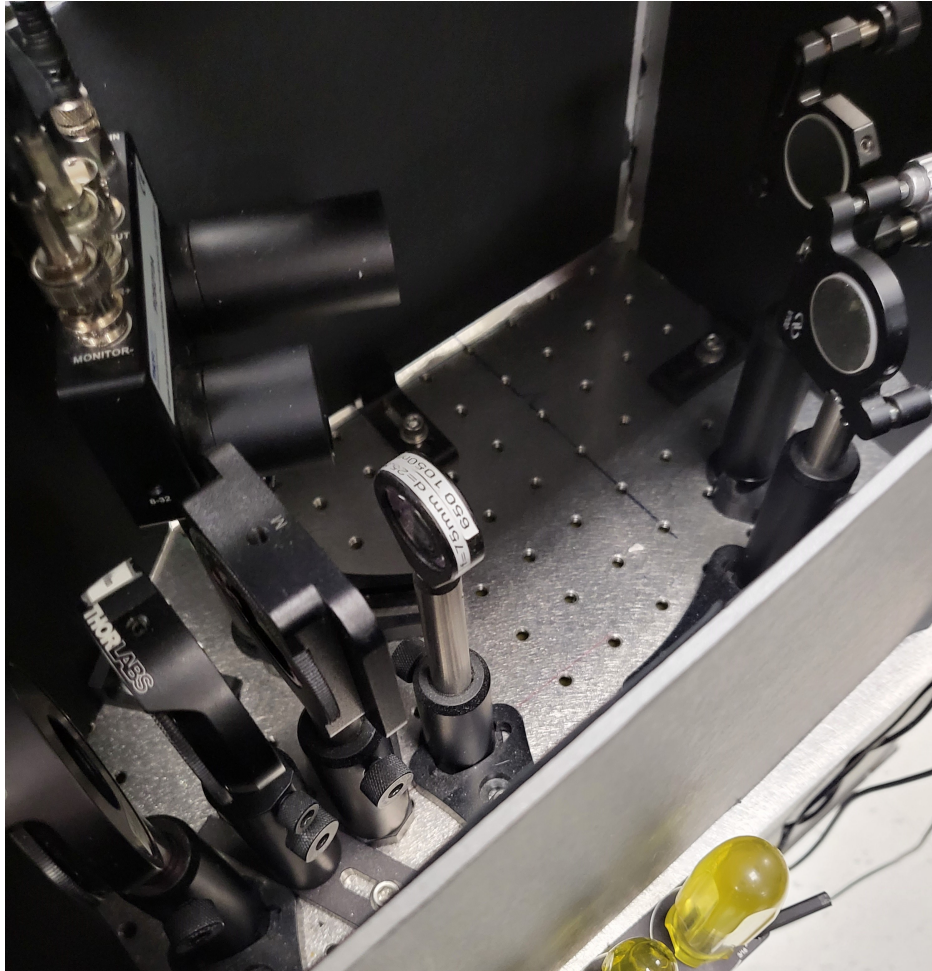
Figure 4.2: Light box enclosure of the main electro-optic sampling (EOS) apparatus. The Light box enclosure was added to prevent pollution from ambient light. A lid (not shown) with holes cut out for the photodiode connectors is placed on top. When balancing the photodiodes the only optics that are adjusted are the quarter-wave plate and the alignment of the mirrors used to guide light to the photodiodes.
