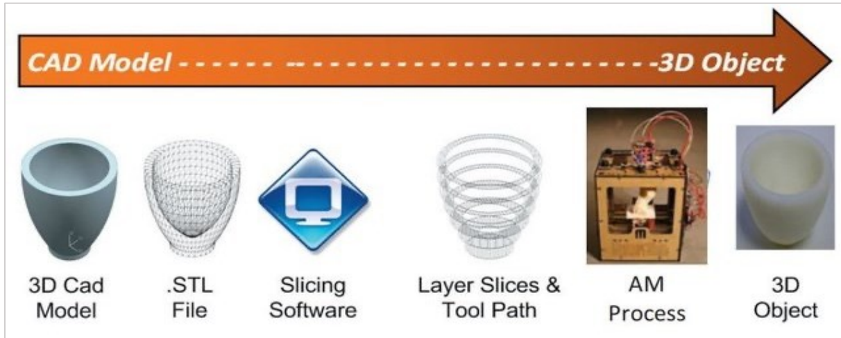
Figure 1.4 Schematic of 3DP process step-by-step (Campbell et al, 2011)
