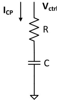
**Figure 2.7 2<sup>nd</sup> order LF with series resistance to ensure stability of the system**
