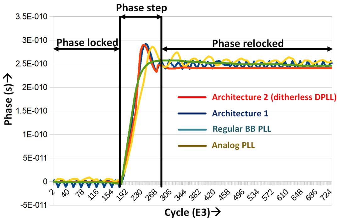
Figure 3.25 Phase step response of VCO clocks for 4 different PLL architectures
