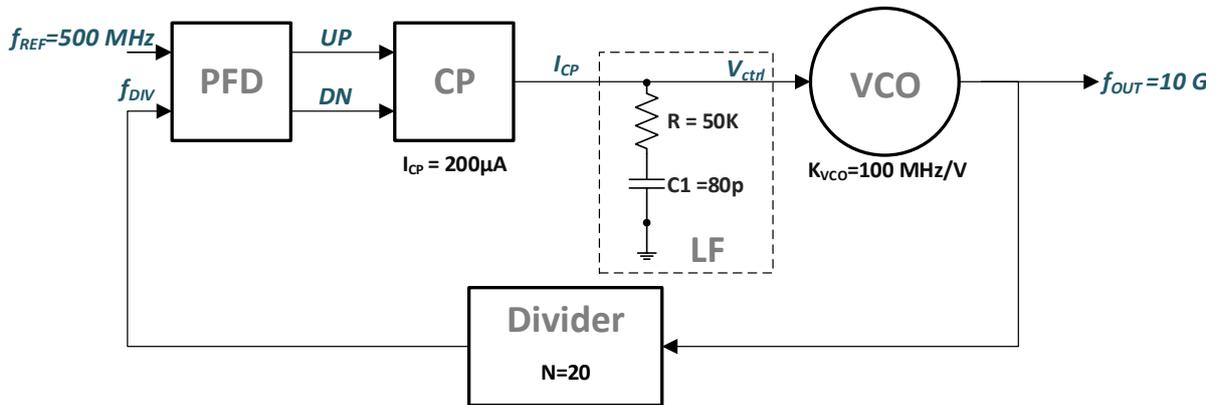
Figure 2.20 APLL circuit simulated in Cadence AMS environment
