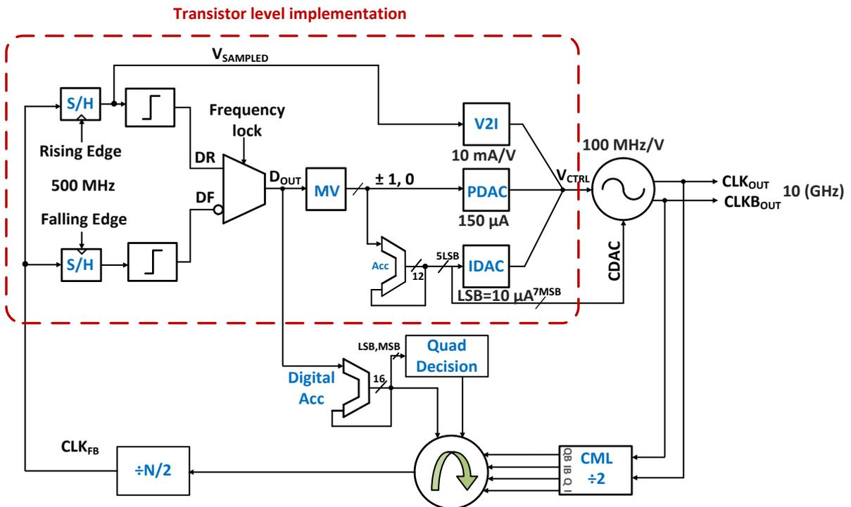
Figure 3.19 DPLL Architecture 2: ditherless DPLL with dual edge sampled Hybrid PD and mixed mode phase accumulator
