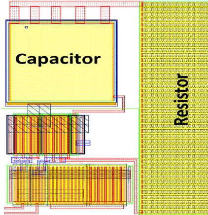
*Figure 4.17 Layout view of V2I circuit*
