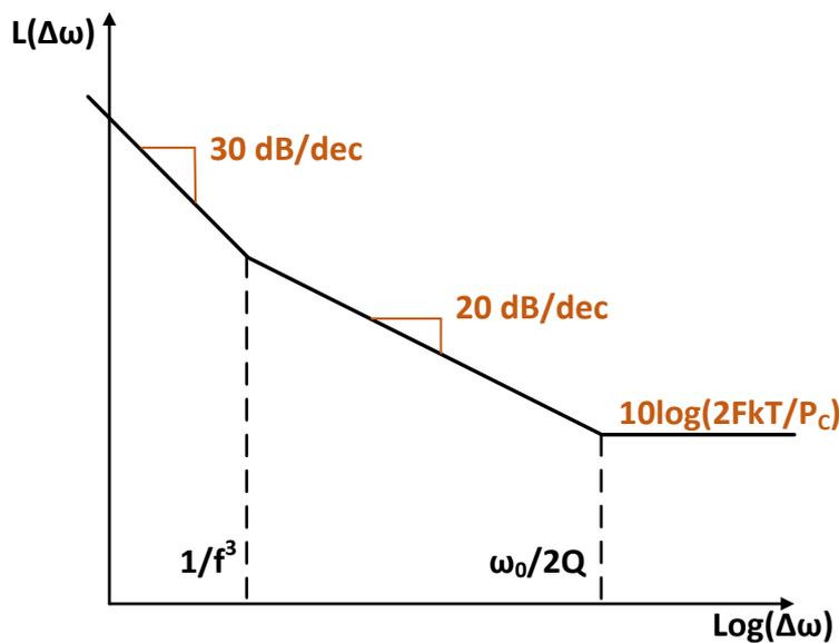
**Figure 2.4 Graphical representation of Leeson phase noise characteristic for an oscillator**
