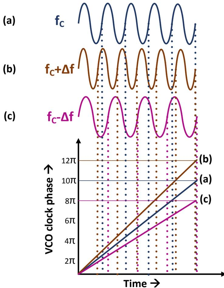
*Figure 3.1 Phase error accumulation of VCO for a frequency error of  $\Delta f$*
