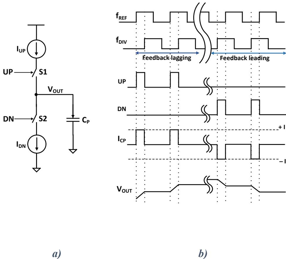
**Figure 2.6 Operation of Charge Pump: a) Basic block diagram b) Variation of output current  $I_{CP}$  and loop filter voltage  $V_{OUT}$  with UP/DN signals of PFD**
