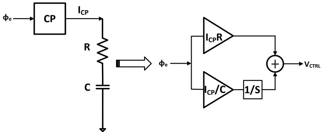
Figure 2.13 Proportional and Integral gains of Loop Filter
