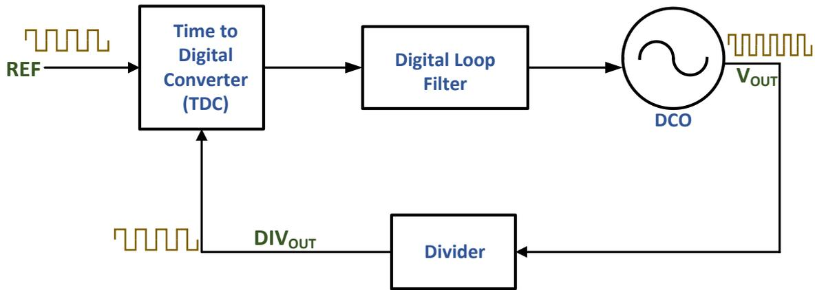
*Figure 2.9 Conventional Digital PLL architecture*
