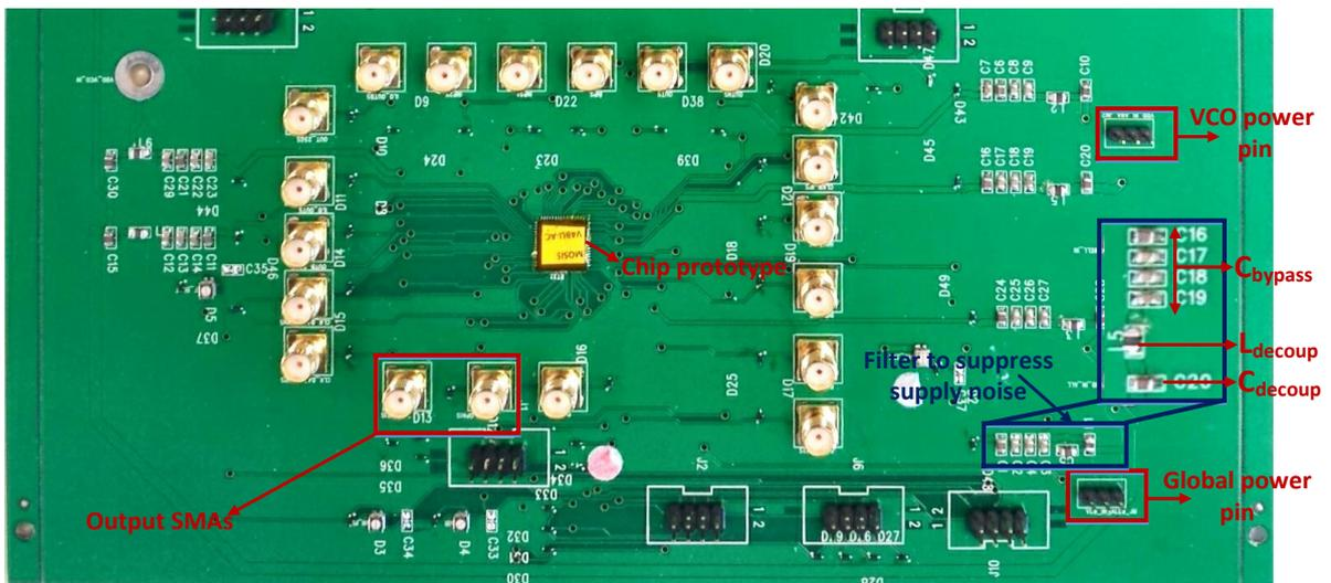
Figure 5.2 PCB board used to test chip prototype
