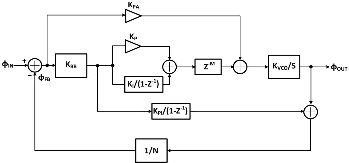
Figure 3.15 Linearized model for proposed DPLL (Architecture 2)
