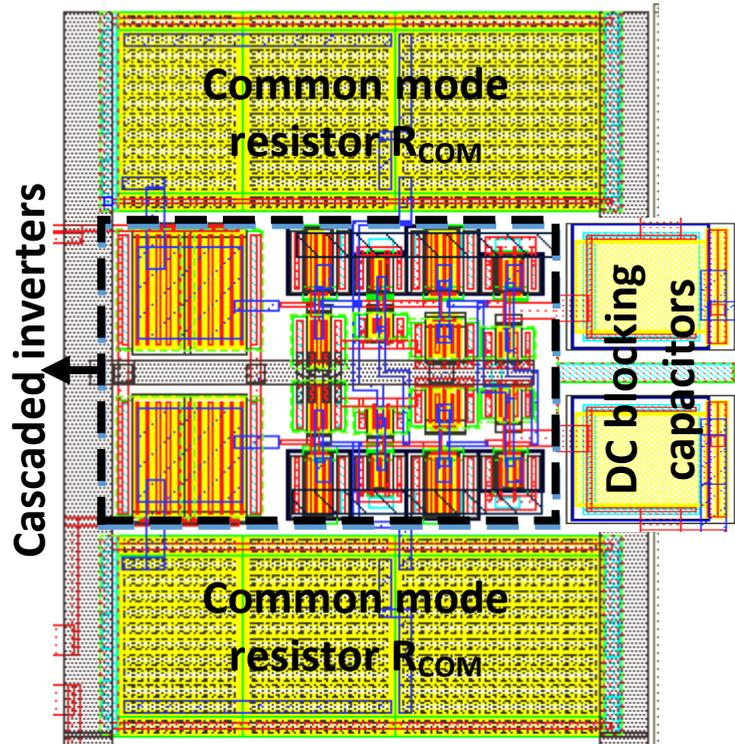
*Figure 4.10 Layout view of Decision circuit*
