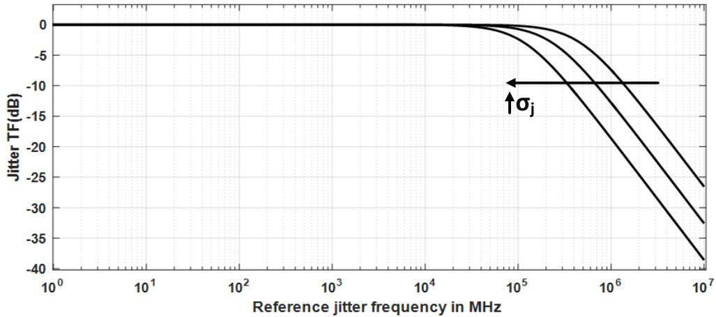
**Figure 3.16** Jitter transfer plot for regular BB DPLL with different input jitter amplitude
