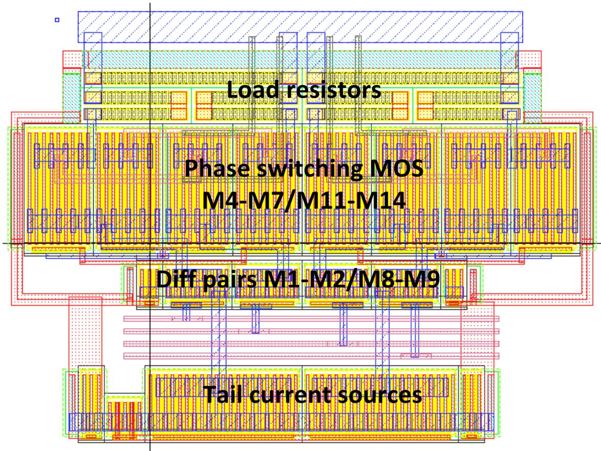
*Figure 4.25 Layout view of phase selection MUX*
