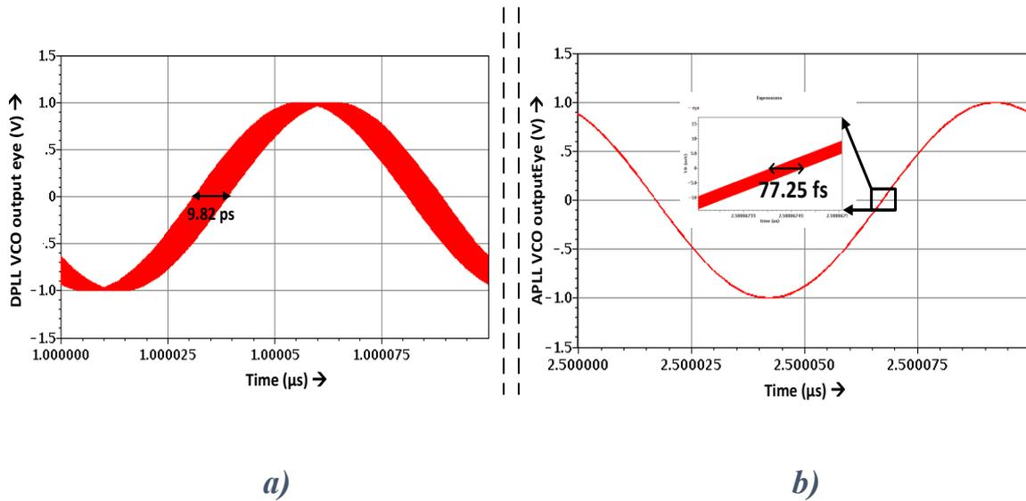
Figure 2.24 PLL output eye diagram: a) DPLL has  $J_{pp}=9.82$  ps b) APLL has  $J_{pp}=77.25$  fs
