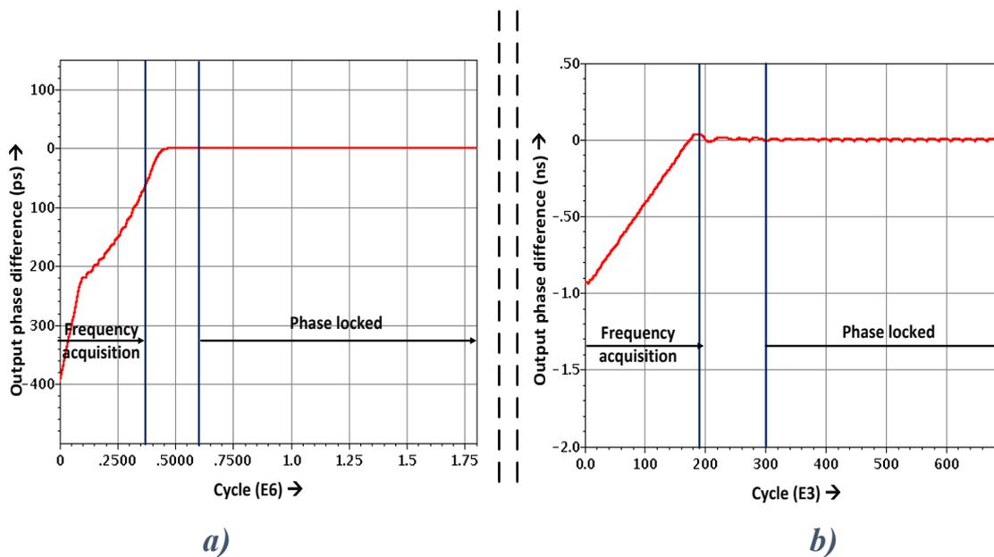
Figure 3.23 Output clock phases of DPLLs (compared with an ideal 10 GHz clock): a) Architecture 2 b) Architecture 1
