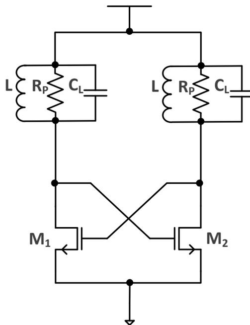
**Figure 4.1** Cross coupled LC oscillator
