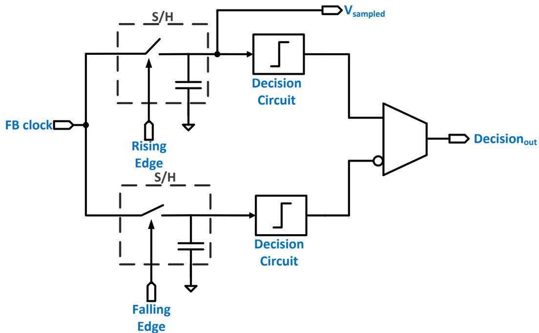
Figure 3.11 Schematic of Improved/dither free Hybrid PD
