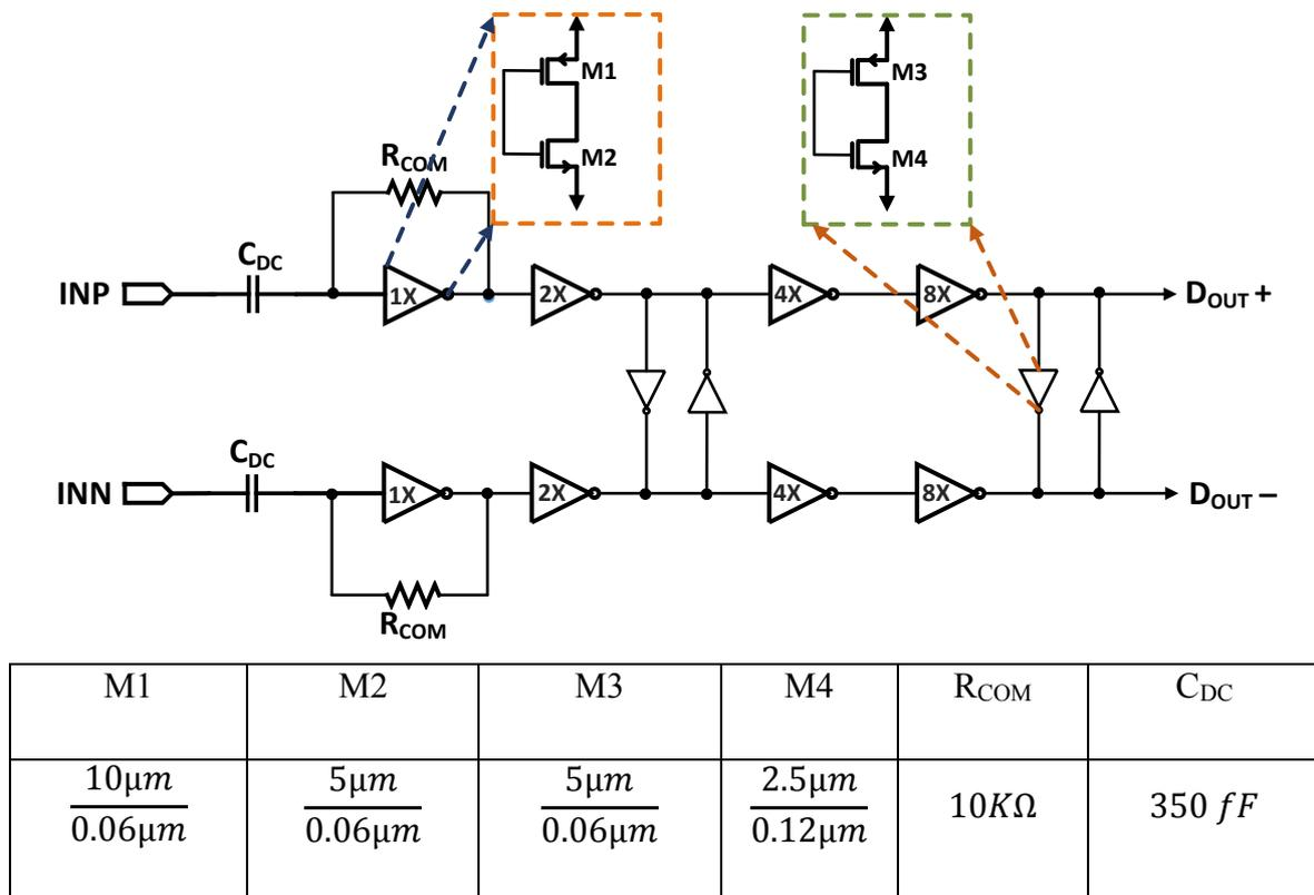
Figure 4.7 Schematic of Decision circuit
