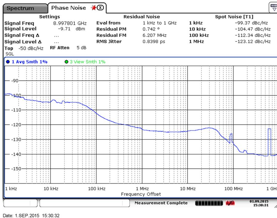
Figure 5.6 Measured phase noise plot for DPLL output clock
