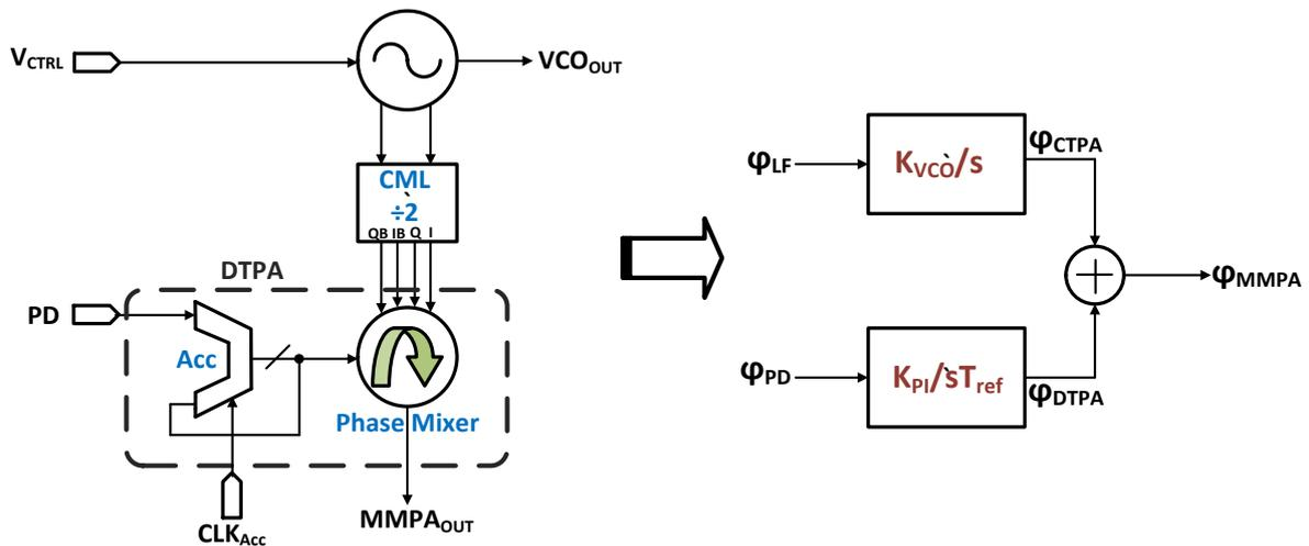
**Figure 3.3 Conceptual block diagram of mixed mode phase accumulator**
