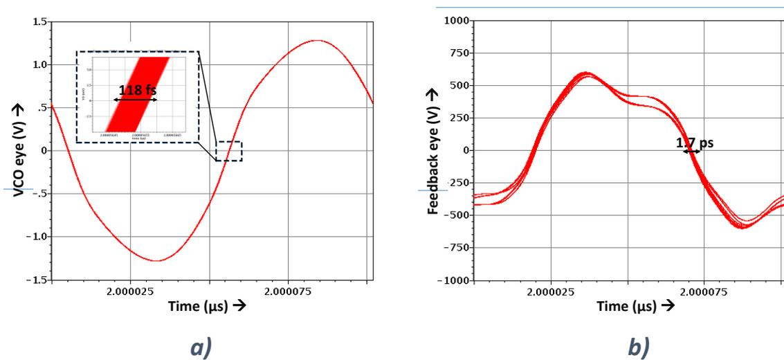
Figure 4.30 Eye diagram of output clock of DPLL: a) VCO b) Feedback
