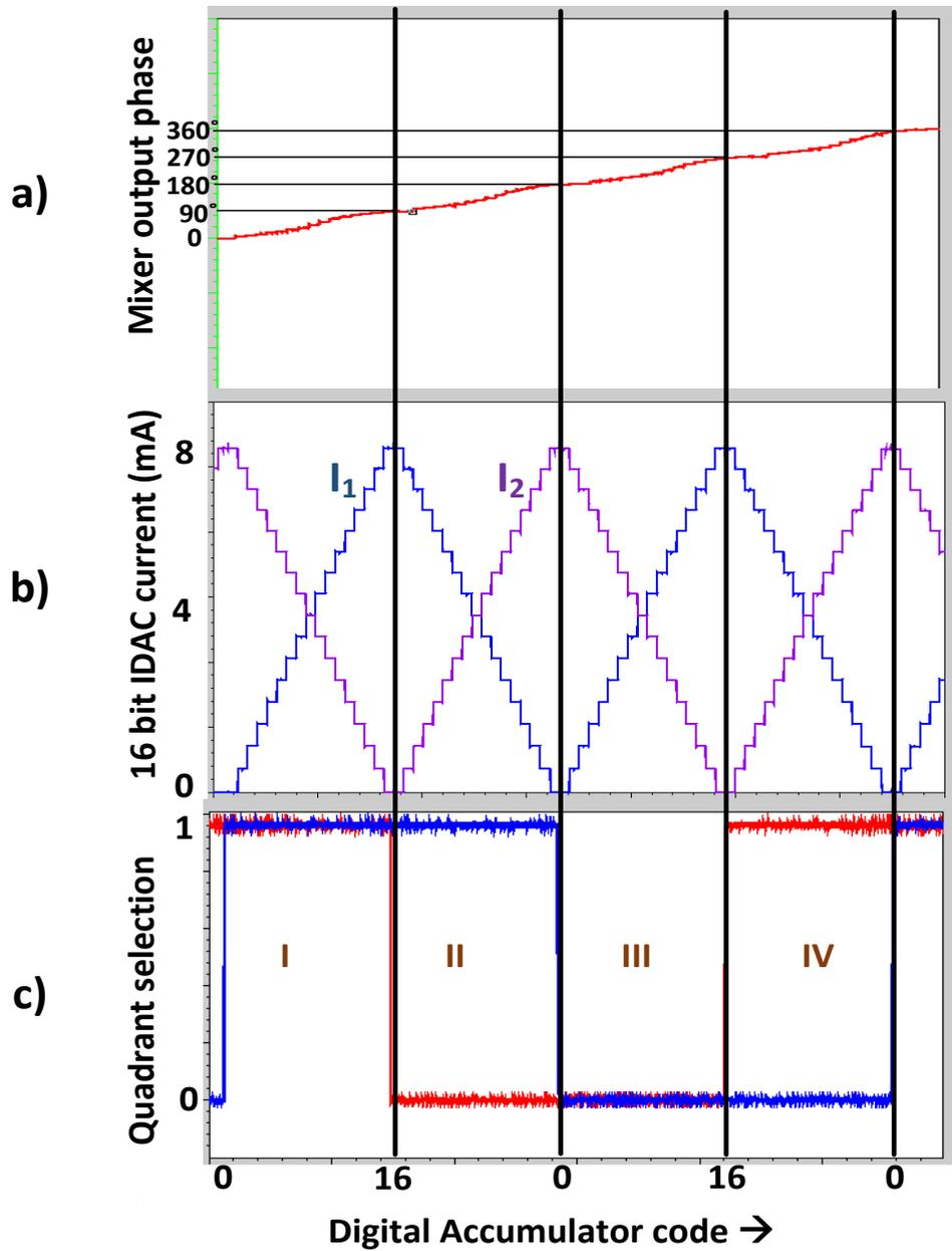
Figure 4.23 Simulated waveforms of discrete time phase accumulator: a) DPC interpolated output phase b) variation of currents in two IDACs according to digital code word c) quadrant selection signals
