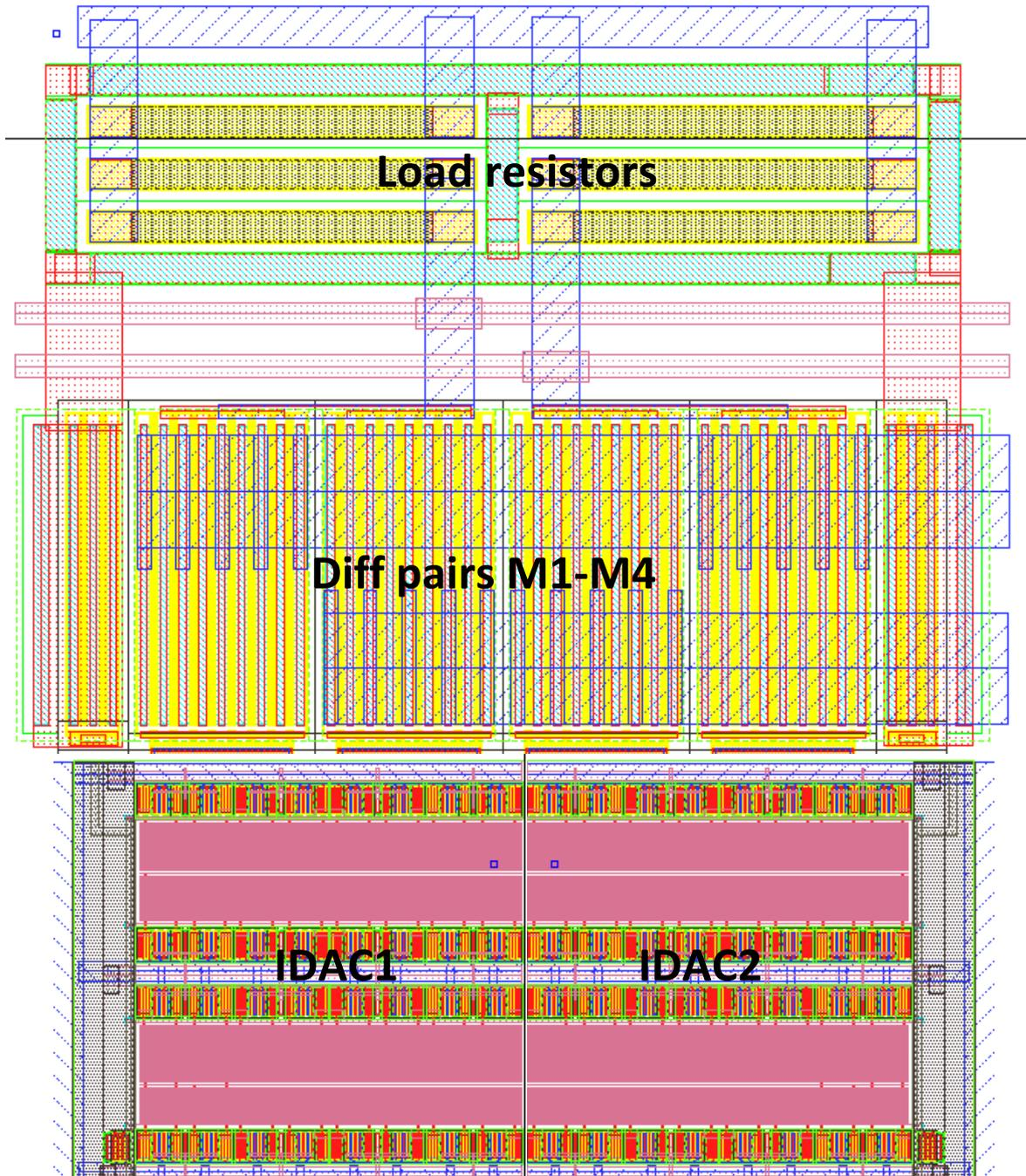
*Figure 4.24 Layout view of analog phase mixer*
