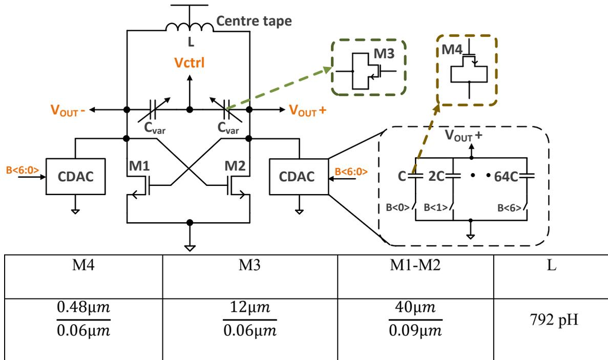
Figure 4.2 Mixed mode VCO for wide frequency tuning range
