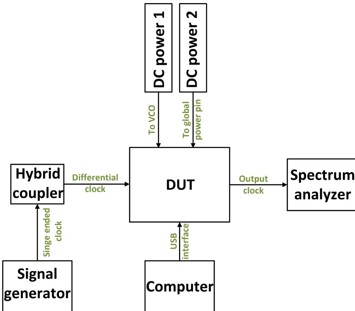
Figure 5.4 Block diagram of external test setup to measure PCB mounted chip
