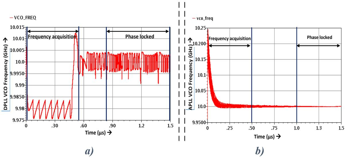
Figure 2.22 Output clock frequency of PLLs : a) DPLL b) APLL
