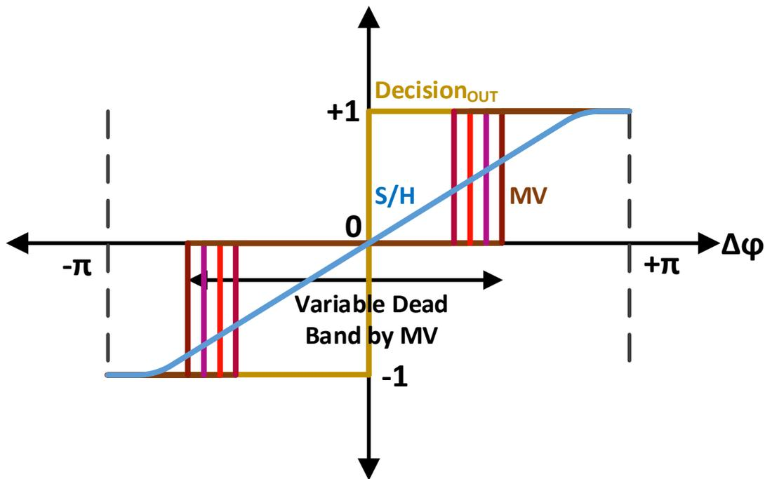
*Figure 3.9 MV creates dead band in decision circuit characteristic*
