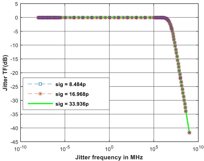
*Figure 3.17 jitter transfer plot for proposed DPLL with different input jitter amplitude*
