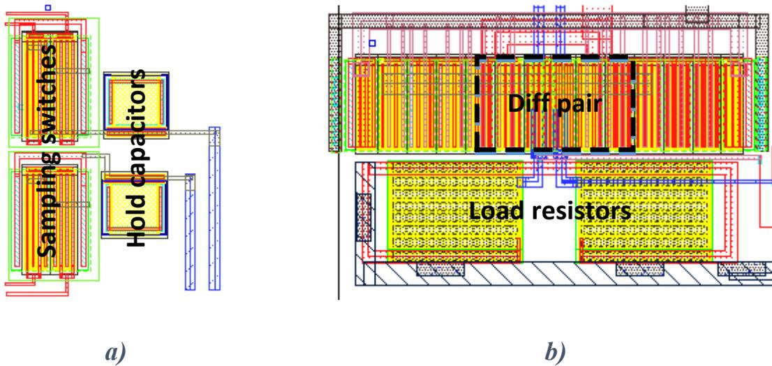
Figure 4.9 Layout views of a) sampler and b) amplifier
