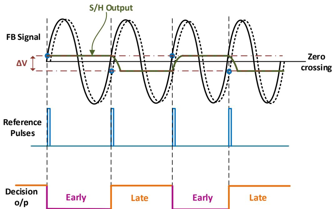
**Figure 3.7** Transient characteristic of hybrid PD
