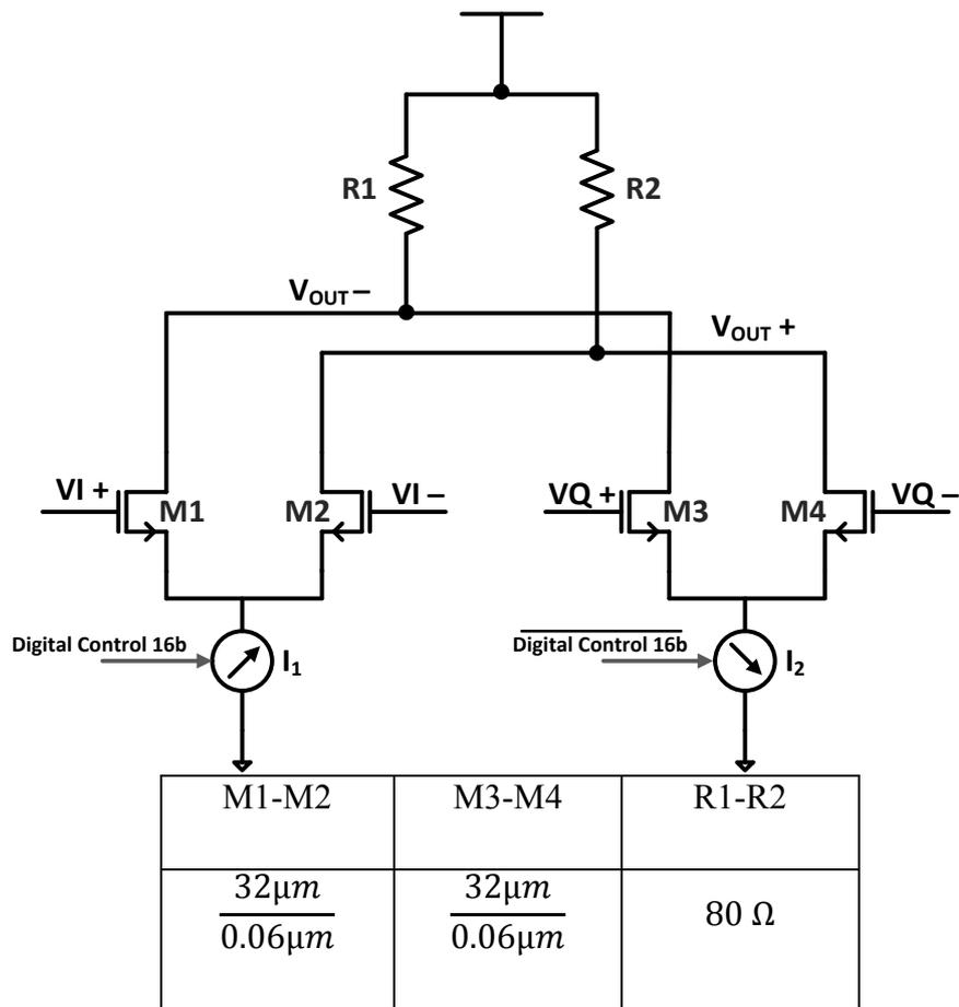
**Figure 4.21 Schematic of analog phase mixer**
