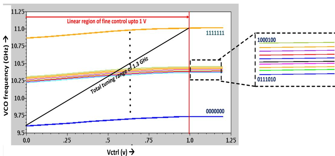
**Figure 4.3 Simulated transfer curve of mixed mode VCO**
