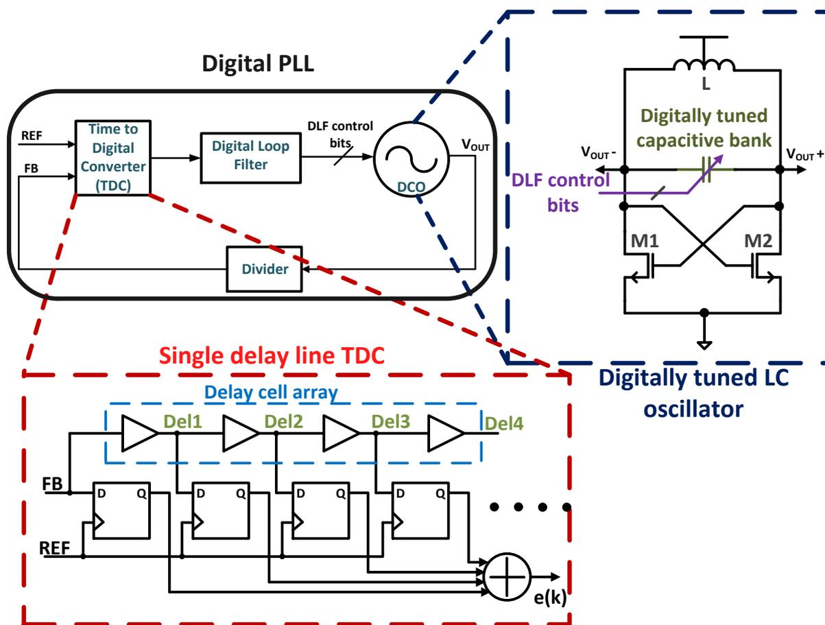
Figure 2.25 Digital PLL architecture with conventional delay line TDC and digitally controlled LC tank
