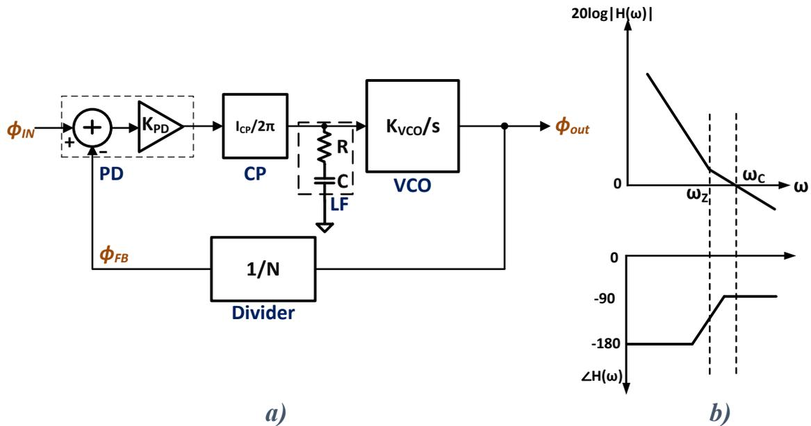
**Figure 2.8 Modelling of Type II 2nd order PLL: a) Complete PLL in s domain b) Open loop frequency response**
