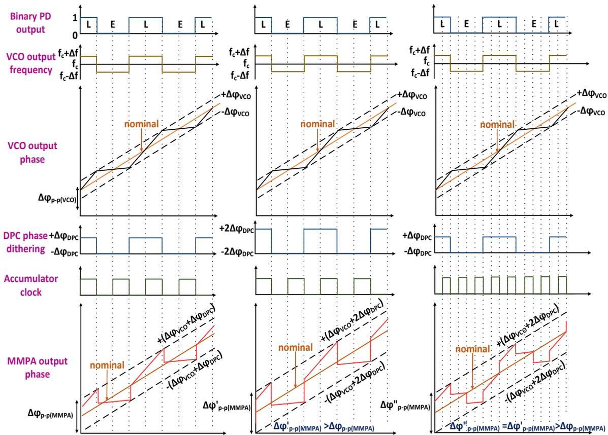
a) MMPA output phase is combination of that of VCO and DPC. Accumulator is updated in both rising and falling edges of clock
