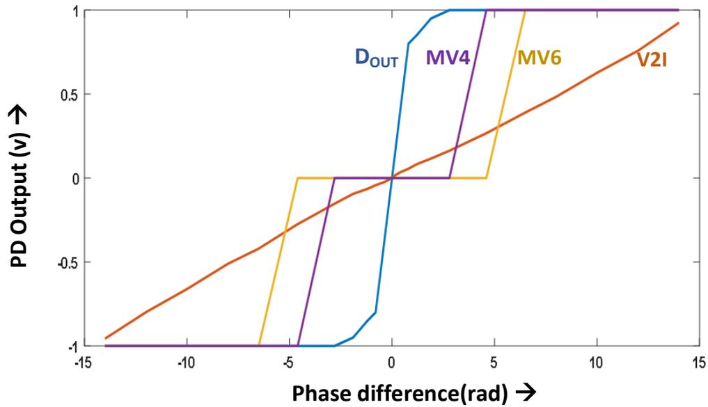
Figure 4.8 Characteristic of Hybrid PD: it includes decision output, V2I current (normalized), and MV output with programmable  $D$
