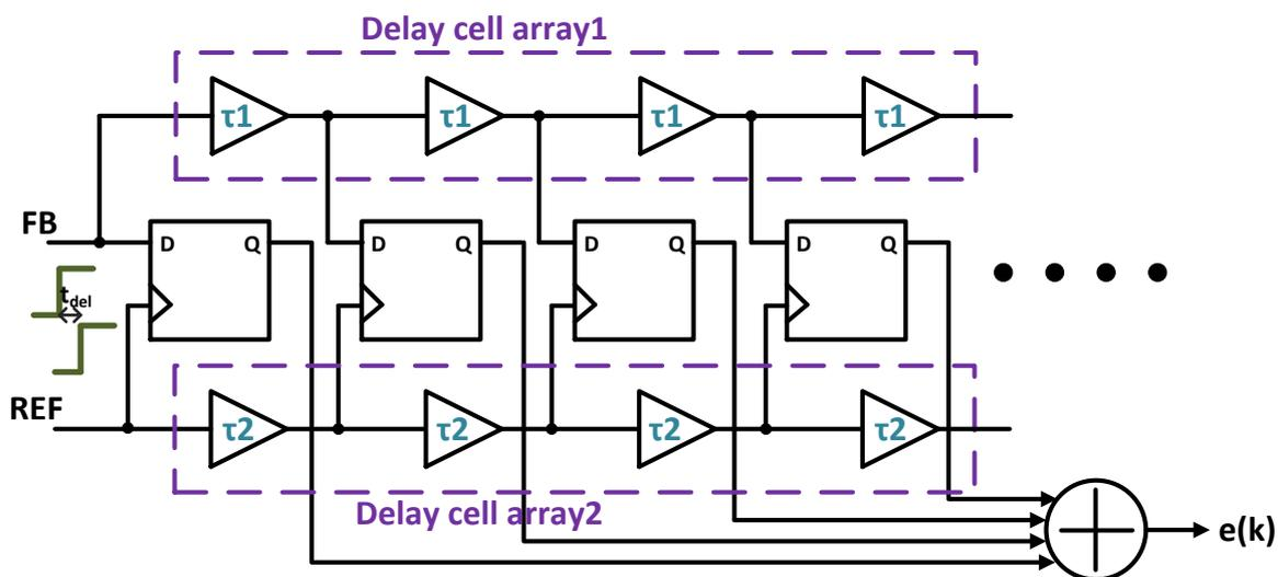
Figure 2.29 TDC architecture based on Vernier delay line principle
