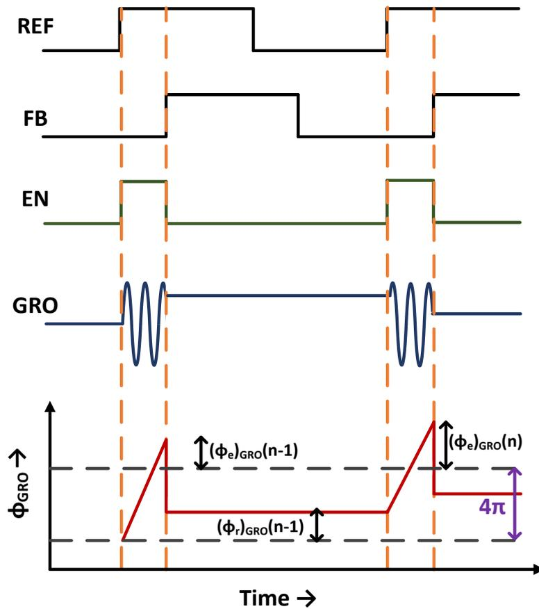
Figure 2.32 Basic timing diagram of GRO based TDC
