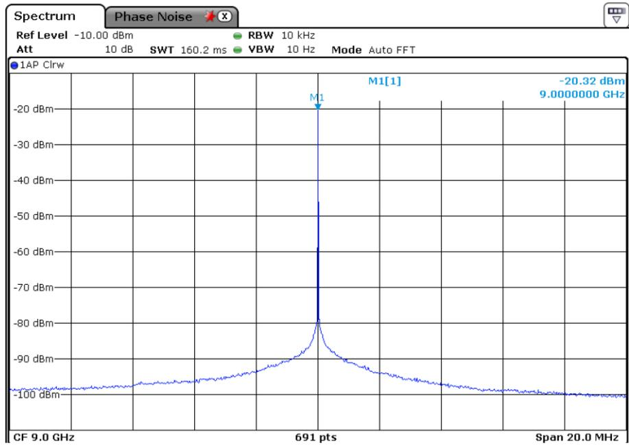
Figure 5.6 Measured frequency spectrum of locked DPLL output clock
