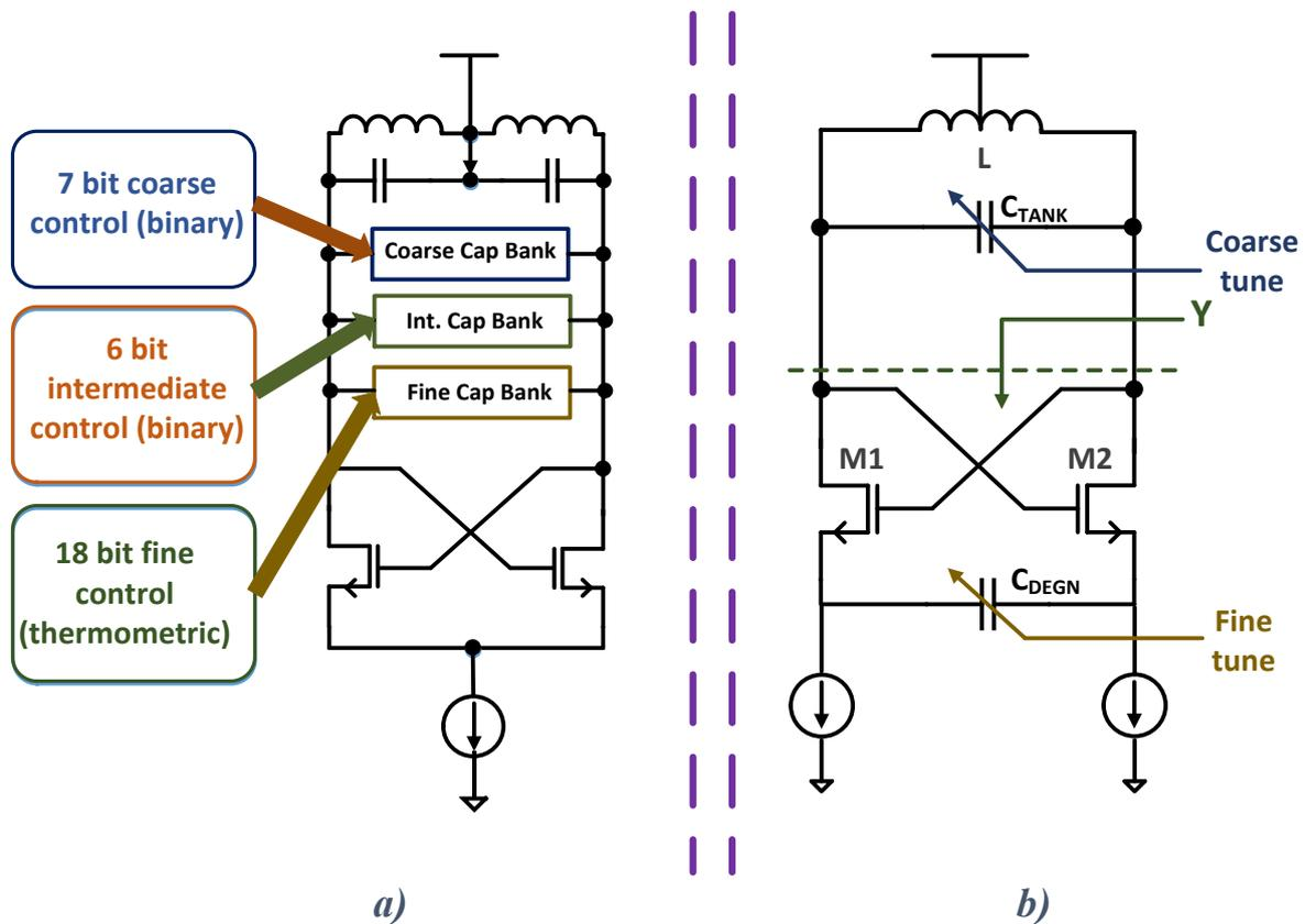
Figure 2.33 Circuit diagram of high resolution LC VCO used in a) [18] b) [19]
