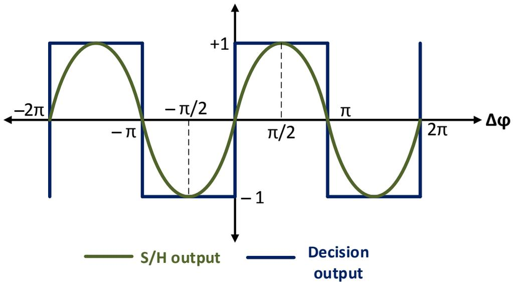
Figure 3.6 Characteristic of Hybrid PD
