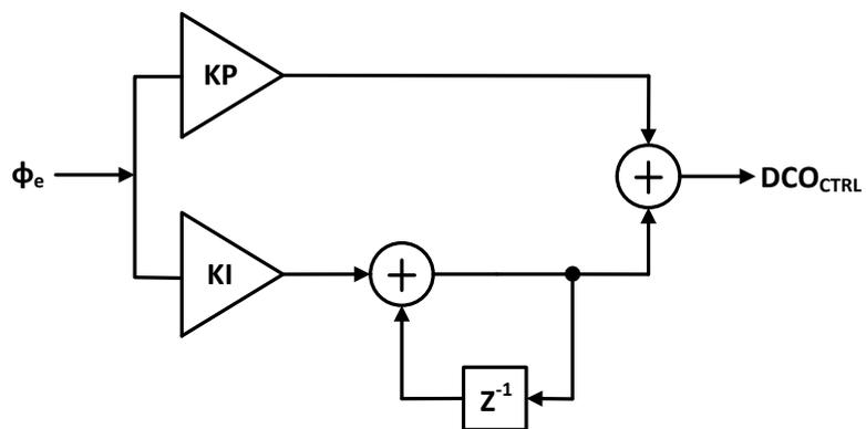
Figure 2.14 Digital loop filter model in z domain
