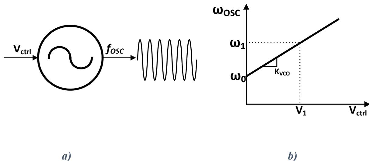
Figure 2.3 Functionality of VCO: a) Functional block diagram b) Transfer characteristic
