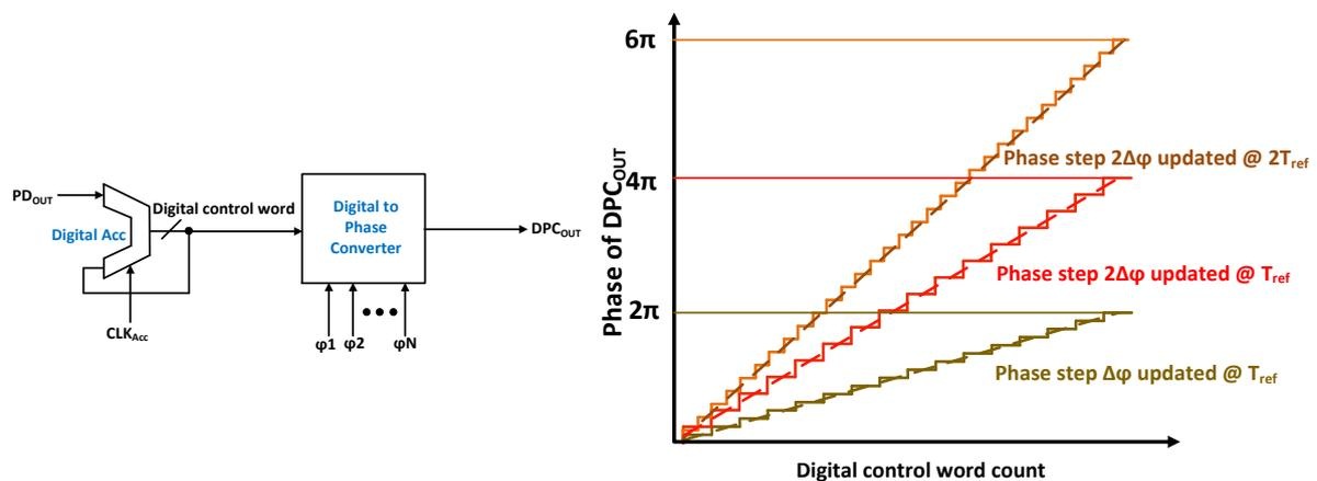
**Figure 3.2** Block diagram of discrete time phase accumulator with its characteristic
