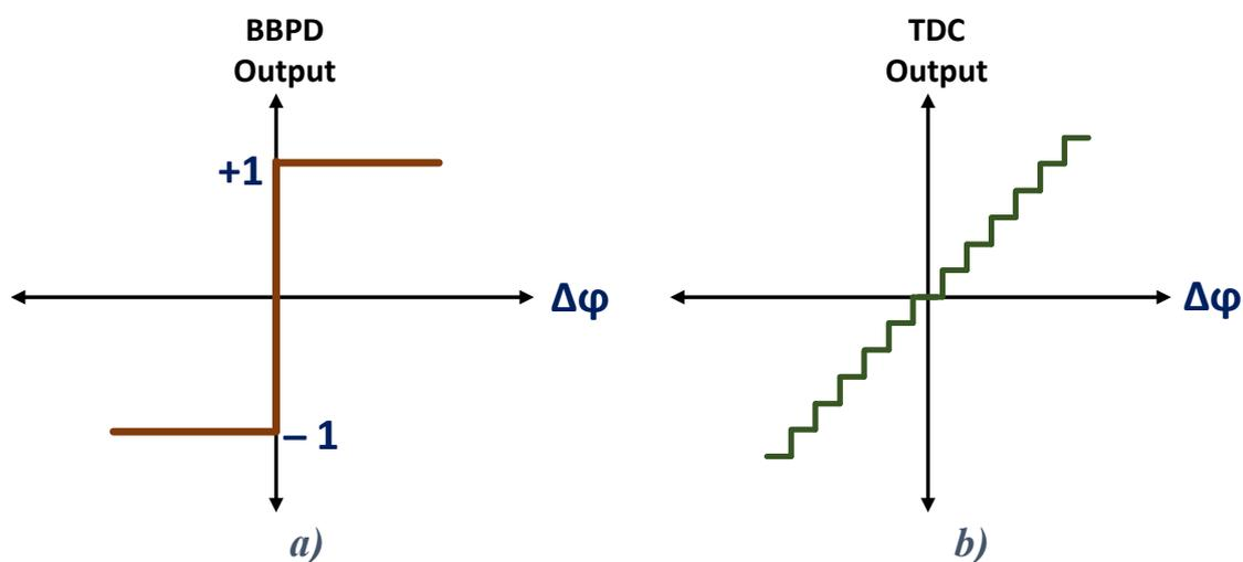
**Figure 2.28** Phase detector transfer characteristic: a) BBPD (only two quantization levels) b) TDC (several quantization levels)
