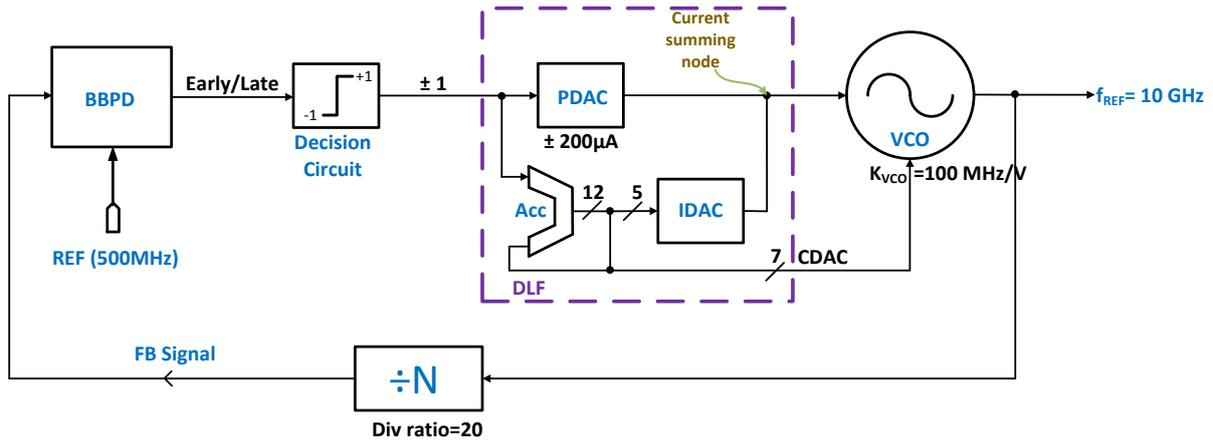
Figure 2.19 DPLL circuit simulated in Cadence AMS environment
