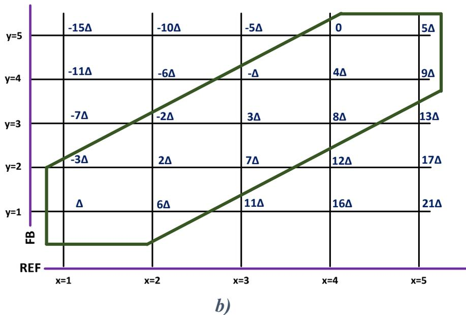
Figure 2.30 Quantization levels: a) linear Vernier TDC b) 2D Vernier TDC [14]
