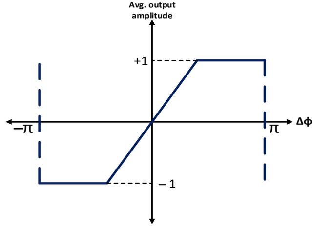
**Figure 2.12 Characteristic of BBPD modified by practical limitation**
