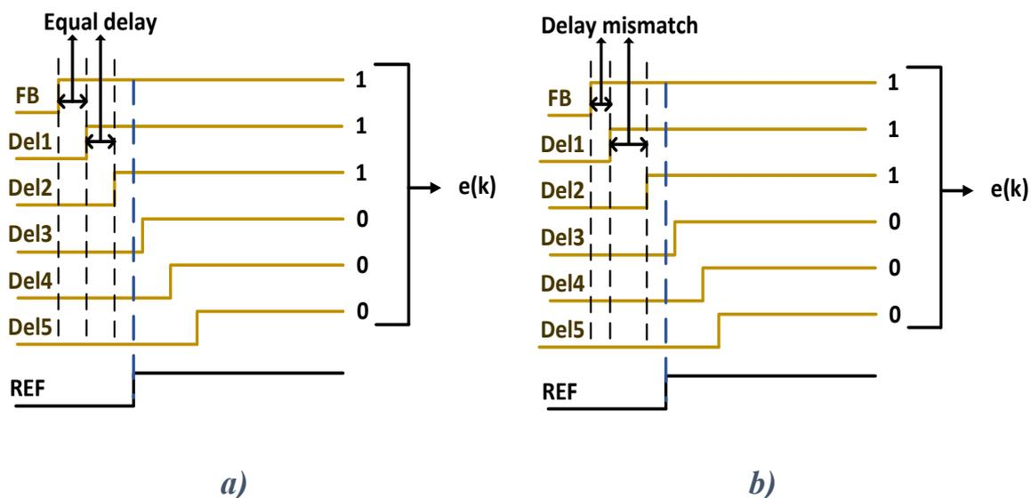
**Figure 2.26** Process of time to digital conversion: *a) ideal case (no mismatch) b) practical case (presence of delay mismatch)*
