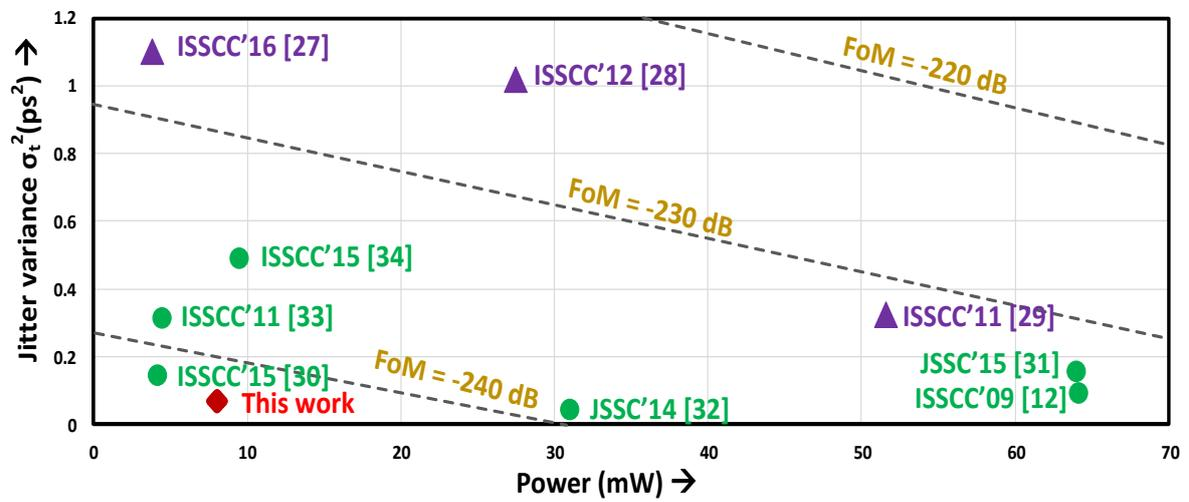
Figure 5.7 FoM comparison with the recently reported PLLs (LC tank based DPLL are in green)
