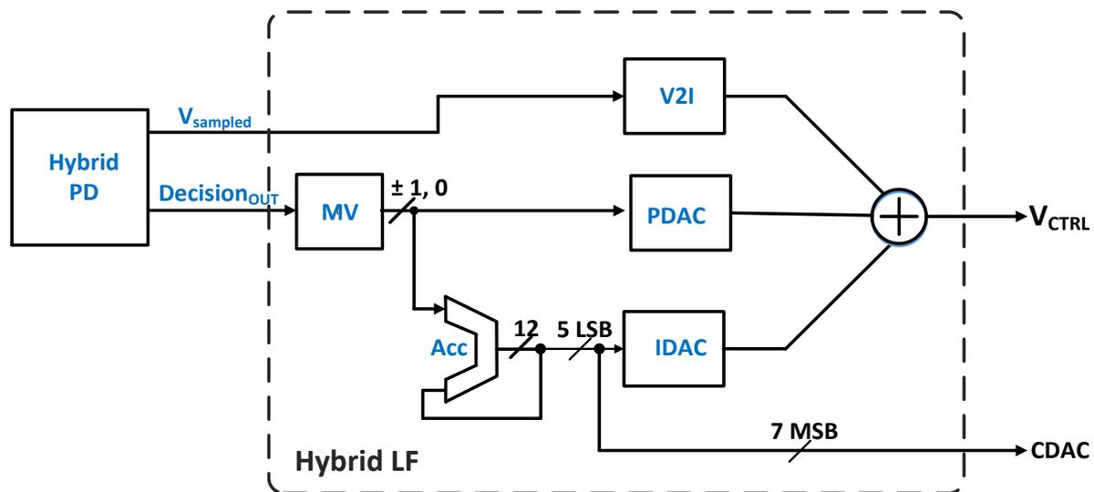
**Figure 3.8 Schematic of Hybrid LF**
