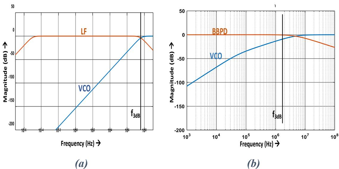
Figure 2.18 Noise transfer functions of PLLs: a) APLL b) DPLL
