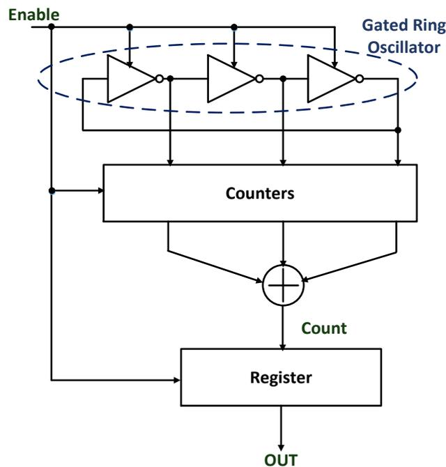
Figure 2.31 Structure of GRO based TDC [17]
