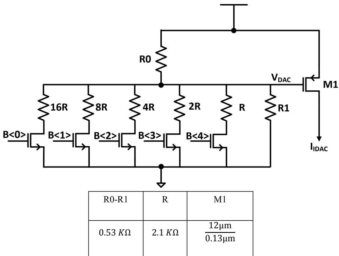
**Figure 4.14 Schematic of 5 bit binary weighted resistive IDAC**
