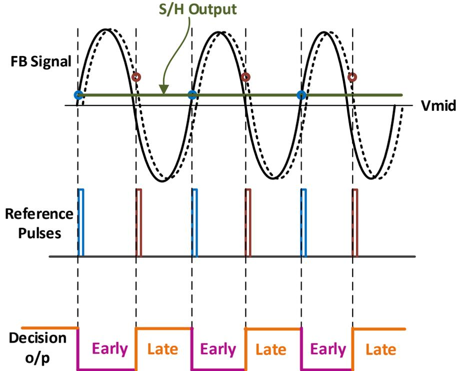
Figure 3.13 Transient characteristic of ditherless Hybrid Phase Detector
