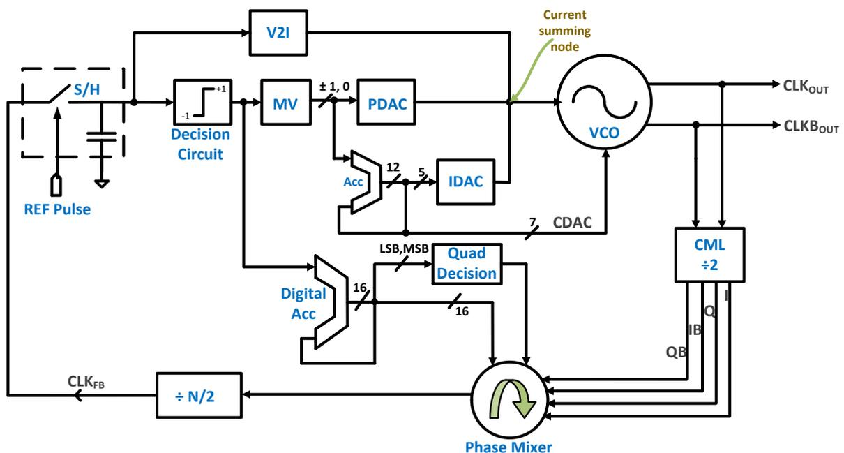
**Figure 3.10 Architecture 1: DPLL based on Hybrid PD and mixed mode phase accumulator**
