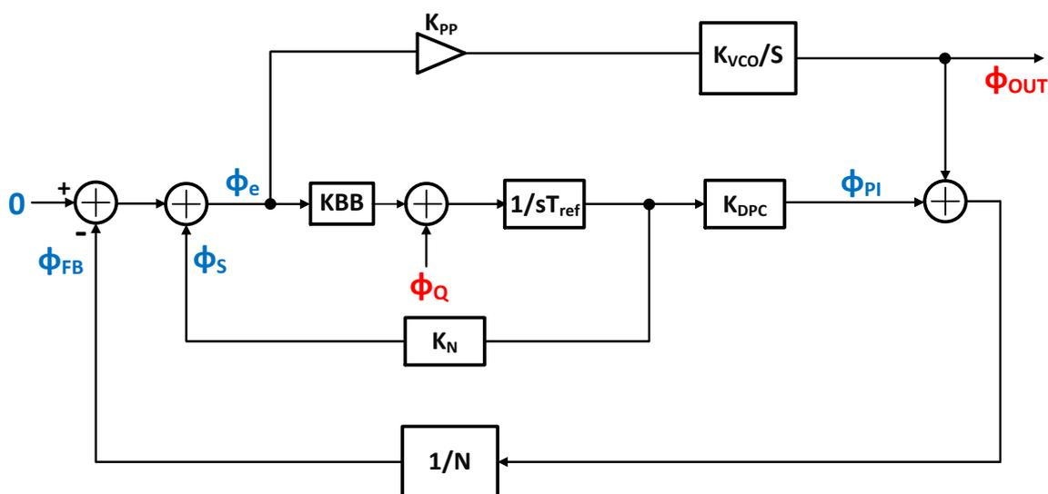
**Figure 3.16 Proposed DPLL s domain model for calculation of quantization noise transfer function**
