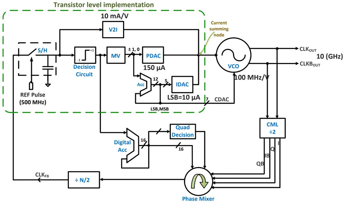
Figure 3.18 DPLL Architecture 1: designed with Hybrid PD and mixed mode phase accumulator
