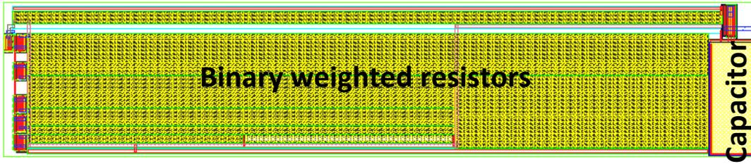
Figure 4.15 Layout of 5 bit binary resistive IDAC
