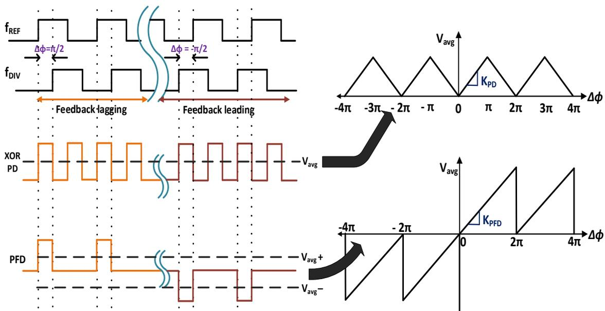
**Figure 2.5** Timing diagram of XOR PD and PFD along with their input-output characteristic
