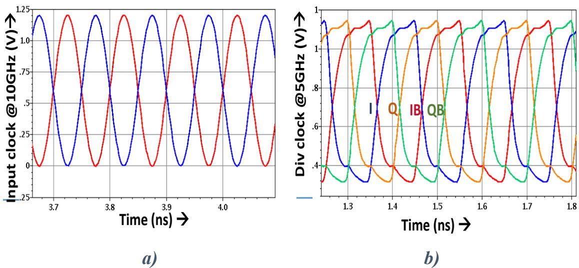
**Figure 4.19** Simulation result for CML divider a) 10 GHz complementary input b) 5GHz quadrature output
