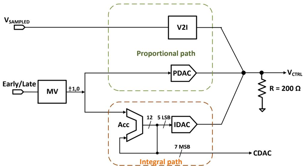
Figure 4.11 Schematic of Hybrid LF
