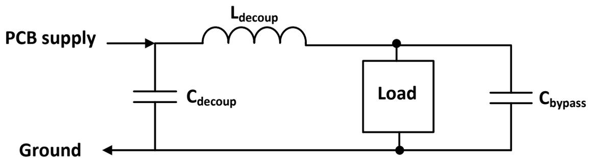
*Figure 5.3 Supply noise filtering technique used in board design*
