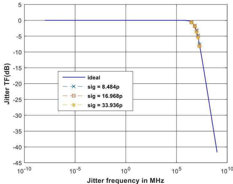
**Figure 4.31 Simulated jitter transfer function of proposed DPLL**
