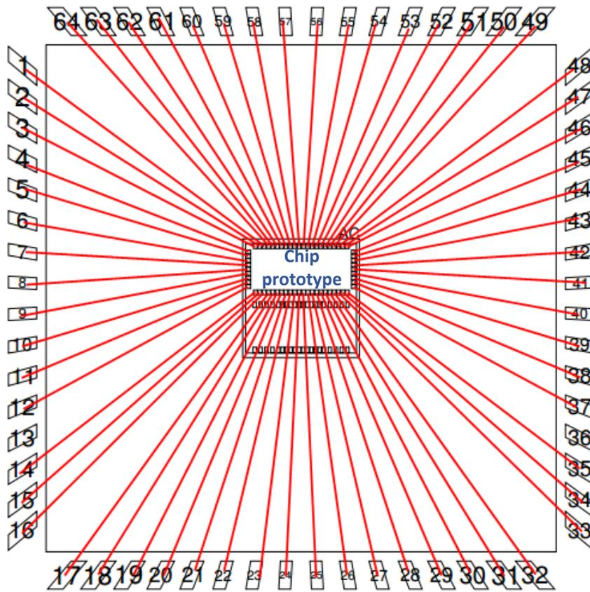
Figure 5.1 OCP\_QFN\_9X9\_64A packaging of chip by MOSIS
