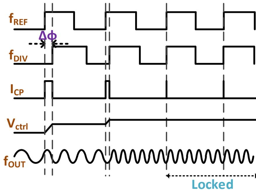
Figure 2.2 PLL locking mechanism
