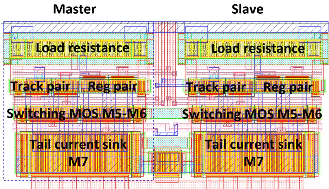
*Figure 4.20 Layout view of CML based DFF*
