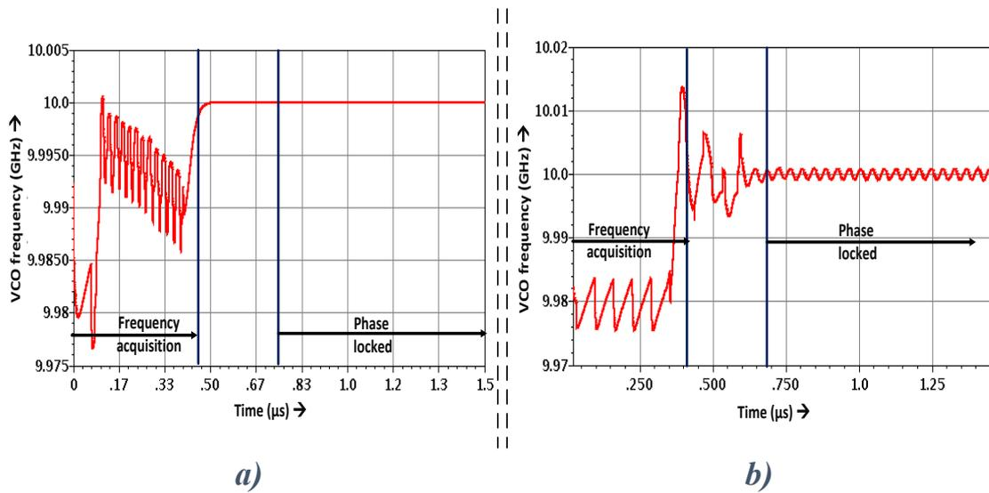
Figure 3.22 Output clock frequencies of DPLLs: a) Architecture 2 b) Architecture 1
