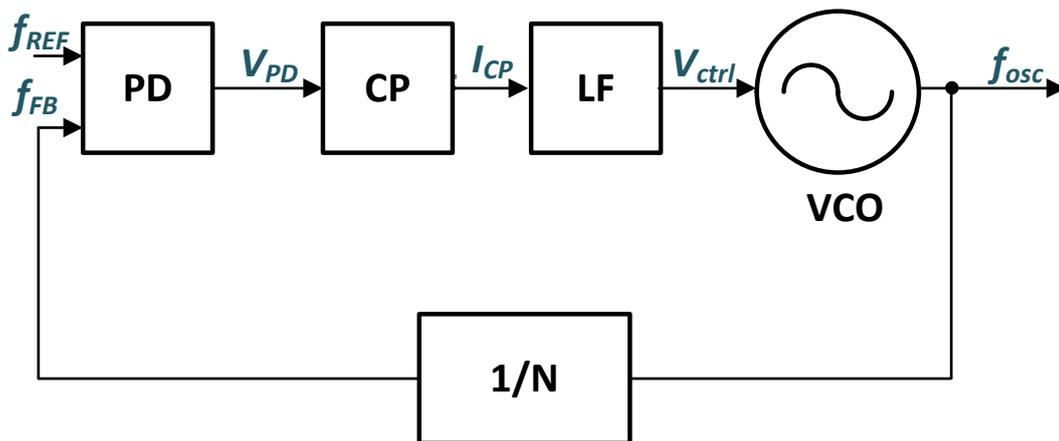
Figure 2.1 Basic Block Diagram of Analog PLL
