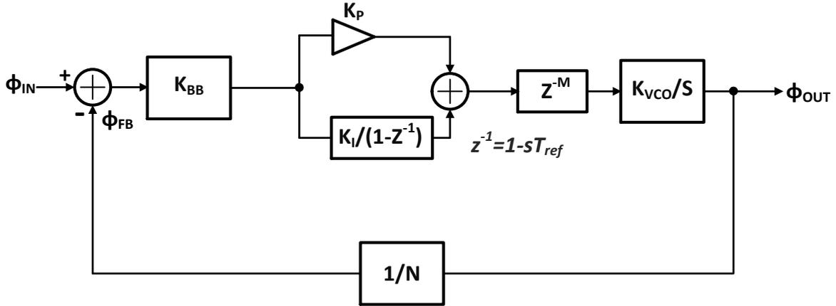
Figure 2.15 Linearized model of regular BB PLL
