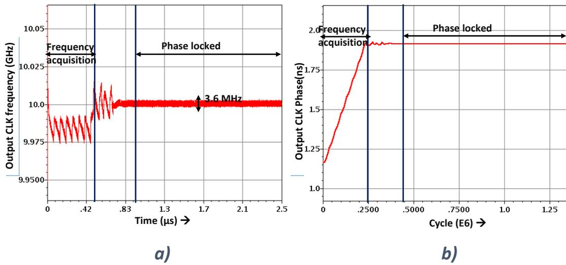
Figure 4.29 Output clock of DPLL: a) frequency plot b) Phase plot
