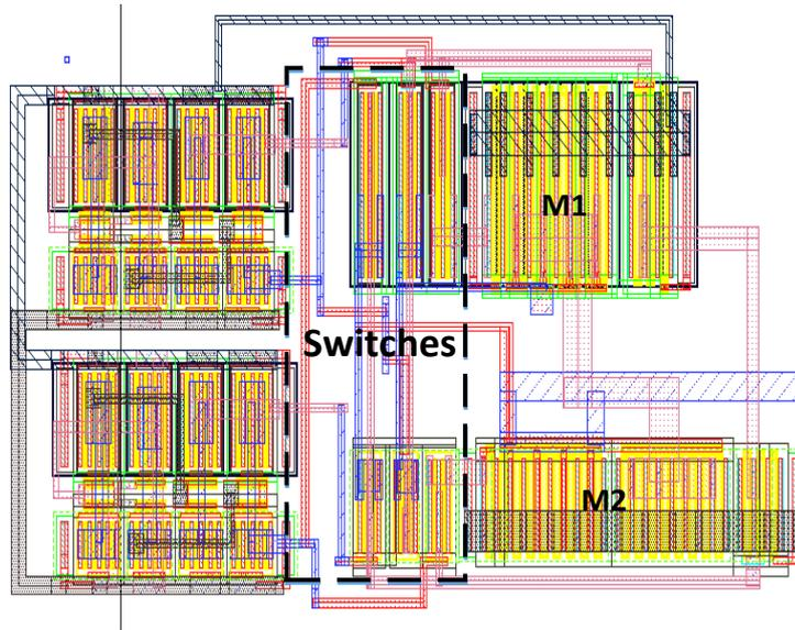
**Figure 4.13** Layout view of 2 bit PDAC
