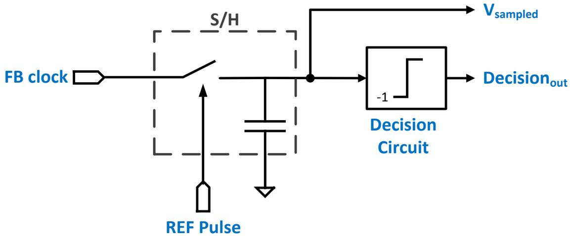
Figure 3.5 Schematic of proposed hybrid PD
