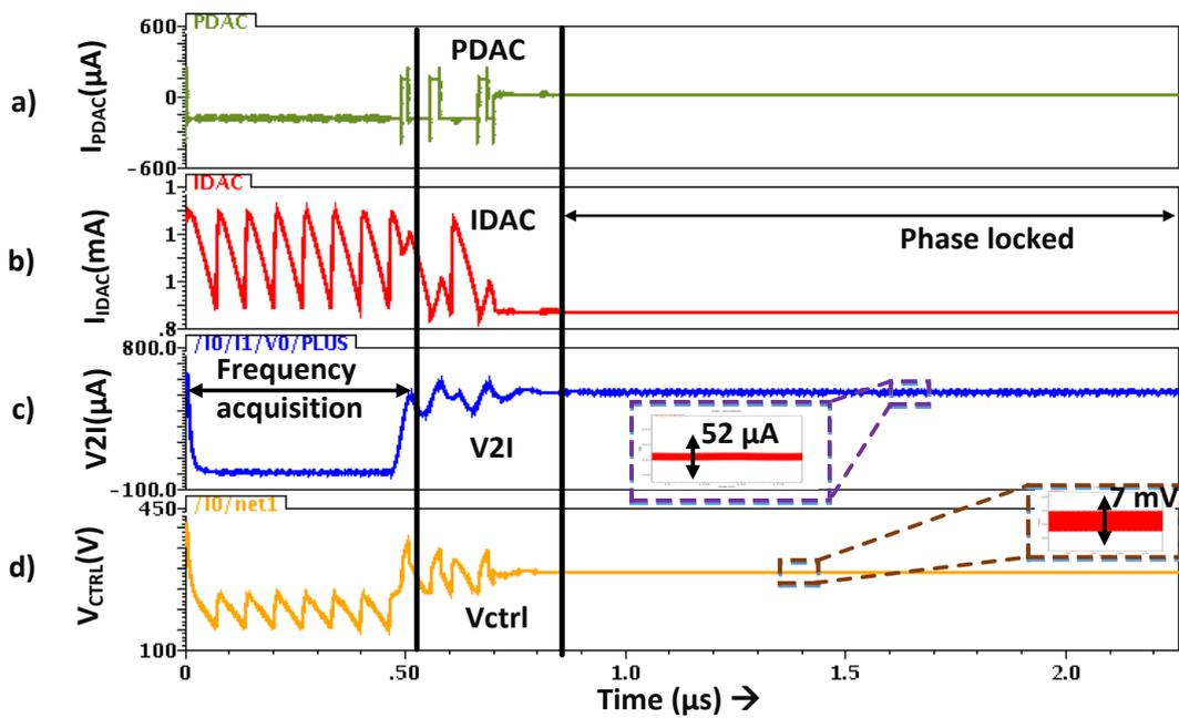
Figure 4.28 Control nodes of DPLL: a) PDAC b) IDAC c) V2I c) Vctrl
