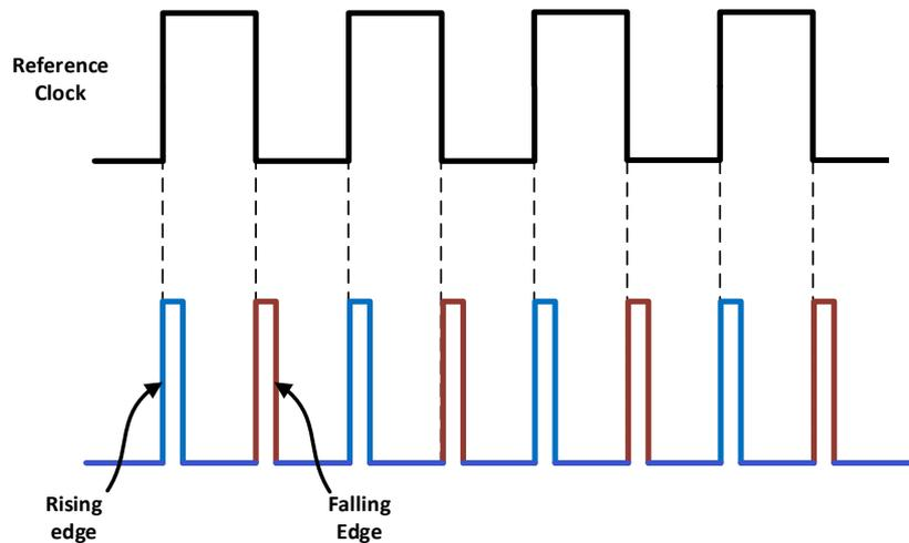
**Figure 3.12 Dual edge pulse generation**
