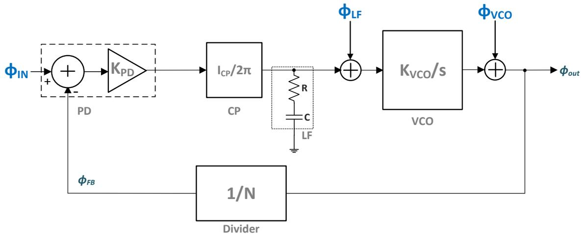
Figure 2.16 Various noise sources of analog PLL
