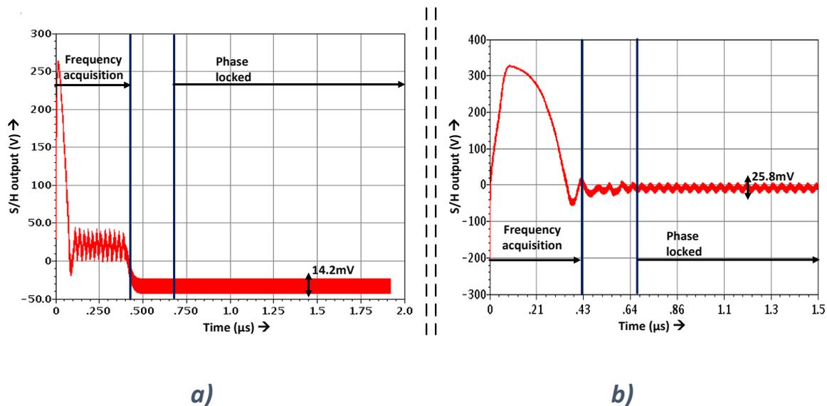
**Figure 3.20 Output voltage of S/H: a) Architecture 2 has less dithering than b) Architecture 1**
