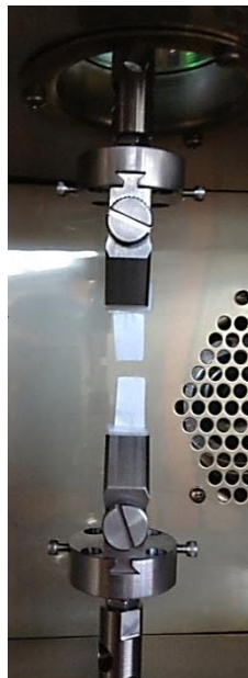
Figure 12. Tensile test specimen that broke in the gauge section center during tensile testing.
