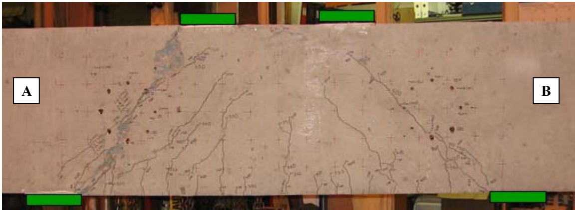
Figure 4-50 Specimen NS1-4 after failure
