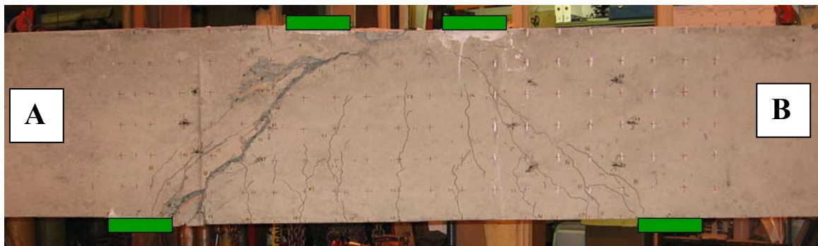
Figure 4-38 Specimen MW1-2 after failure
