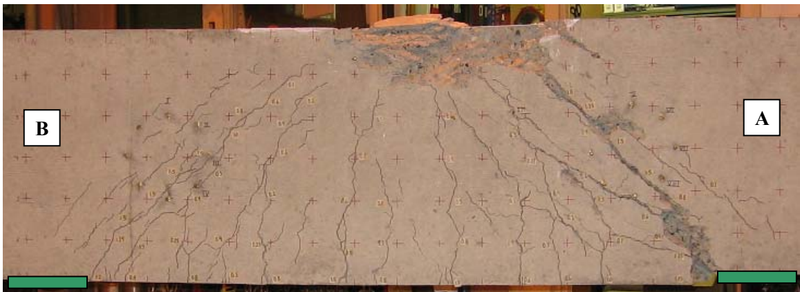
Figure 4-8 Specimen MS1-2 after failure
