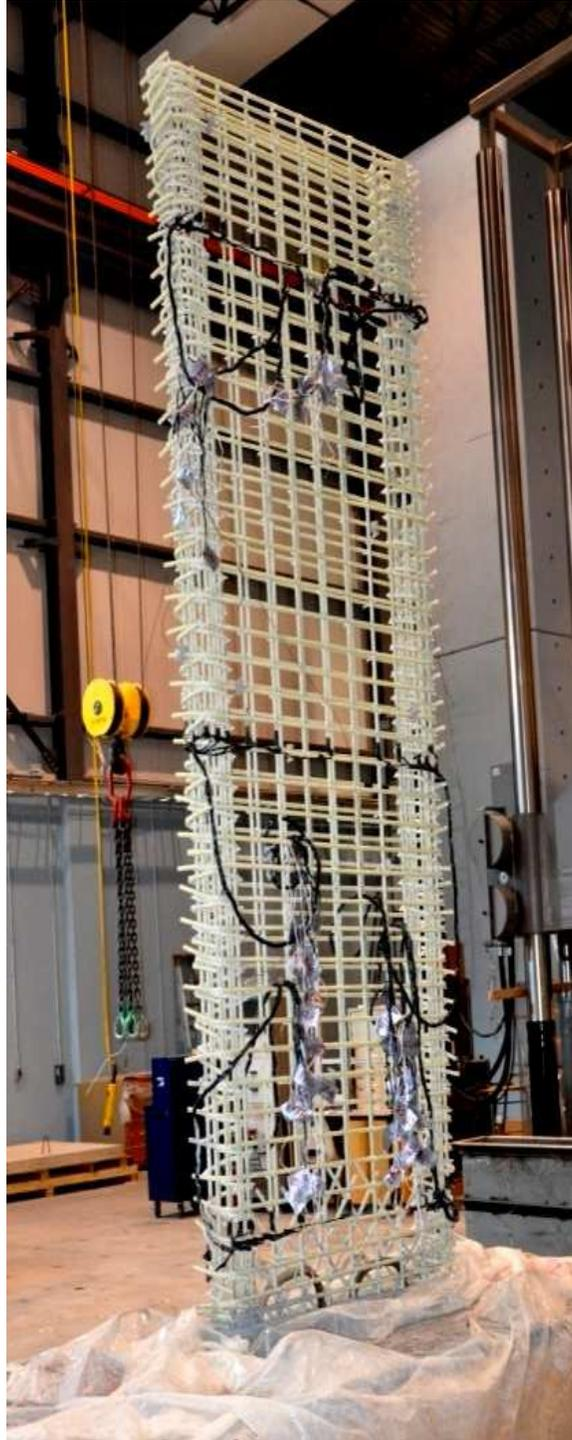
Figure 3. 4: Reinforcement cage of G12 (Mohamed et al. 2013)
