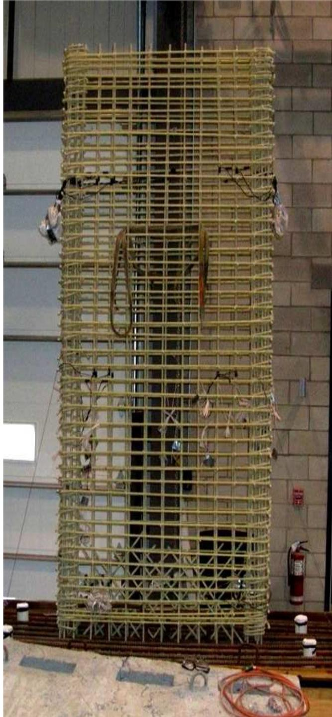
**Figure 3. 5: Reinforcement cage of G15 (Mohamed et al. 2013)**
