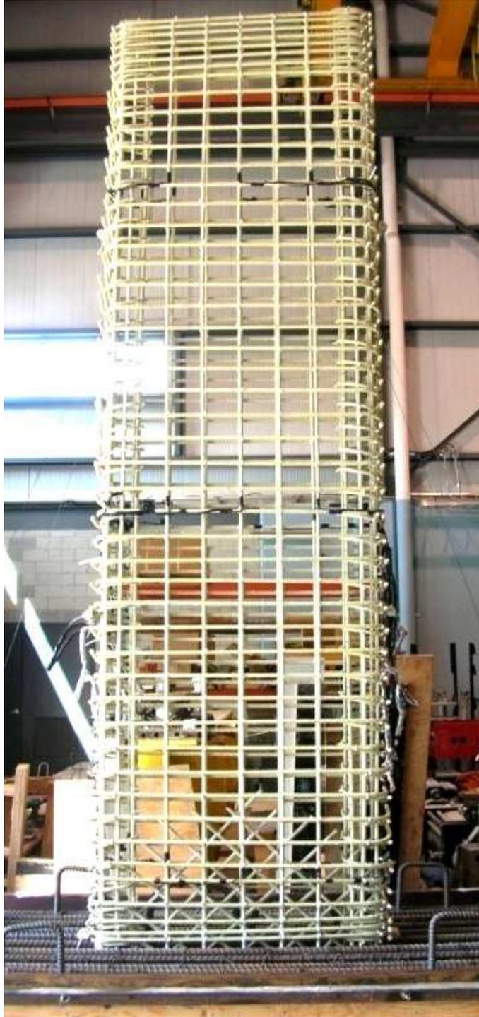
**Figure 3. 3: Reinforcement cage of G10 (Mohamed et al. 2013)**
