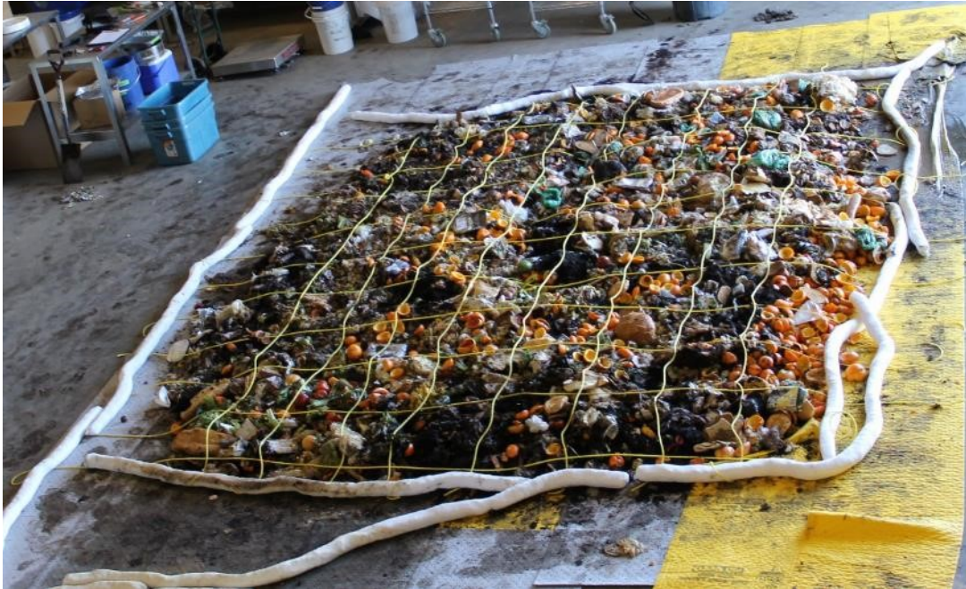
Figure C.4. Unprocessed source separated organics sampling steps (step3.b, making grids).
