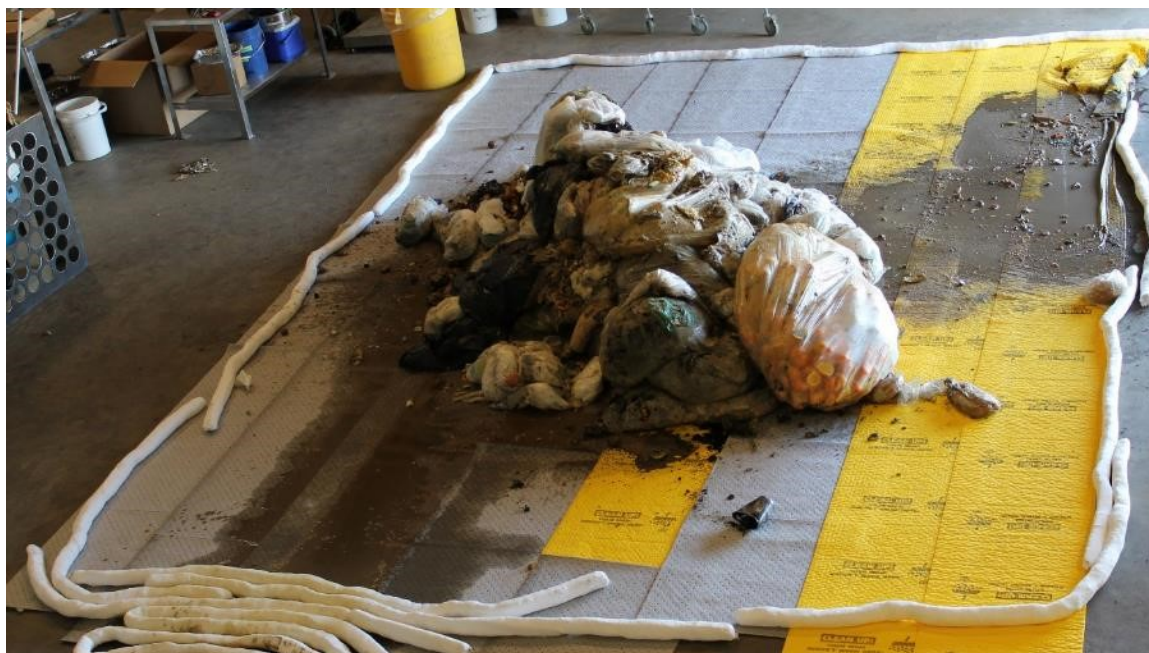
Figure C.1. Unprocessed source separated organics sampling steps (step1, debagging).
