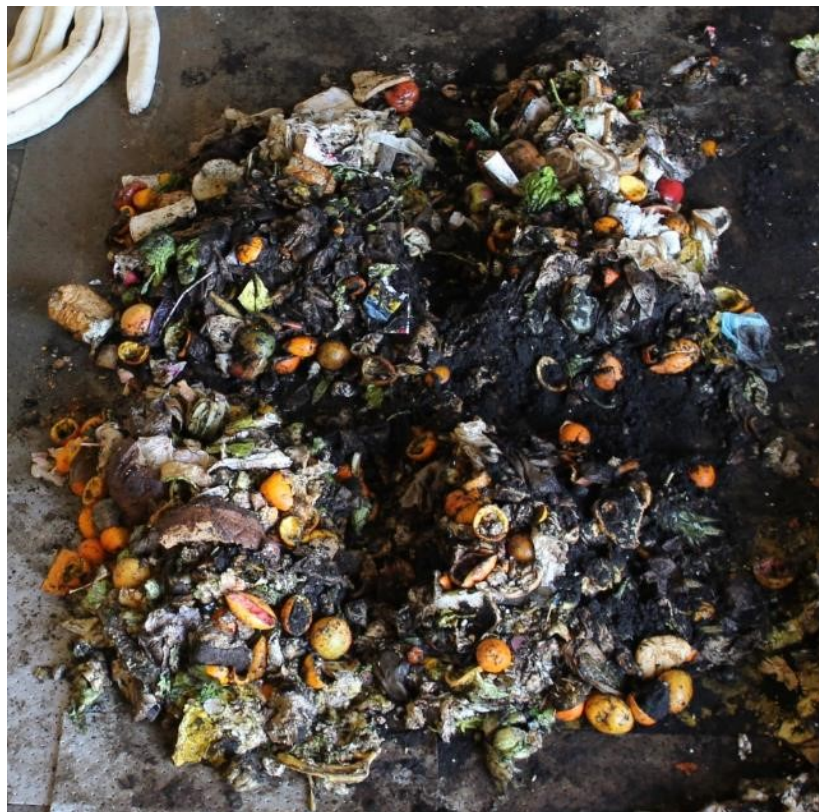
Figure C.5. Unprocessed source separated organics sampling steps (step4, quartering).
