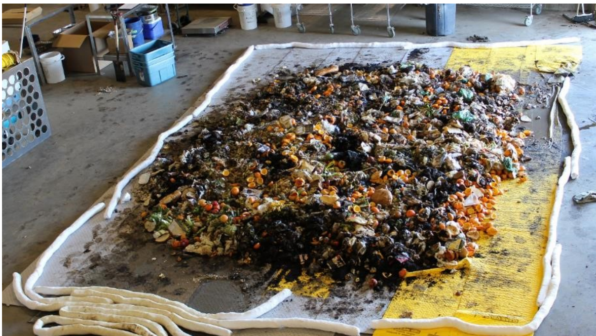
Figure C.2. Unprocessed source separated organics sampling steps (step2, distribution).
