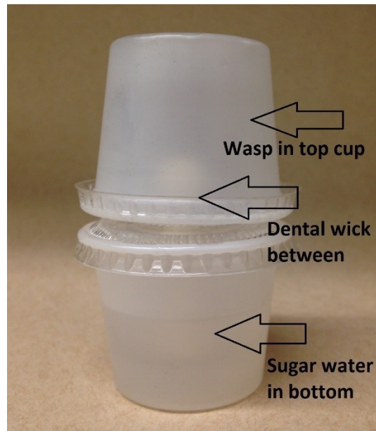
Figure 3.1 Feeder for sucrose solution feeding experiments. 36 ml plastic cups joined by a 3cm cotton wick.
