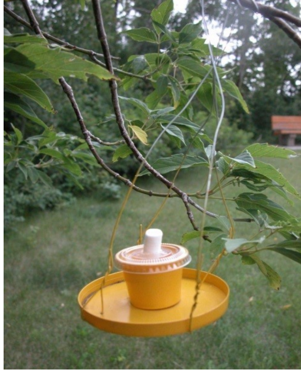
Figure 3.6 Feeders providing sucrose solutions used in Experiment 5. Feeders consisted of a 10 cm diameter plastic Petri Plate with the 36 ml cup attached to the centre. Access to the sucrose solution in the cup was through a 3 cm dental wick attached to the cup lid. The entire feeding apparatus was painted yellow and suspended within the canopy of ash trees with wires.
