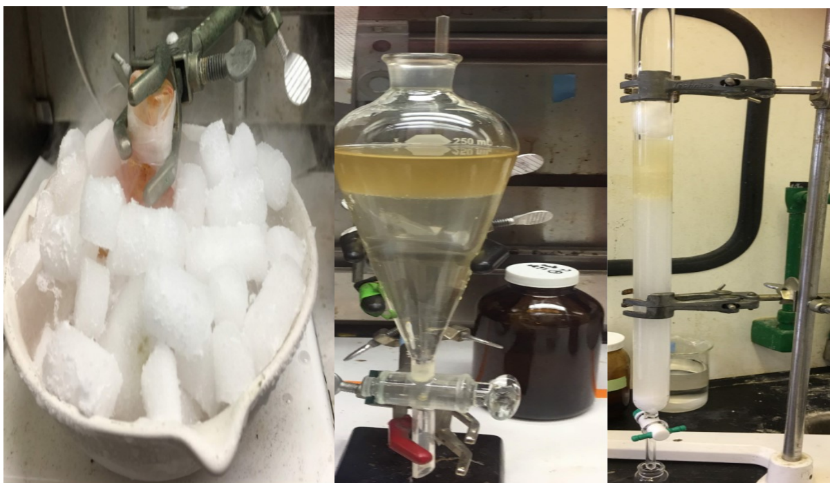
Figure C. 4. Reaction set ups for the test runs, from left to right: -Reaction mixture at low temperatures using dry ice in the absence of ice as the coolant -Liquid-liquid phase separation of immiscible organic-inorganic mixtures to define the side-products. -Column setup for liquid-solid chromatography for product purification
