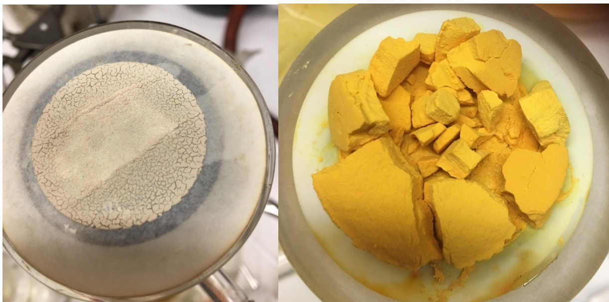
Figure C. 6. Residue on filter papers; after water washing of reactions products (right), after drying mixture with Na_2SO_4 (left)
