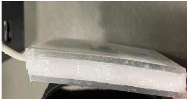
**Figure 5. Side view of the force sensors. Two plexiglass sheets, sealed with regular caulking silicon, contained the two sensors inside.**
