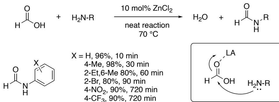
Scheme 1-9: Selected examples of formamides obtained with ZnCl<sub>2</sub> and proposed intermediate.
