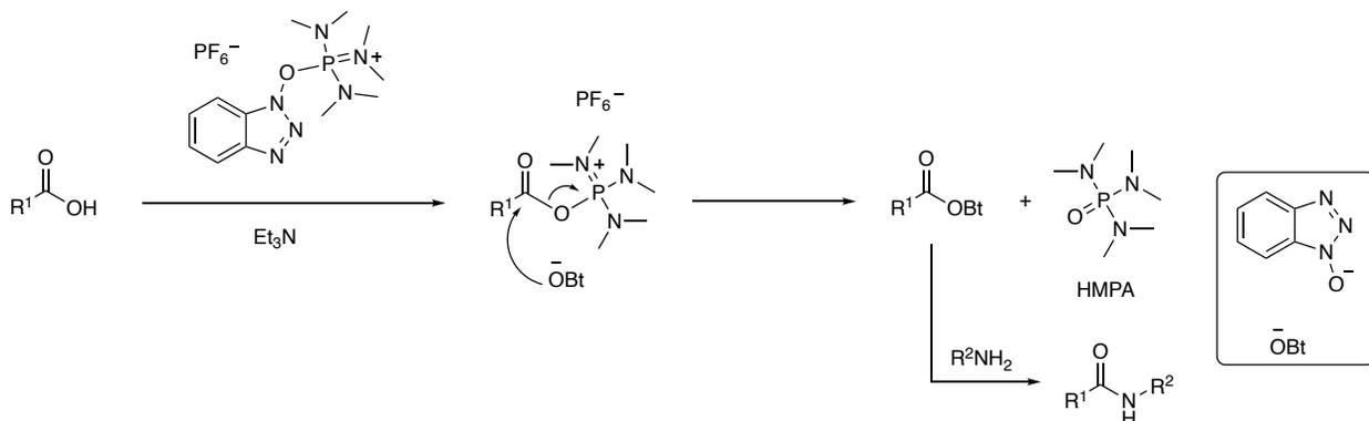
Scheme 1-7: Mechanism of BOP mediated amidation reaction.
