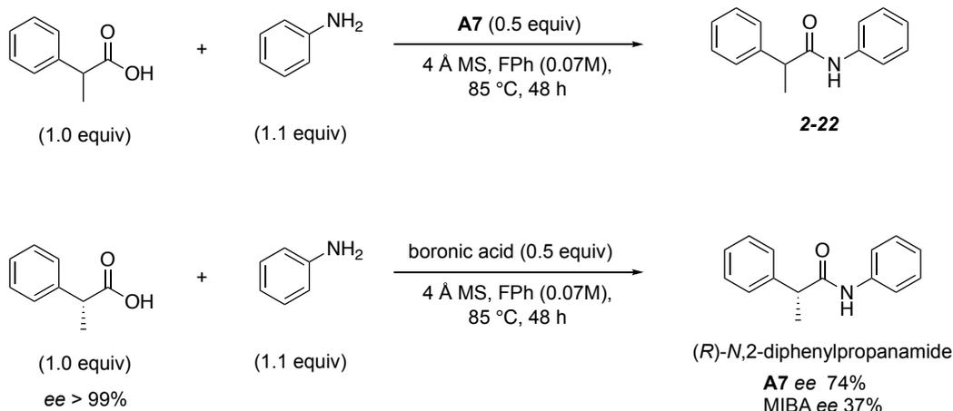
Scheme 2-8: Determination of enantiomeric excesses for the amidation reaction with a chiral acid obtained with chiral HPLC.
