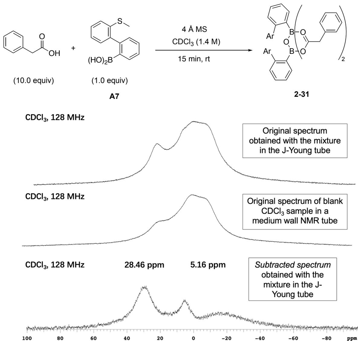
Scheme 2-11:  $^{11}\text{B}$  NMR experiment with phenylacetic acid and boronic acid **A7**.
