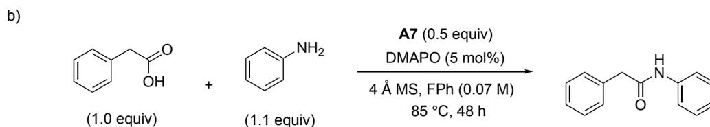
Scheme 2-5: a) Comparison of our optimized conditions and literature's conditions. b) The optimized conditions for anilide preparation.
