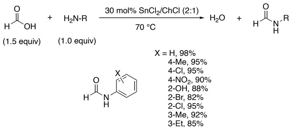
Scheme 1-10: Selected formanilide examples obtained with SnCl<sub>2</sub>/ChCl DES catalyst.
