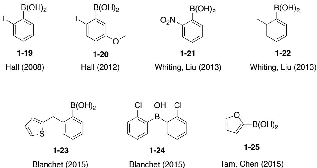
Figure 1-12: Selected organoboron catalysts for amidation reactions at temperatures below 100 °C.
