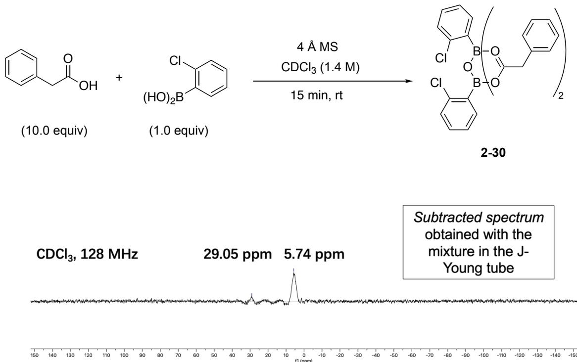
Scheme 2-10: <sup>11</sup>B NMR experiment with phenylacetic acid and 2-chlorophenylboronic acid.
