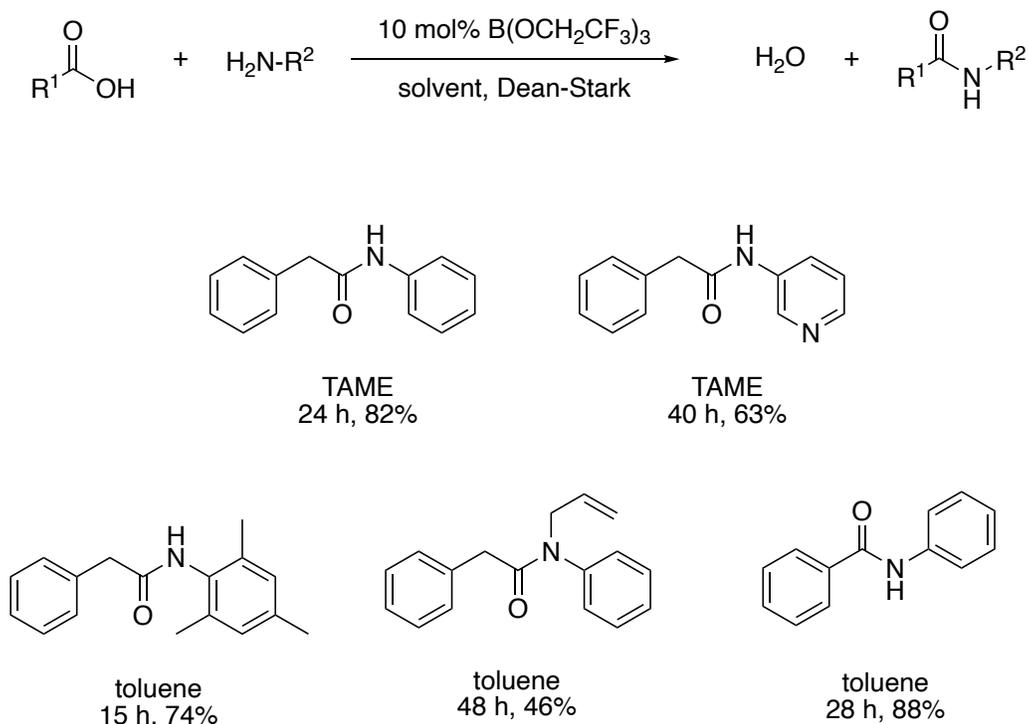
Scheme 1-16: The B(OCH<sub>2</sub>CF<sub>3</sub>)<sub>3</sub> mediated amidation reaction and selected anilide examples
