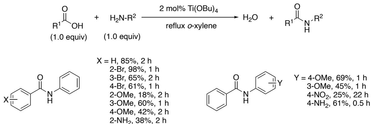
Scheme 1-8: Selected examples of amidation reactions catalyzed by Ti(OBu)<sub>4</sub>.
