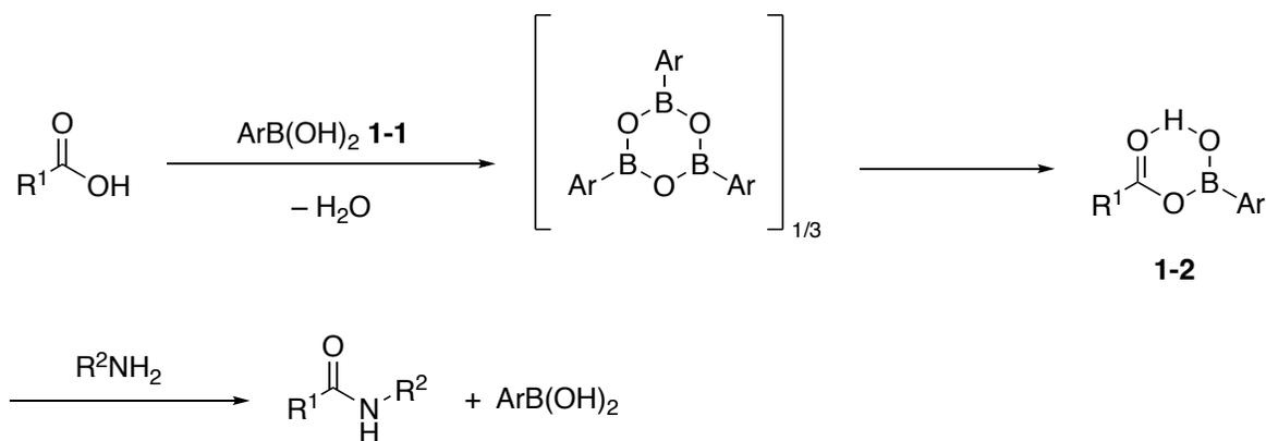
Scheme 1-12: The proposed mechanism of boronic acid **1-1** catalyzed amidation reaction.
