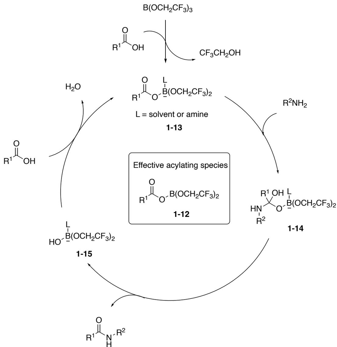
Figure 1-10: The proposed mechanism of the amidation reaction catalyzed by  $\text{B}(\text{OCH}_2\text{CF}_3)_3$ .
