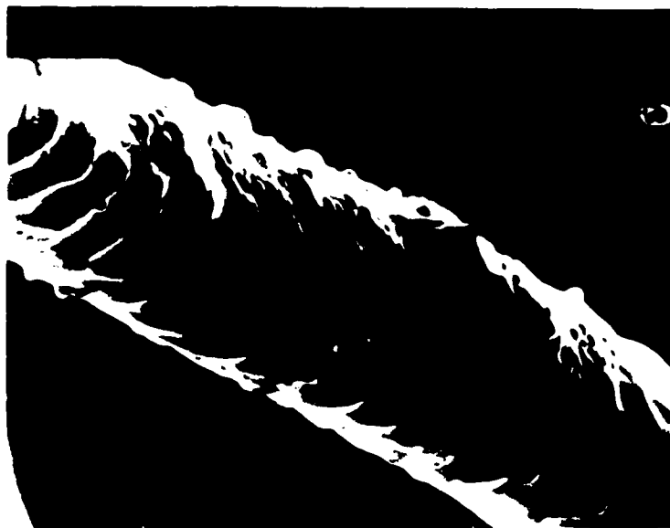
Plate 6.12.6 Bubbles and pits on surface of commercially scoured, handspun Merino wool fumigated with S.W.A.T.® for 6 days at 50°C.
