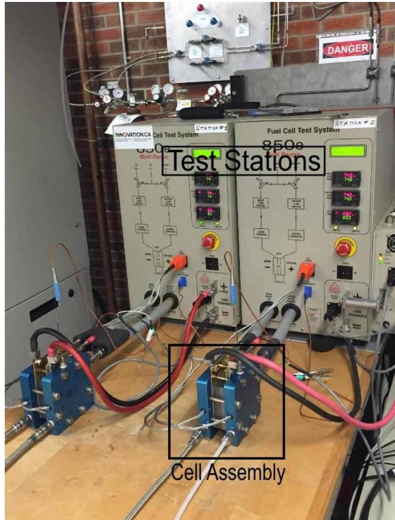
**Figure 2.10** – Fuel cell test station with the attached cell assembly
