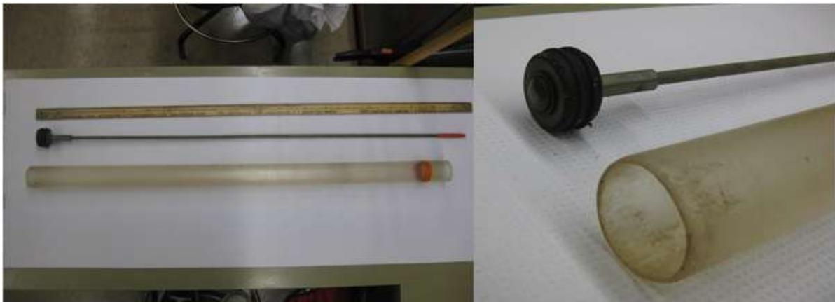
**Figure 2.5. Example of a sediment corer. This corer was constructed out of an acrylic tube 5.72 cm in diameter and a plunger made from a fitted rubber stopper attached to a threaded metal handle. The acrylic tube has sharpened edges to aid in cutting through fibrous material.**
