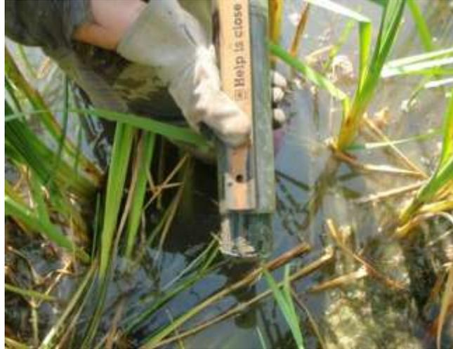
**Figure 2.7. Example of extruding excess sediment during sediment sampling.**
