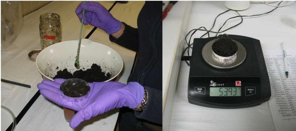
**Figure 2.8. Soil homogenization and weighing procedures carried out during sediment processing.**
