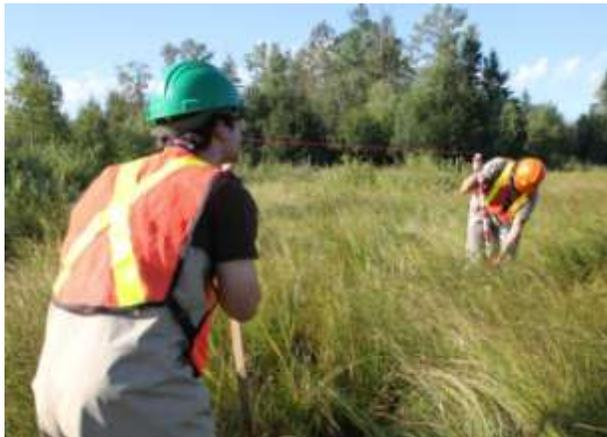
**Figure 4.4. Example of the Robel pole method, a visual obstruction technique used as a proxy measurement of biomass.**
