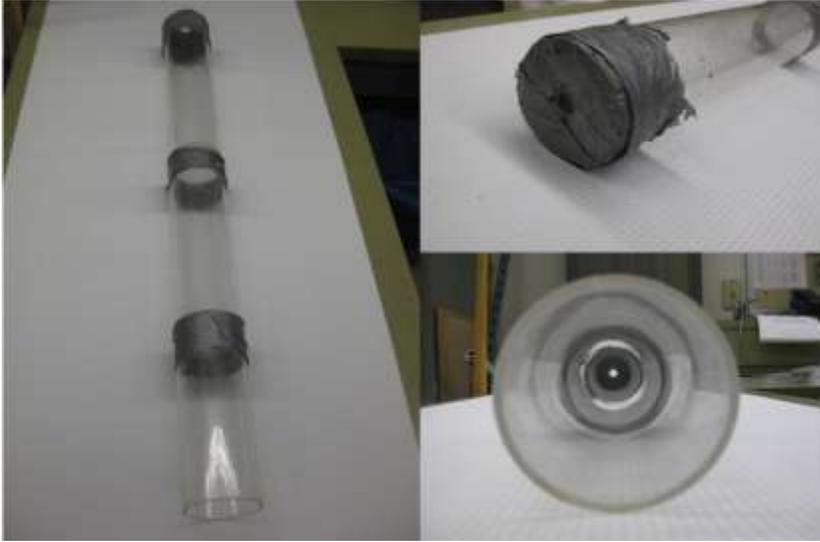
**Figure 2.4. Example of an integrated water sampling tube. A sampling tube like the one shown can be constructed out of a clear acrylic tube (left inset) that is open at one end (bottom right inset) and has a small hole drilled into the centre of other end (see top right inset).**
