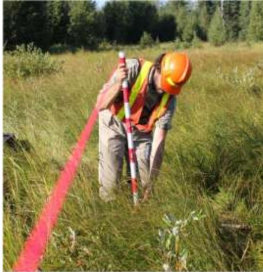
**Figure 4.5. Example of reading Robel height.**
