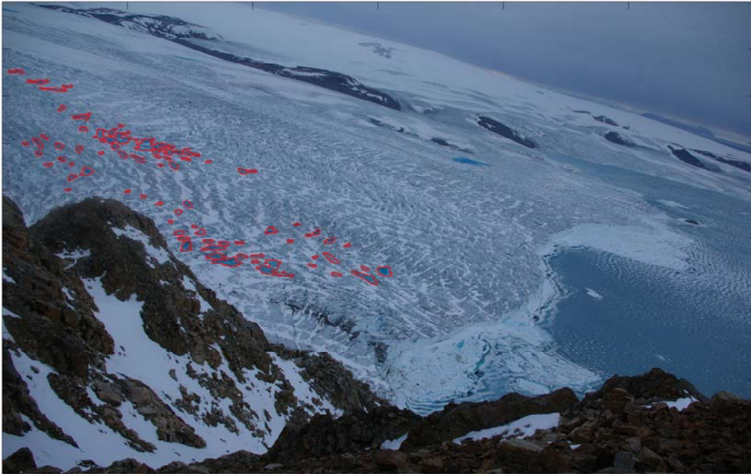
Figure 2-2: Single image acquired by TLCam4 on June 30, 2009 showing the results of our automated image classification technique. In this case our technique has successfully picked out water-filled crevasses (outlined in red).
