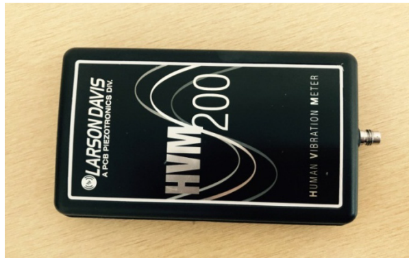
Figure 5.2: HVM 200 Data logger recorded which was well within the required range for operator health and safety, identified as 0.5 to 80 Hz range. (ISO 2631-1, 1997)
