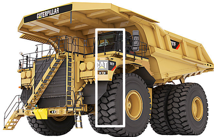
Figure 3.4: LF strut positioning relative to operator's seat
