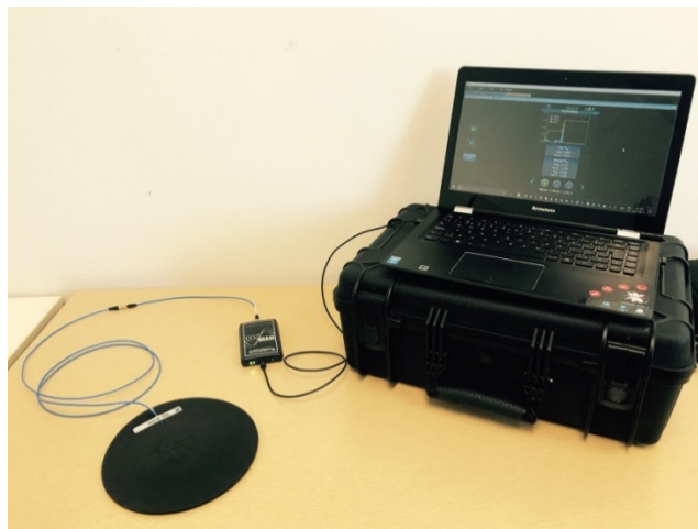
Figure 5.3: WBV Measurement Kit Setup
