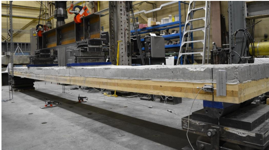
Figure 8.85: Typical bending test setup of a 6 m long CLT specimen
