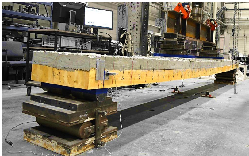
Figure 6.5: Typical bending test setup of a specimen
