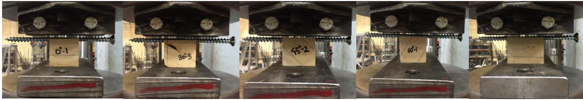
Figure 8.77: Embedment test of the screw in timber at 0^\circ , 30^\circ , 45^\circ , 60^\circ and 90^\circ angle respectively to the grain
