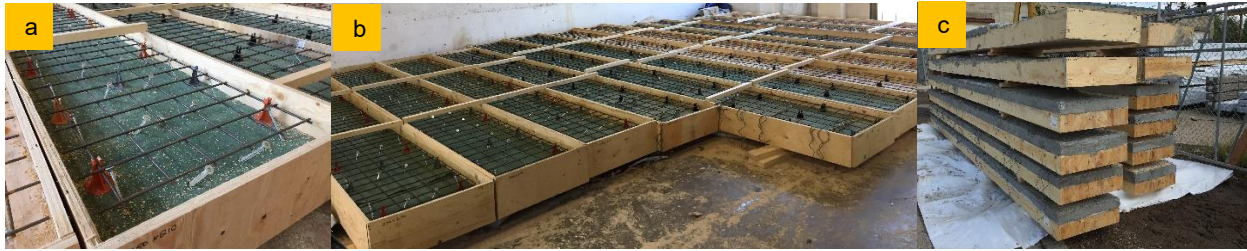
Figure 8.83: Bending test specimen preparation; a) insertion of cross-pair screw in the cross-section with wire mesh, b) specimens are ready for casting and, c) specimens are ready for testing
