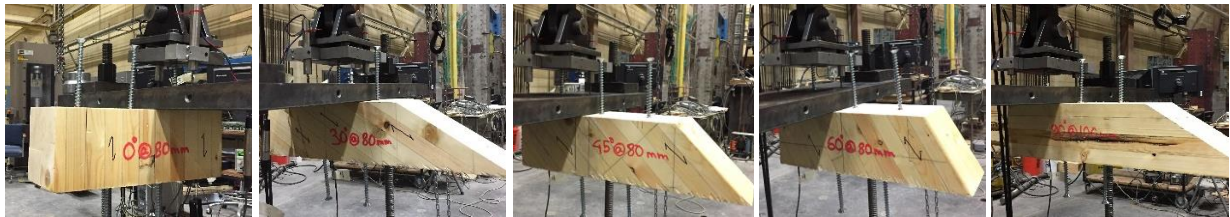
Figure 8.78: Withdrawal test of screws at 0^\circ , 30^\circ , 45^\circ , 60^\circ , and 90^\circ angle respectively to the timber grain
