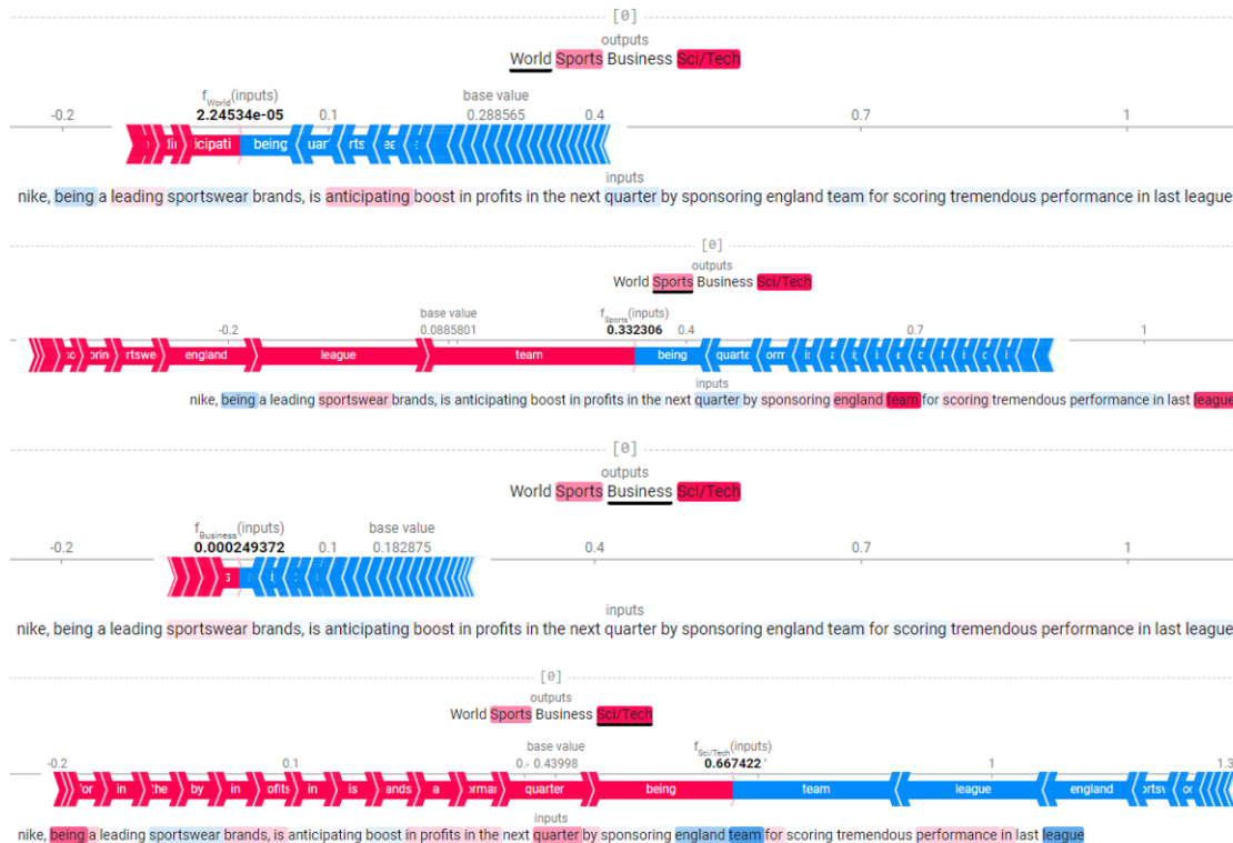
Figure 5.24: The explanation provided by SHAP for an instance of the news classification dataset. The red color in the figure represents features that have contributed positively to the prediction. Features in blue have contributed negatively to the prediction.
