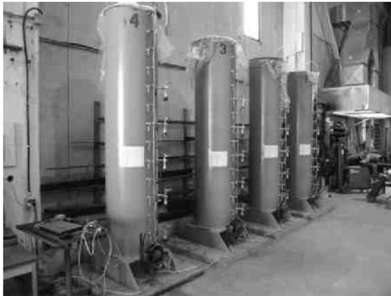
**Figure 2. Indoor Consolidation Columns**
