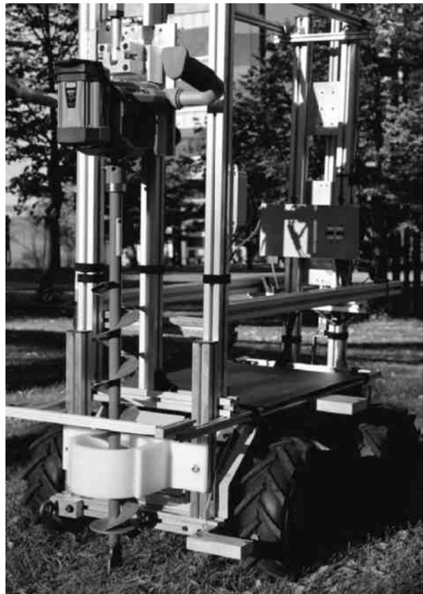
**Figure 6. Earth auger and brushless DC motor mounted on linear actuator.**
