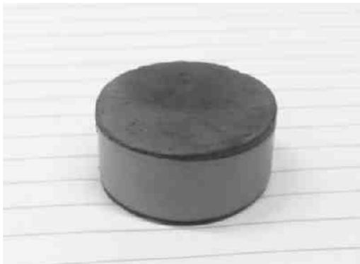
Figure 5. FMFT sample in the confinement of the electrical tape
