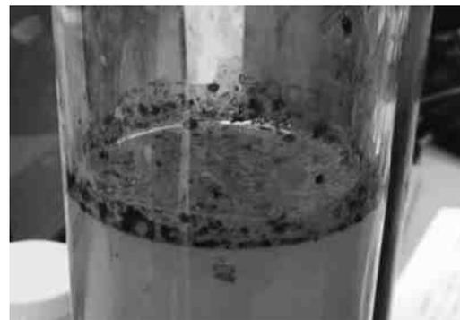
Figure 6. Oil residue at the top of the experimental column
