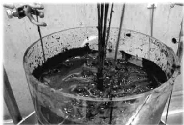
**Figure 4. Settled TSRU Tailings Loaded in Smoldering Vessel**
