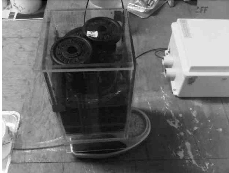
**Figure 2. View of the calibration test cell with applied surface load.**
