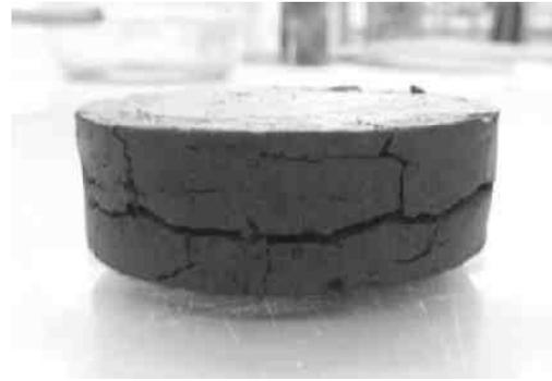
**Figure 8. FMFT specimen at the end of free swelling test**
