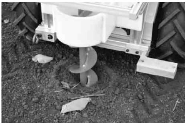
**Figure 9. Drilling mechanism on loose soil.**
