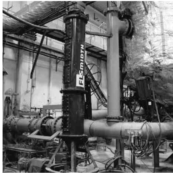
Figure 1. 0.6 m ID FLS Deep Cone Thickener
