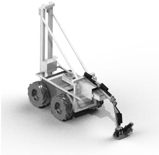
**Figure 4. CAD As-Built of Robotic Manipulator Mounted on Mobile Platform**
