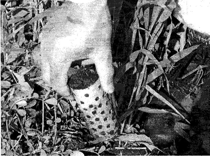
b) Acetylene being inserted into jar with soil core
