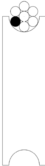
(b) Diagram of Costello's strand cross section on sheave showing the critical wire
