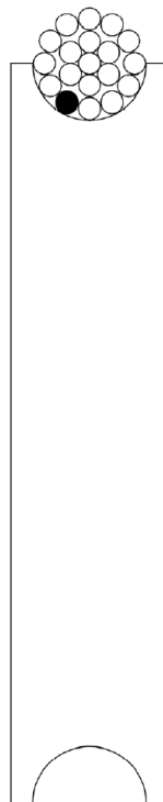
(b) Diagram of Knapp's strand cross section on sheave showing the critical wire
