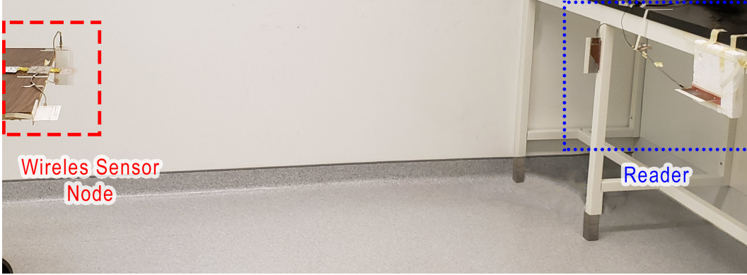
Figure 7.13: Test setup for the proposed non-hybrid six-port RFID-based battery-less wireless with pin diode attached at the sensing element port.
