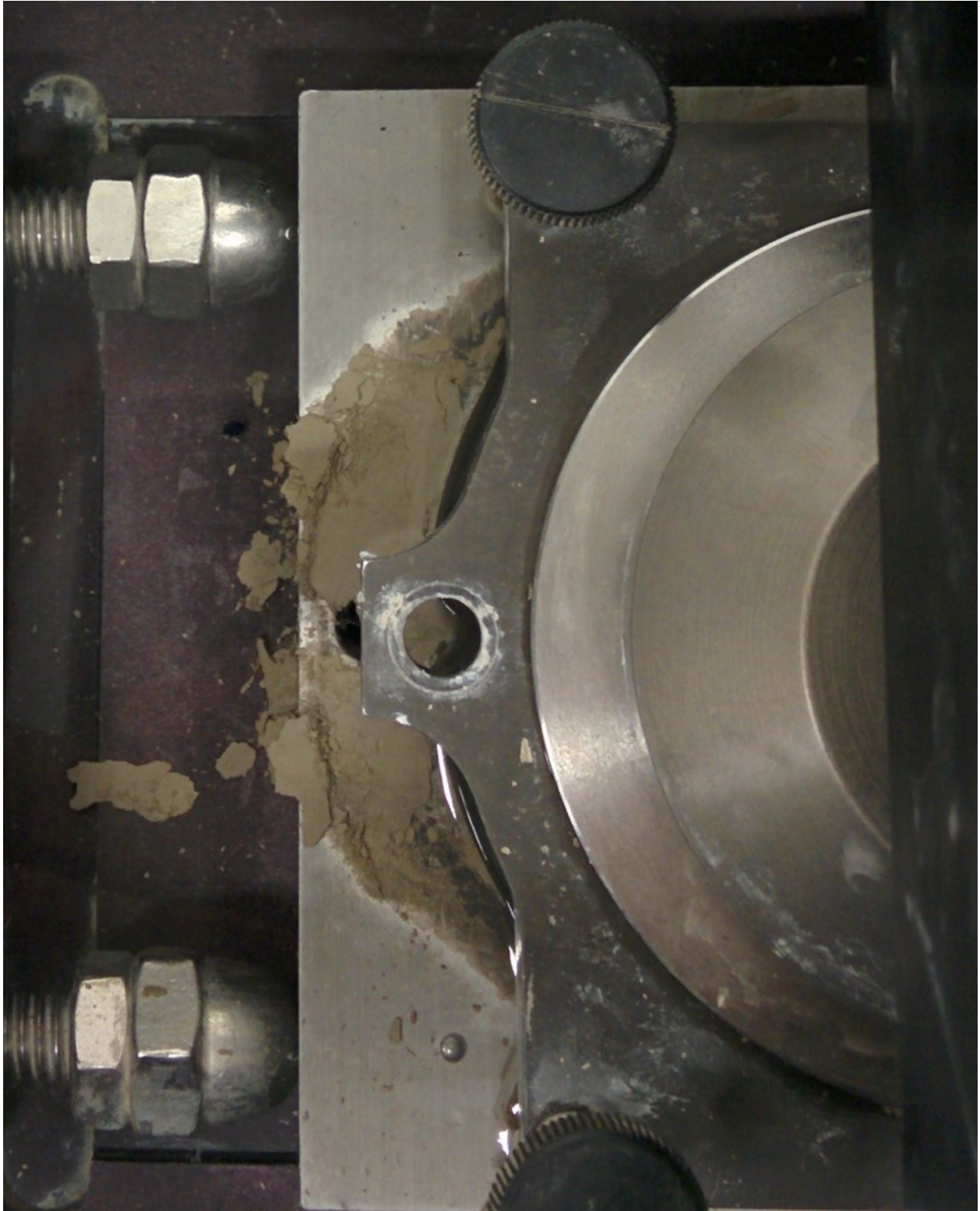
Figure F.1. Soil extrusion at gap between shear box halves in Test S42_2
