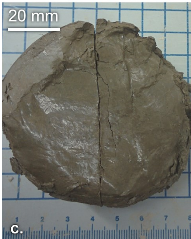
Figure B.2 Slickensides: (a) BH15-03 depth 9.5 m; (b) BH15-01 depth 10.1 m; (c) BH15-01 depth 12.0 m; (d) BH15-01 depth 7.7 m
